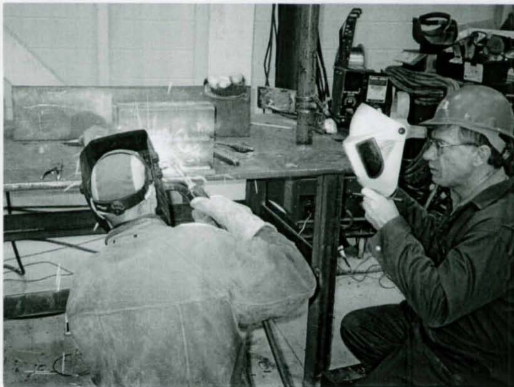
Figure 22. Horizontal Welding of Test Specimen at Walters Inc.
