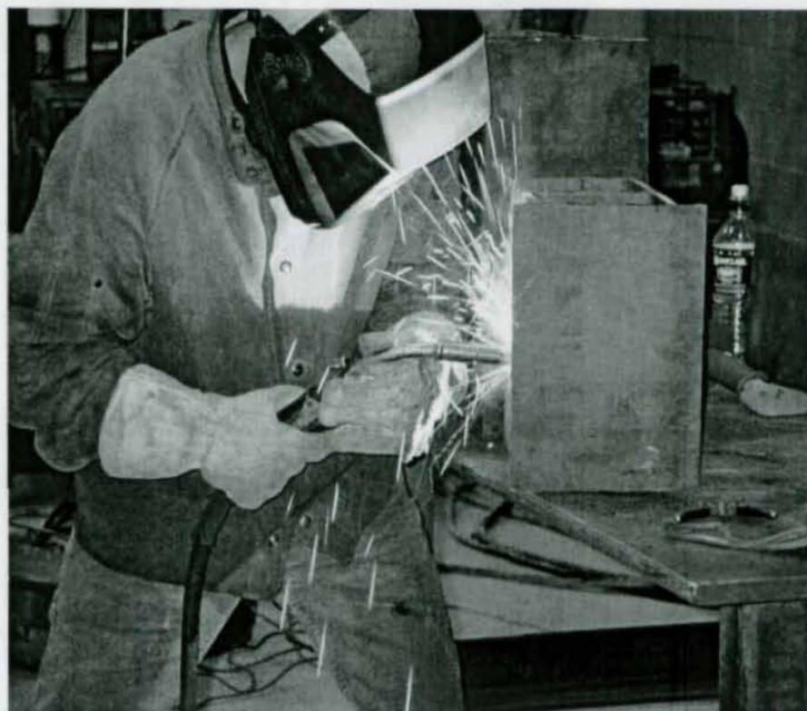
Figure 23. Vertical Welding of Test Specimen at Walters Inc.
