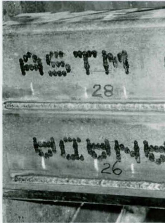
Figure 24. External Appearance of Two FCAW-G Test Welds, No. 26 and No. 28
