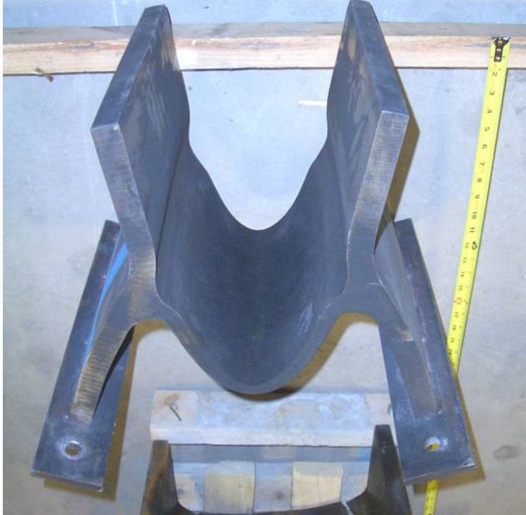
(a) Ductile section response.
