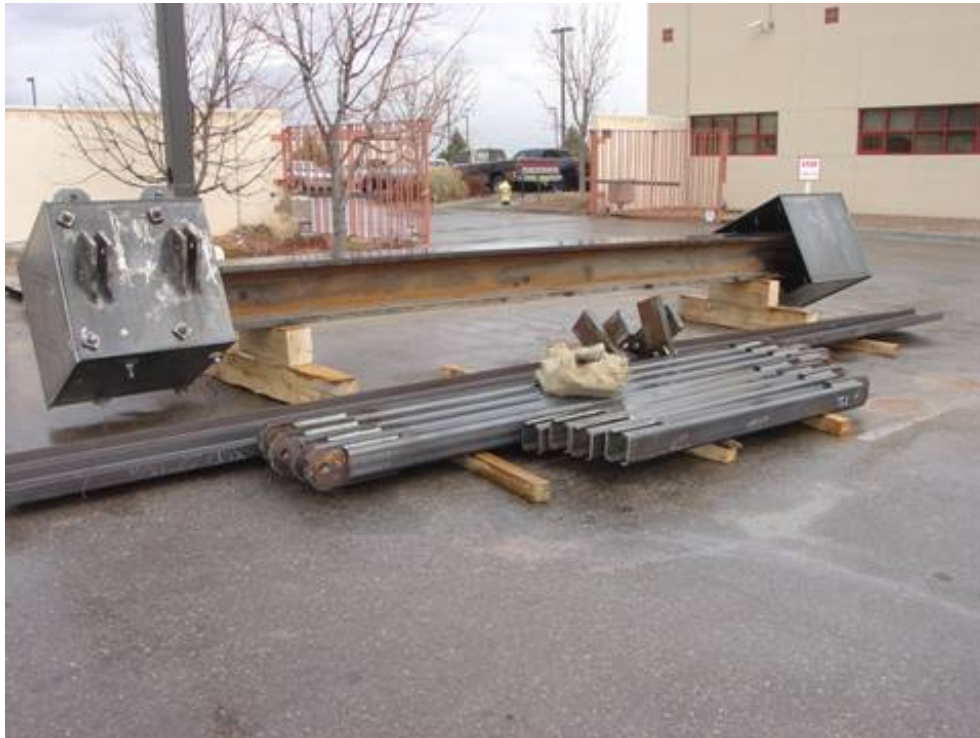
(b) Fabricated column specimen prior to installation.
