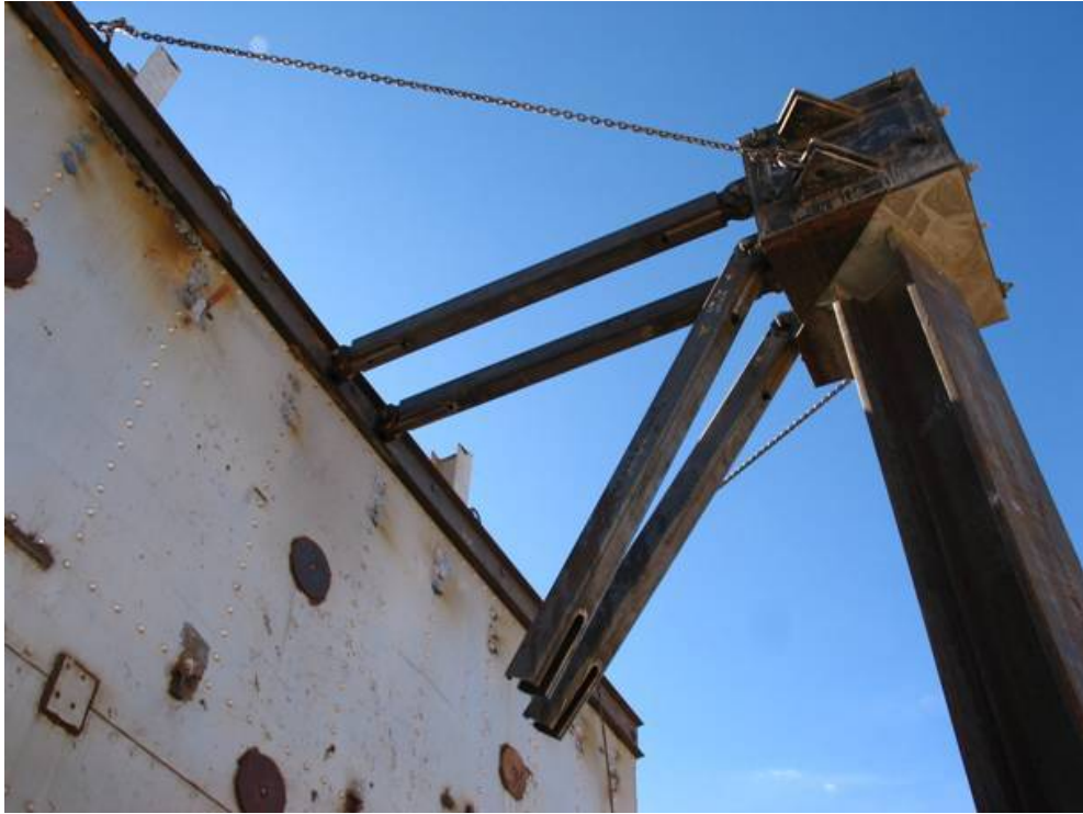
(a) Attachment of the rear reaction struts.
