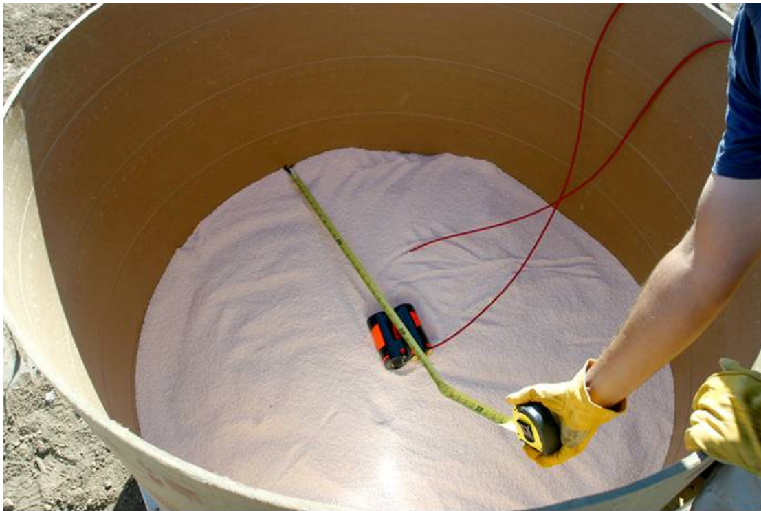
(a) ANFO is filled halfway and the booster placed.
