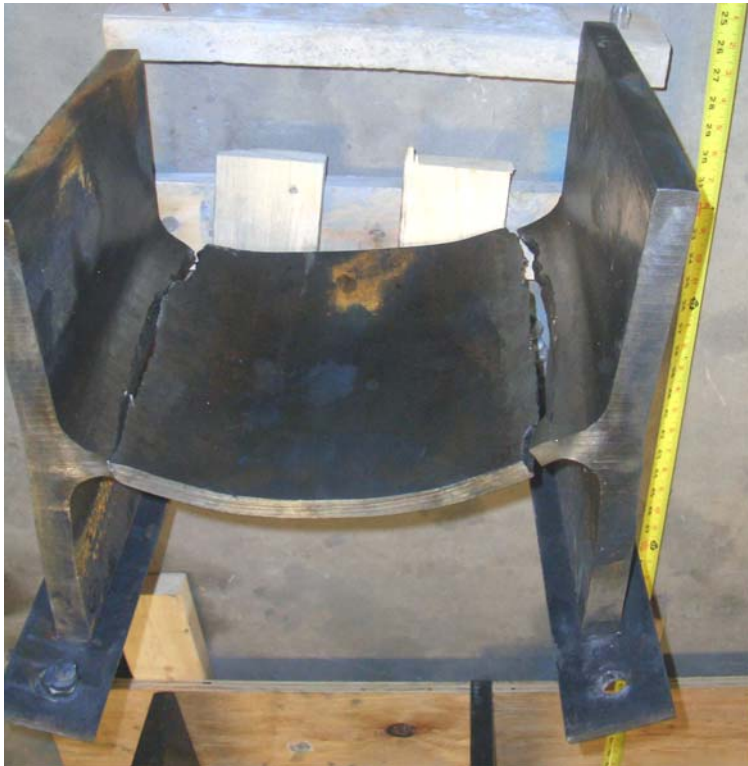
(b) Ductile fracture in K-line.
