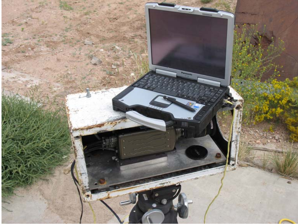
(a) Typical Phantom ® high-speed digital camera w/ laptop computer shown installed in a protective steel box.
