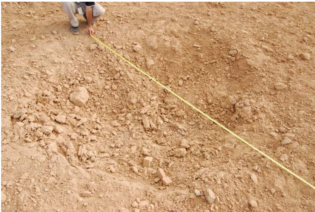
(a) View of detonation crater diameter.
