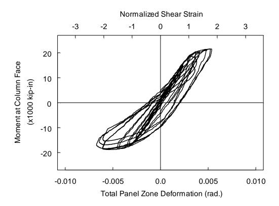
Figure 3.12 Specimen C1 Moment versus Total Panel Zone Shear Deformation Relationship
