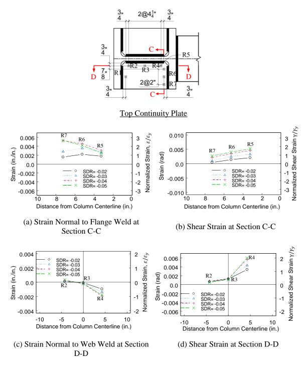
Figure 3.36 Specimen C2 Top Continuity Plate Strain Profiles
