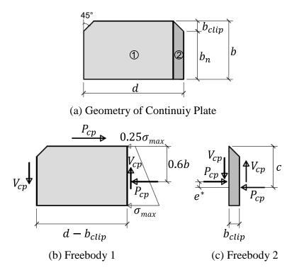
Figure 1.3 Continuity Plate Freebody Diagrams (Exterior Connection)
