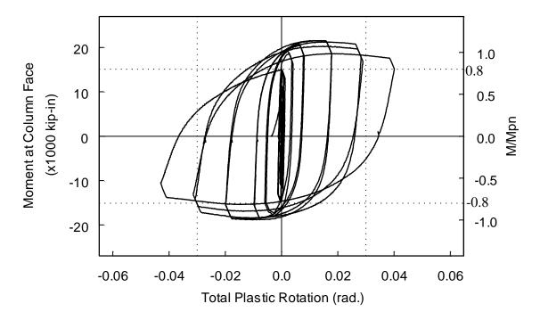
Figure 3.11 Specimen C1 Moment versus Total Plastic Rotation Relationship
