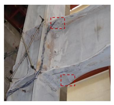
Figure 3.21 Specimen C2 Beam Flange Yielding at Completion of 0.01 rad Drift Cycles
