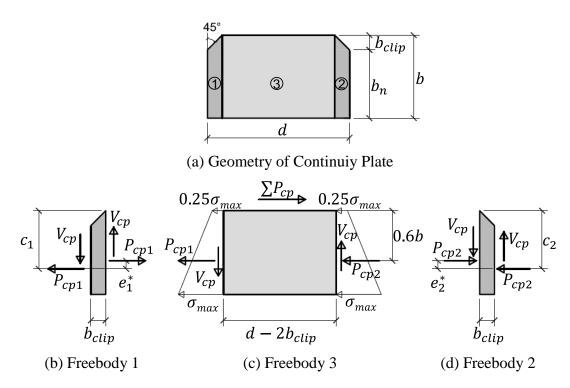
Figure 1.2 Continuity Plate Freebody Diagrams (Interior Connection)
