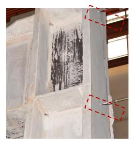
(b) Column Flange Yielding Due to Column Kinking (Back Side)
