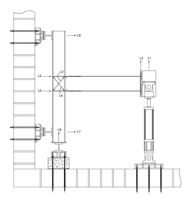
Figure 2.7 Location of Displacement Transducers
