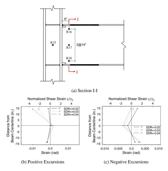
Figure 3.39 Specimen C2 Beam Web Shear Strain Profiles
