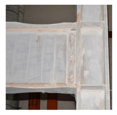
Figure 3.20 Specimen C2 Panel Zone Minor Yielding at Completion of 0.0075 rad Drift Cycles
