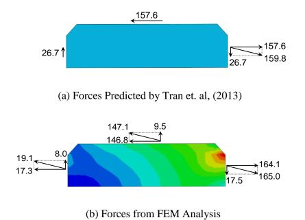
Figure 4.8 Specimen C1 Comparison of Forces Acting on Continuity Plate
