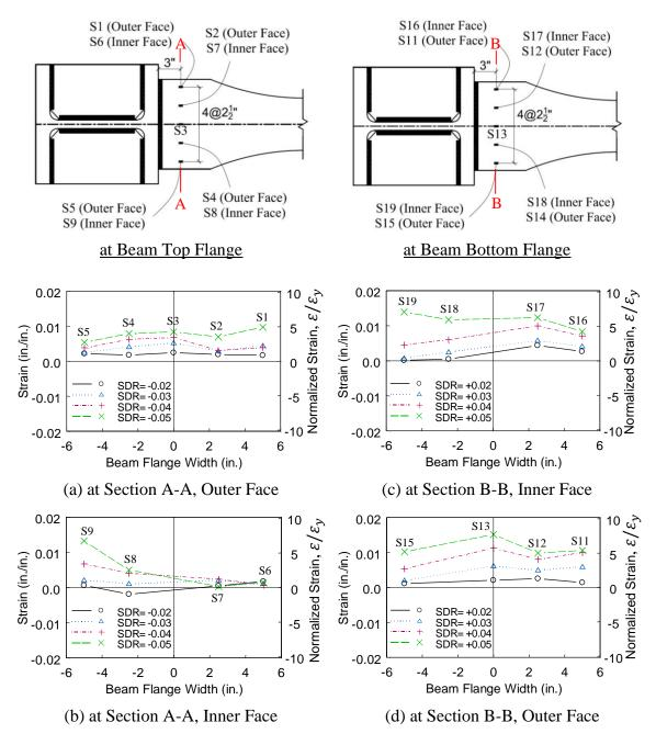
Figure 3.35 Specimen C2 Beam Flange Flexural Strain Profiles
