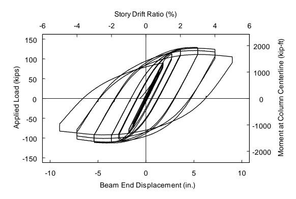
Figure 3.9 Specimen C1 Load versus Beam Tip Displacement Relationship
