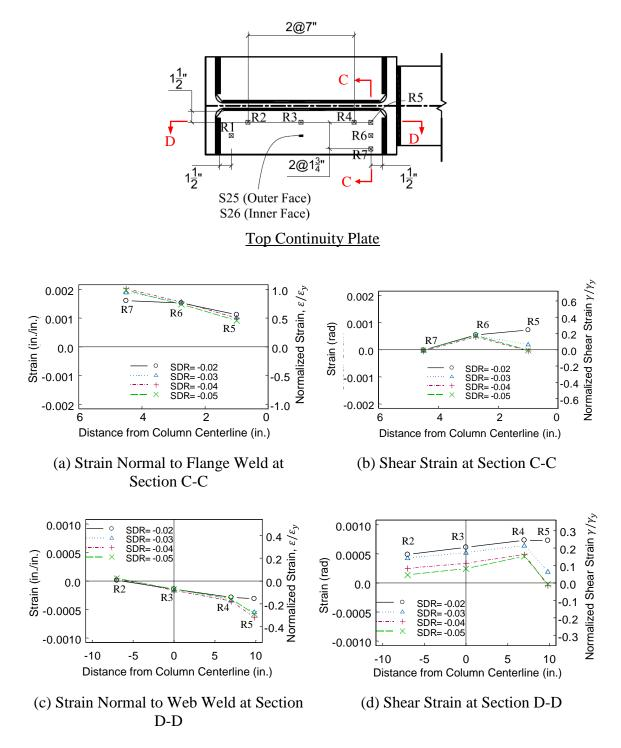
Figure 3.14 Specimen C1 Top Continuity Plate Strain Profiles
