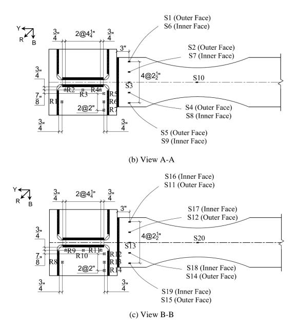
Figure 2.9 Specimen C2 Strain Gage and Rosette Locations (continued)
