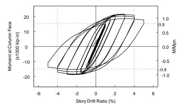
Figure 3.10 Specimen C1 Moment versus Story Drift Angle Relationship
