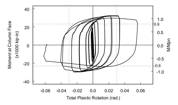
Figure 3.33 Specimen C2 Moment versus Total Plastic Rotation Relationship
