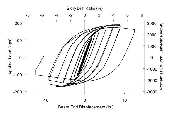
Figure 3.31 Specimen C2 Load versus Beam Tip Displacement Relationship
