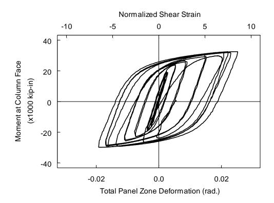
Figure 3.34 Specimen C2 Moment versus Total Panel Zone Shear Deformation Relationship
