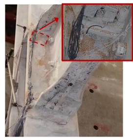
(c) Column Flange Yielding Due to Column Kinking (Front Side)
