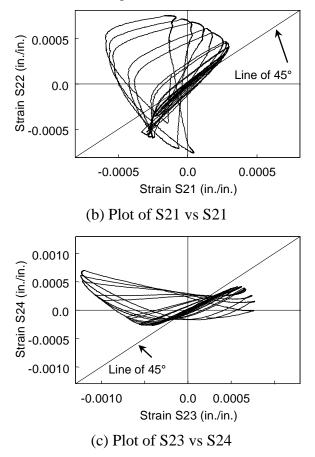
Figure 3.17 Specimen C1: Effect of Column Twisting on Column Flexural Strains
