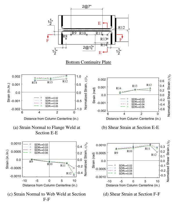
Figure 3.15 Specimen C1 Bottom Continuity Plate Strain Profiles
