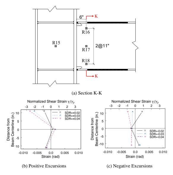
Figure 3.18 Specimen C1 Beam Web Shear Strain Profiles
