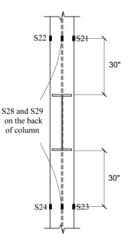
(a) Location of Strain Gages on the South Face of the Column
