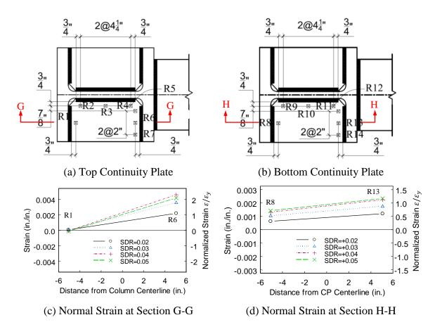
Figure 3.38 Specimen C2 Top and Bottom Continuity Plates Strain Profiles
