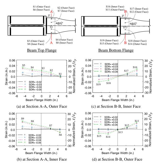
Figure 3.13 Specimen C1 Beam Flange Flexural Strain Profiles
