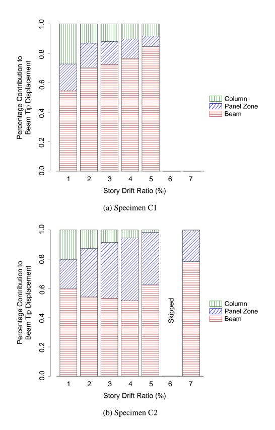
Figure 4.3 Components of Beam End Displacement
