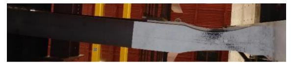
(e) Beam Lateral-Torsional Buckling
