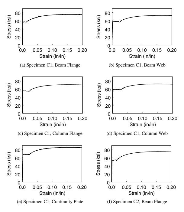
Figure A.1 Tensile Coupon Stress-Strain Relationships
