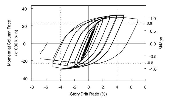
Figure 3.32 Specimen C2 Moment versus Story Drift Angle Relationship
