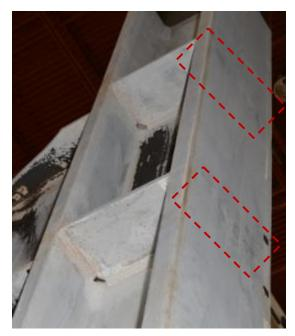
(b) Column Flange Yielding Due to Column Kinking (Back Side)
