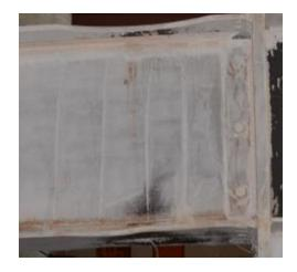
(e) Detail C, Minor Flange and Web Local Buckling
