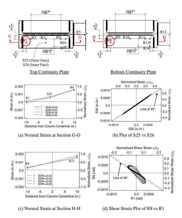
Figure 3.16 Specimen C1 Top and Bottom Continuity Plates Strain Profiles
