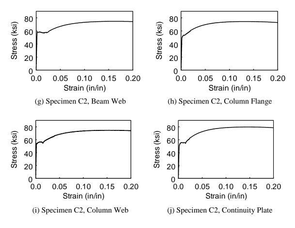
Figure A.1 Tensile Coupon Stress-Strain Relationships (continued)
