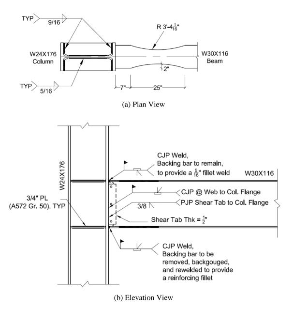
Figure 2.1 Specimen C1 Connection Detail
