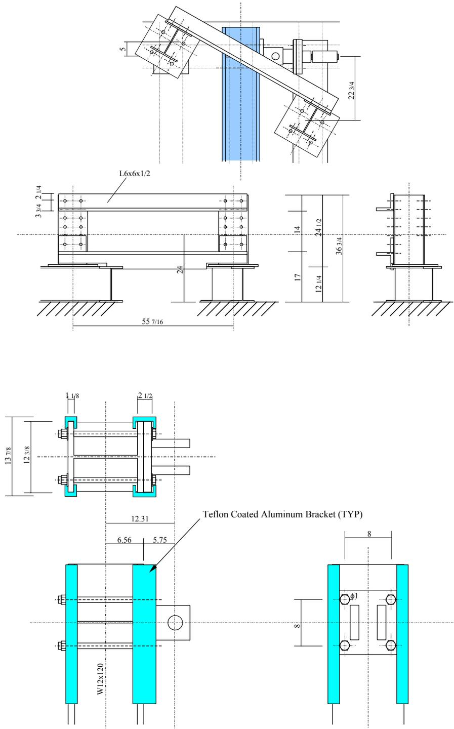
Fig. 17 – Lateral Support System: Details at Top of Column
