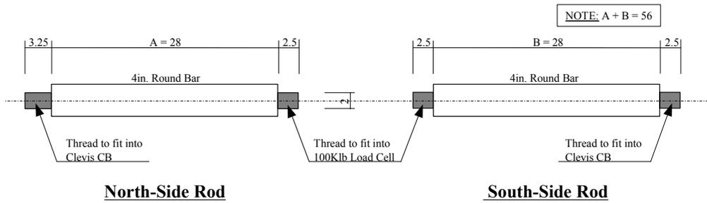
Column Lateral Reaction Rods (2 Complete Assemblies Req'd)
