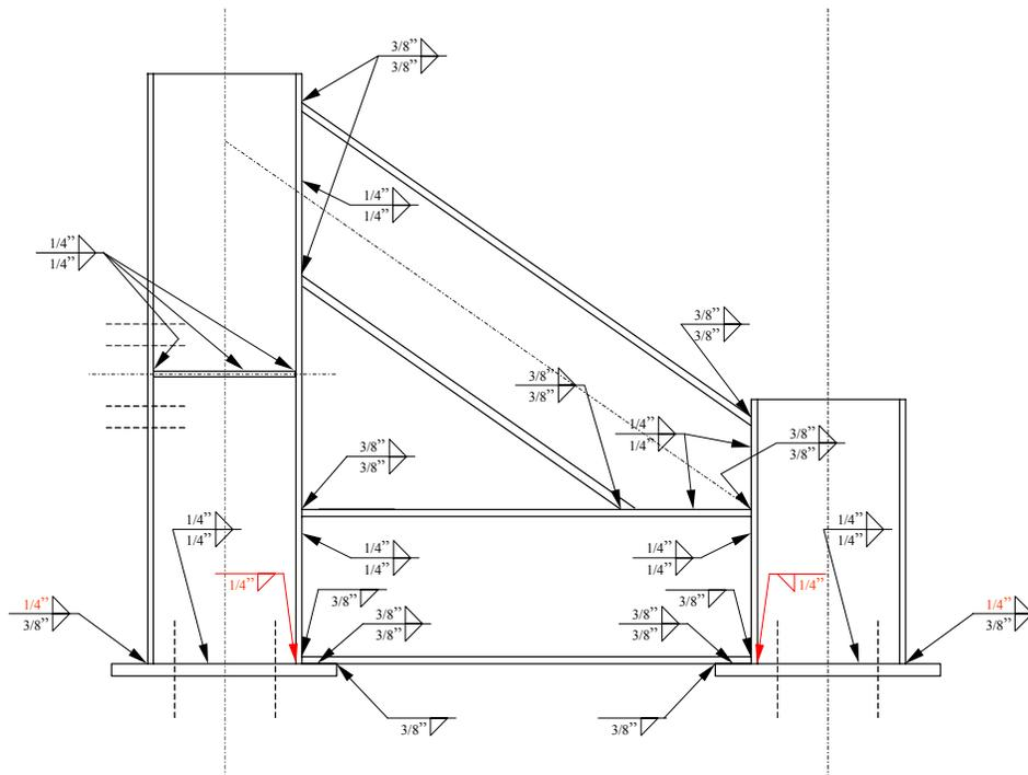
**Reaction Frame for Column Lateral Reactions – Add'l Details**
