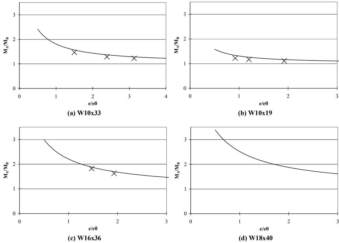
Fig. 10 – Link End Moment Ratios for Test Specimen Sections
