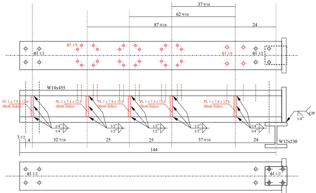
**Reaction Beam for Hydraulic Ram Base and Link End Reaction**
