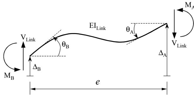
Fig. 9 – Isolated Link for Analysis of End Moment Ratio
