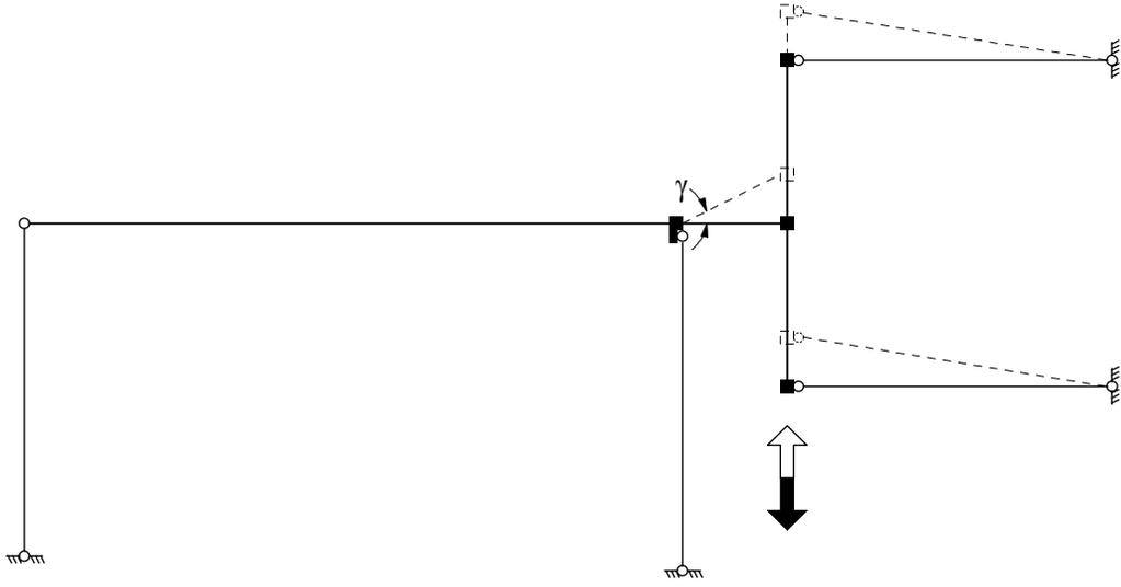
Fig. 2 - Rigid – Plastic Kinematics of Test Setup
