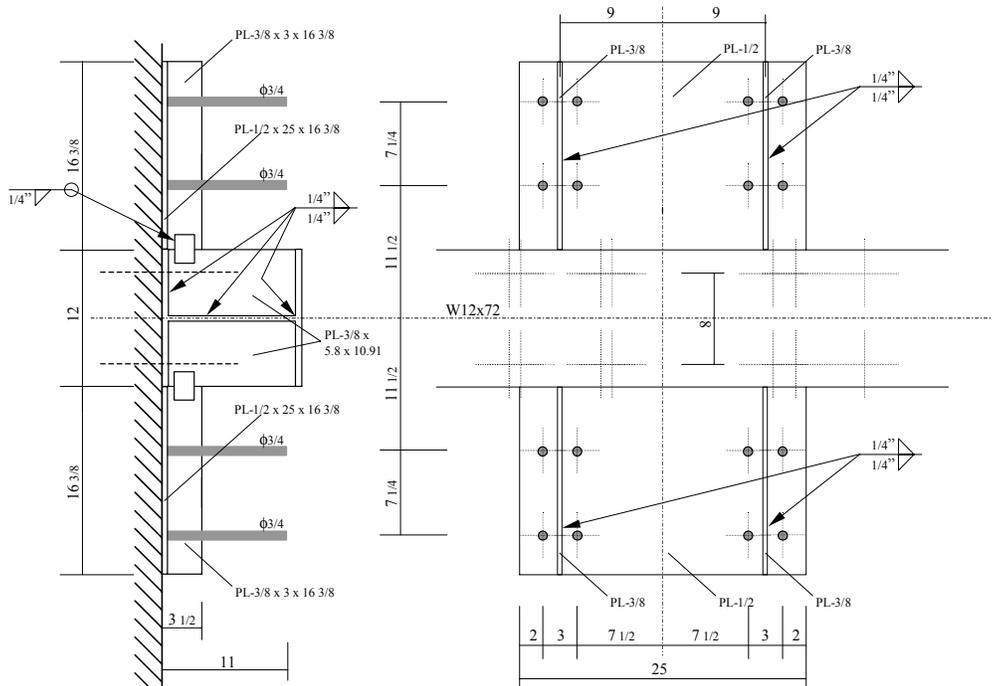
***Fixture for Attachment of Link End Lateral Support to***
