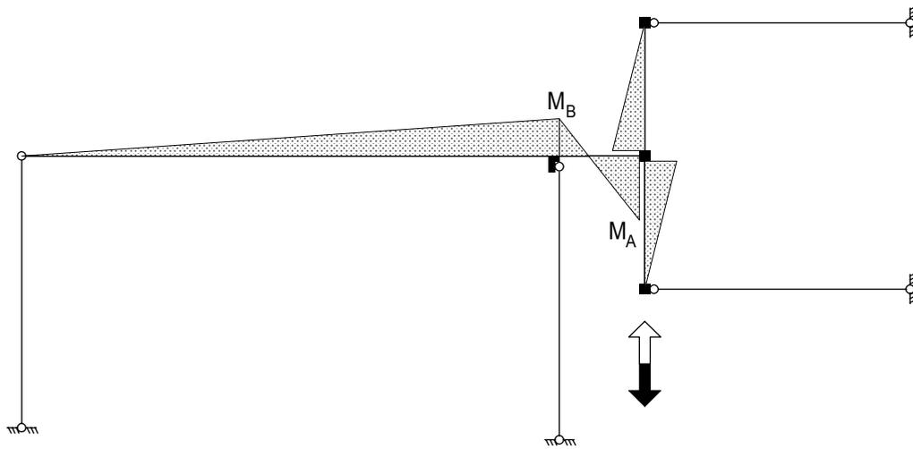
Fig. 3 – Moment Diagram for Test Setup
