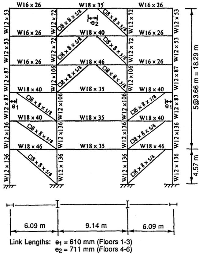
Fig.5 – Prototype Six Story EBF Used for Evaluation of Link End Moment Ratio (Ricles and Popov 1994)
