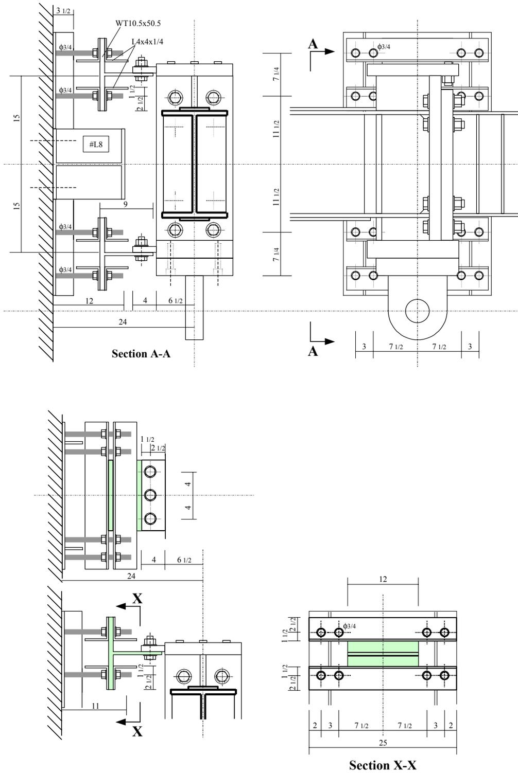
Fig. 19 – Lateral Support System: Details at Link End
