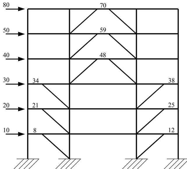
Fig. 6 – Loading and Link Identifiers for Prototype EBF
