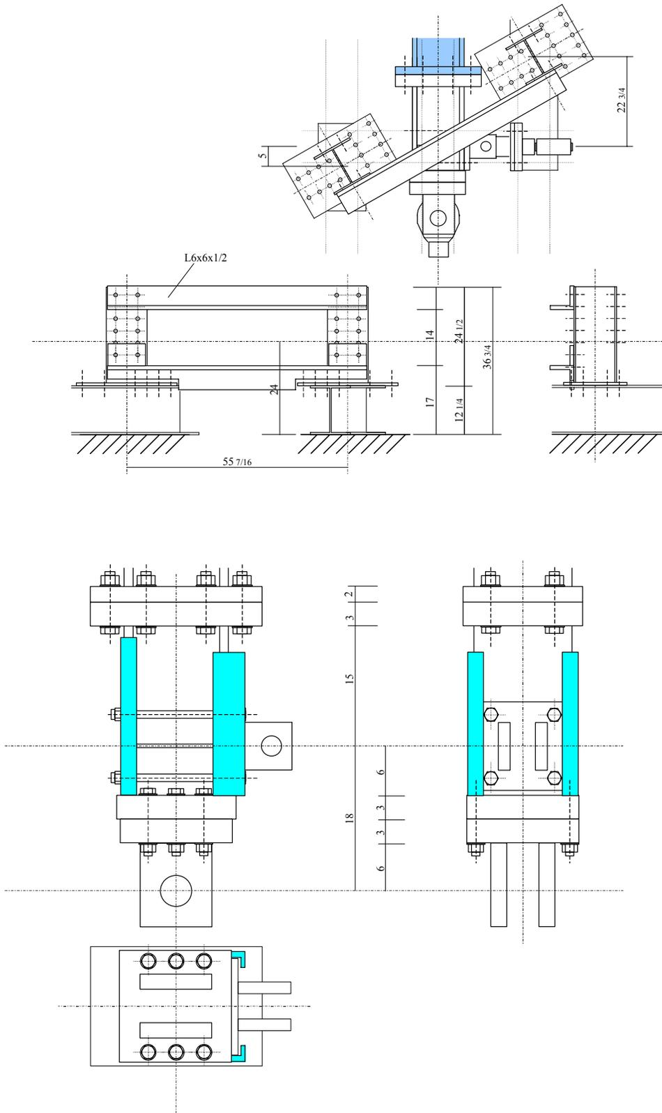
Fig. 18 – Lateral Support System: Details at Base of Column
