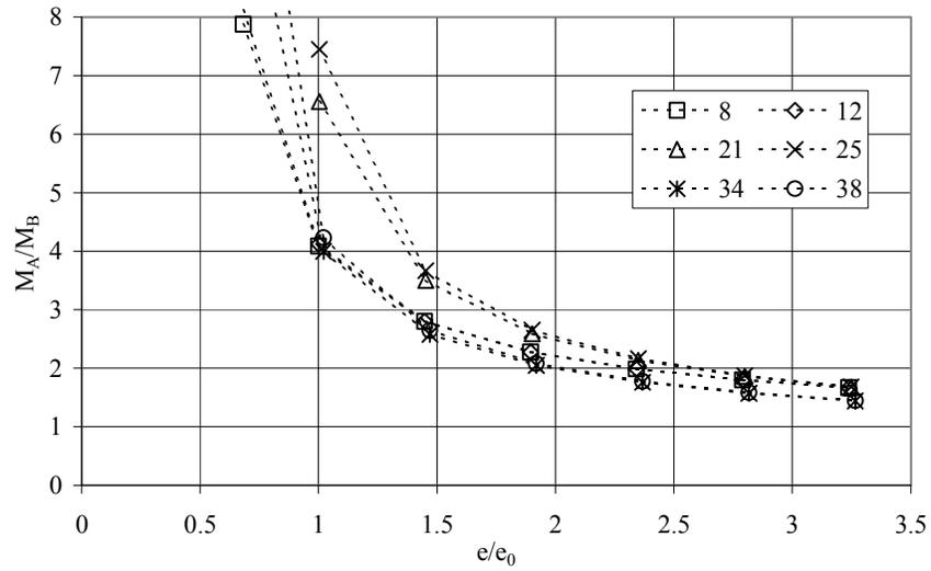
Fig. 7 – Link End Moment Ratios for Prototype EBF: Dual System
