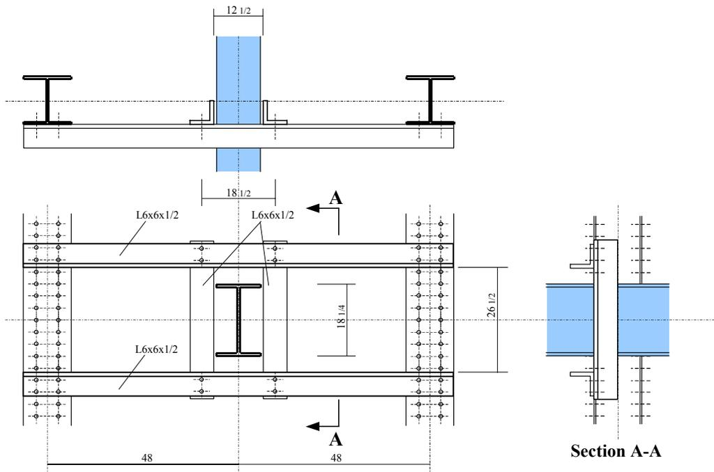
Fig. 20 – Lateral Support System: Details at Beam End
