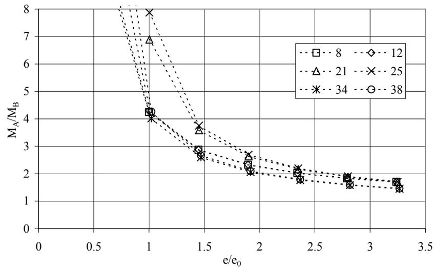
Fig. 8 – Link End Moment Ratios for Prototype EBF: Non-Dual System
