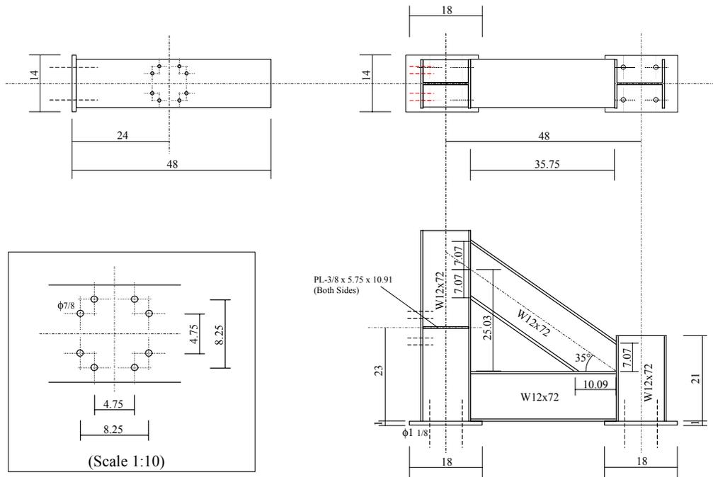
**Reaction Frame for Column Lateral Reactions (2 Req'd)**
