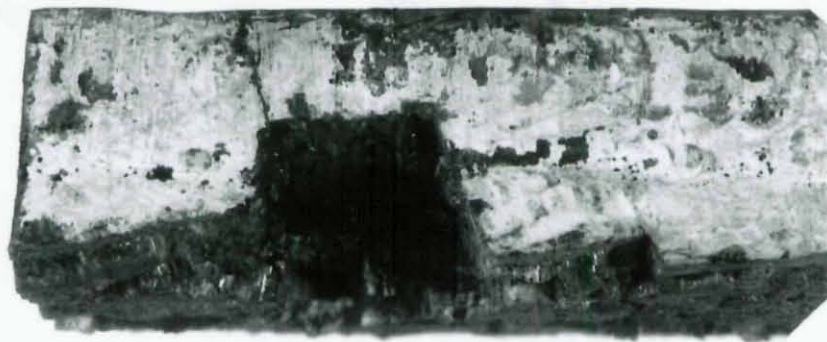
Figure 23. North piece from the beam-side fracture of the east-beam top-flange joint.
