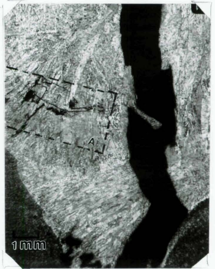
Figure 13. Macro sections from the west-beam bottom-flange joint.
