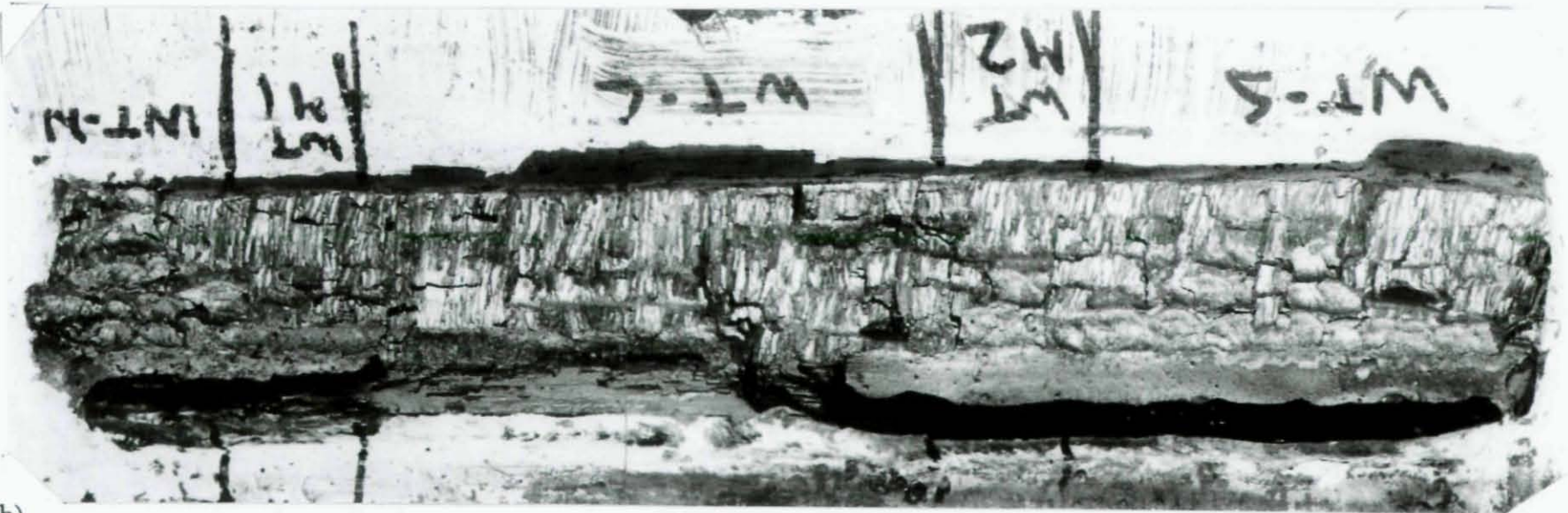
Figure 31. As received fracture pieces from the west-beam top-flange joint.
