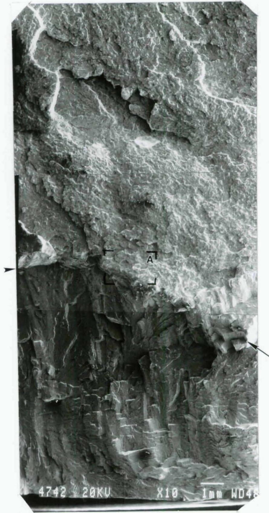
Figure 25. Boundary between weld-metal and fusion-plane fracture surfaces.
