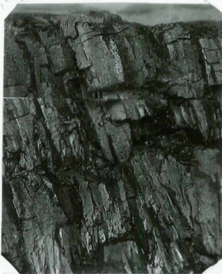
Figure 35. North piece from the fracture surface on the beam side of the west-beam top-flange surface.
