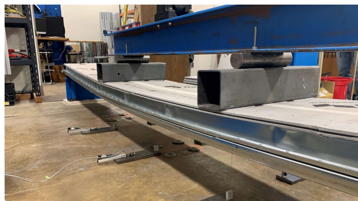
(a) photo of 4 point bending test conducted in JHU lab
