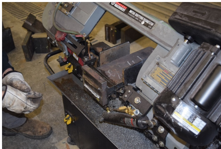
Fig. 3.10. Sectioning a specimen for etching.
