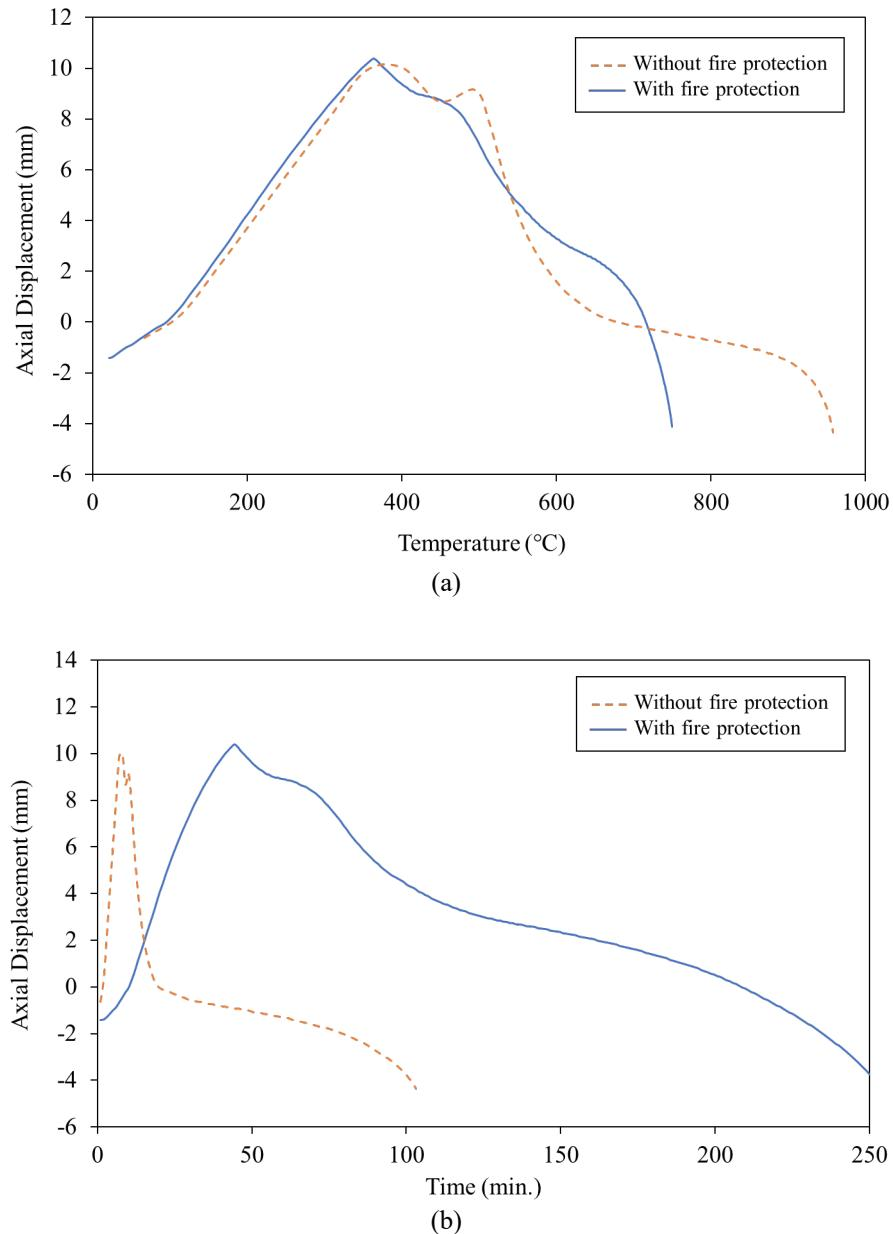
Fig. 4-23. (a) Axial displacement versus surface temperature and (b) axial displacement versus time comparisons for a column with and without fire protection
