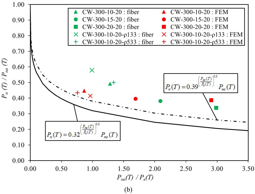
Fig. 4-26. Normalized results of the comparison between fiber-model and FE analysis for wall specimens using section method for (a) 200 mm wall thickness and (b) 300 mm wall thickness
