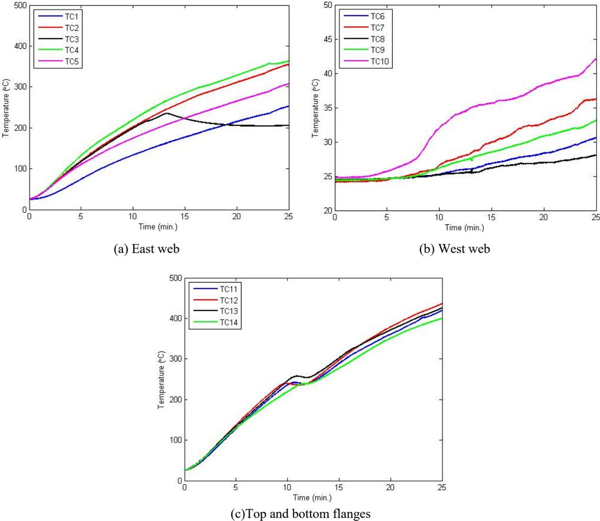
Fig. 2-21. Measured temperatures - CW2 (Test1)
