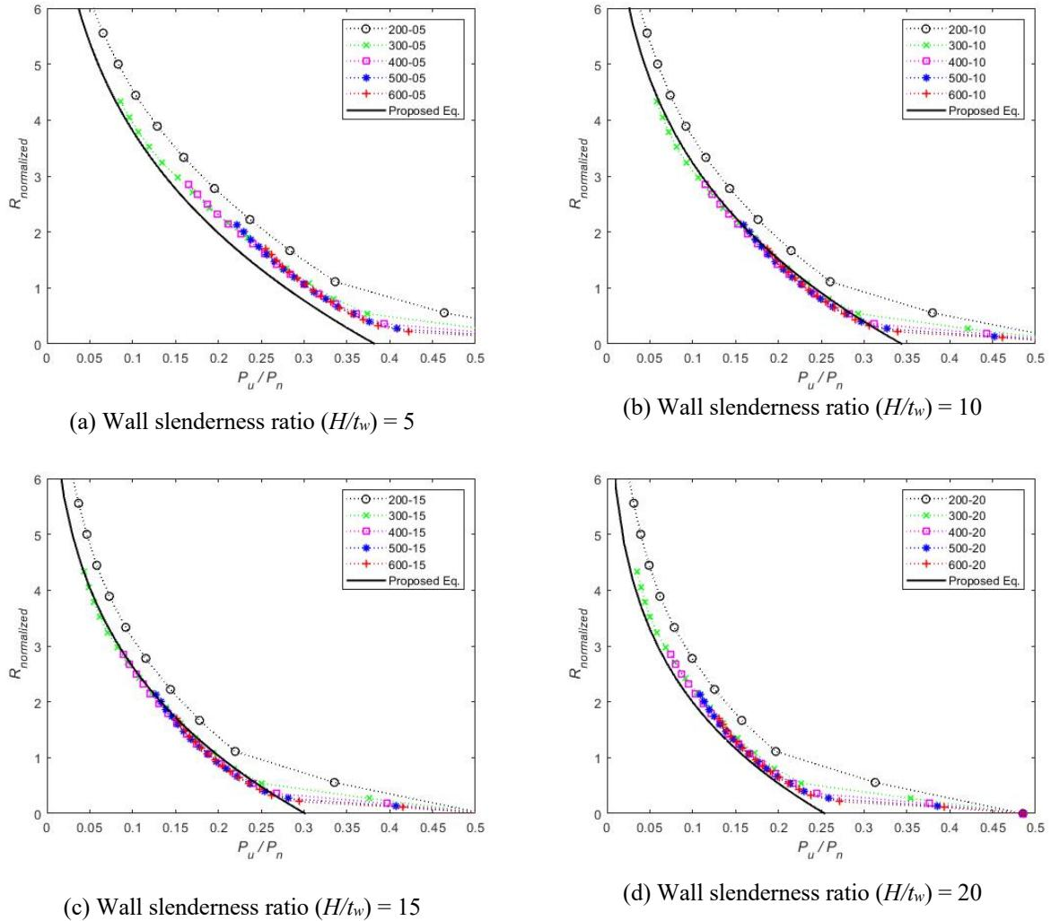
Fig. 3-23. The fitted curve for various wall slenderness ratios (Power format)
