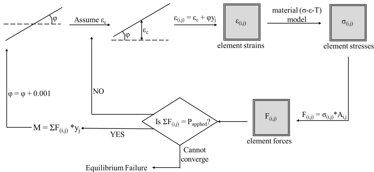
Fig. 4-4. Pictorial flowchart for calculating section moment-curvature response
