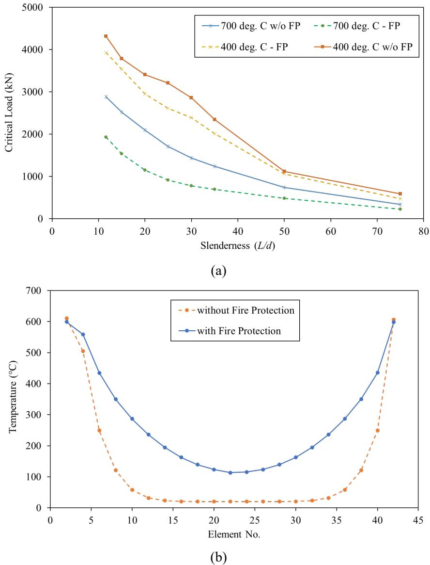
Fig. 4-22. (a) Critical load vs Slenderness comparison for a column with and without fire protection. (b) Temperature profiles for a column at failure with and without FRP for steel surface temperature = 600 °C
