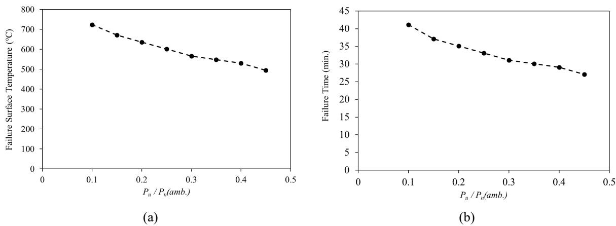
Fig. 4-37. (a) Failure surface temperature and (b) Failure time against axial load ratio for wall slenderness = 25 for single-sided heating
