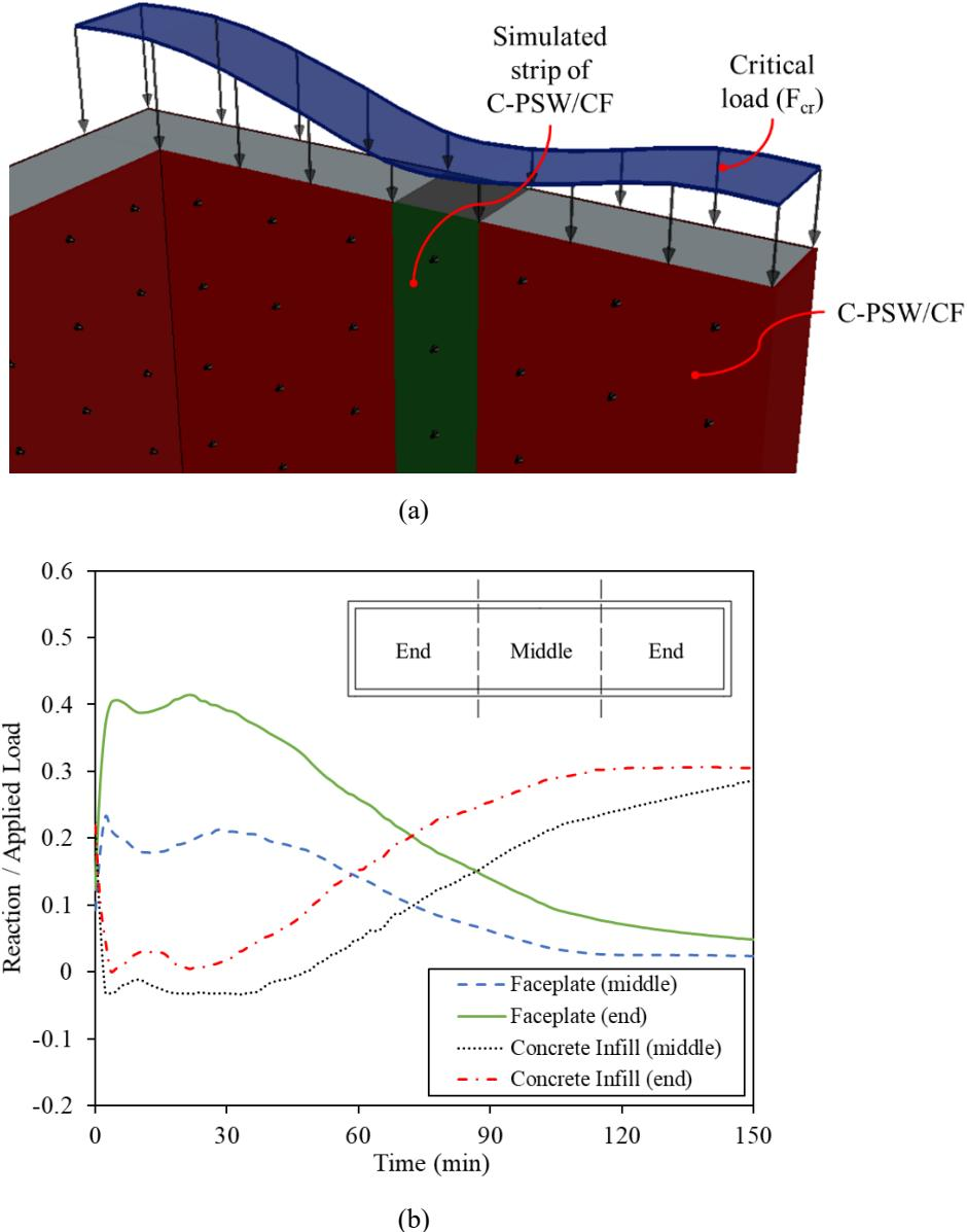
Fig. 3-15. (a)The variation of critical load of a C-PSW/CF along the width. (b) Distribution of axial load between the middle and end regions in SCW4.
