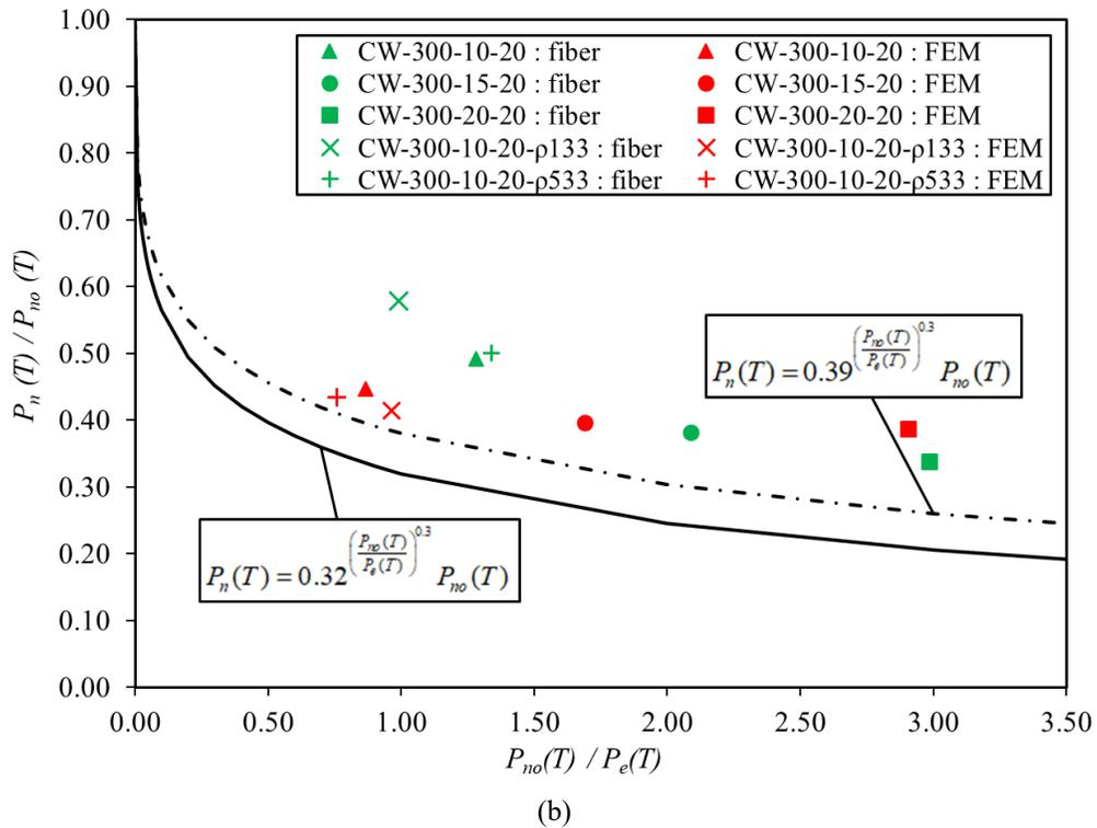
Fig. 4-26. Normalized results of the comparison between fiber-model and FE analysis for wall specimens using section method for (a) 200 mm wall thickness and (b) 300 mm wall thickness
