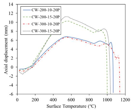
(b) Axial displacement against surface temperature
