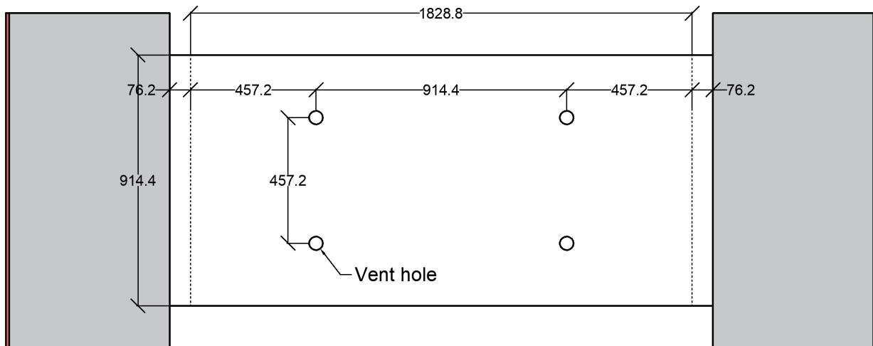
Fig. 2-30. Location of designed vent holes on CW3. All dimensions are in mm.
