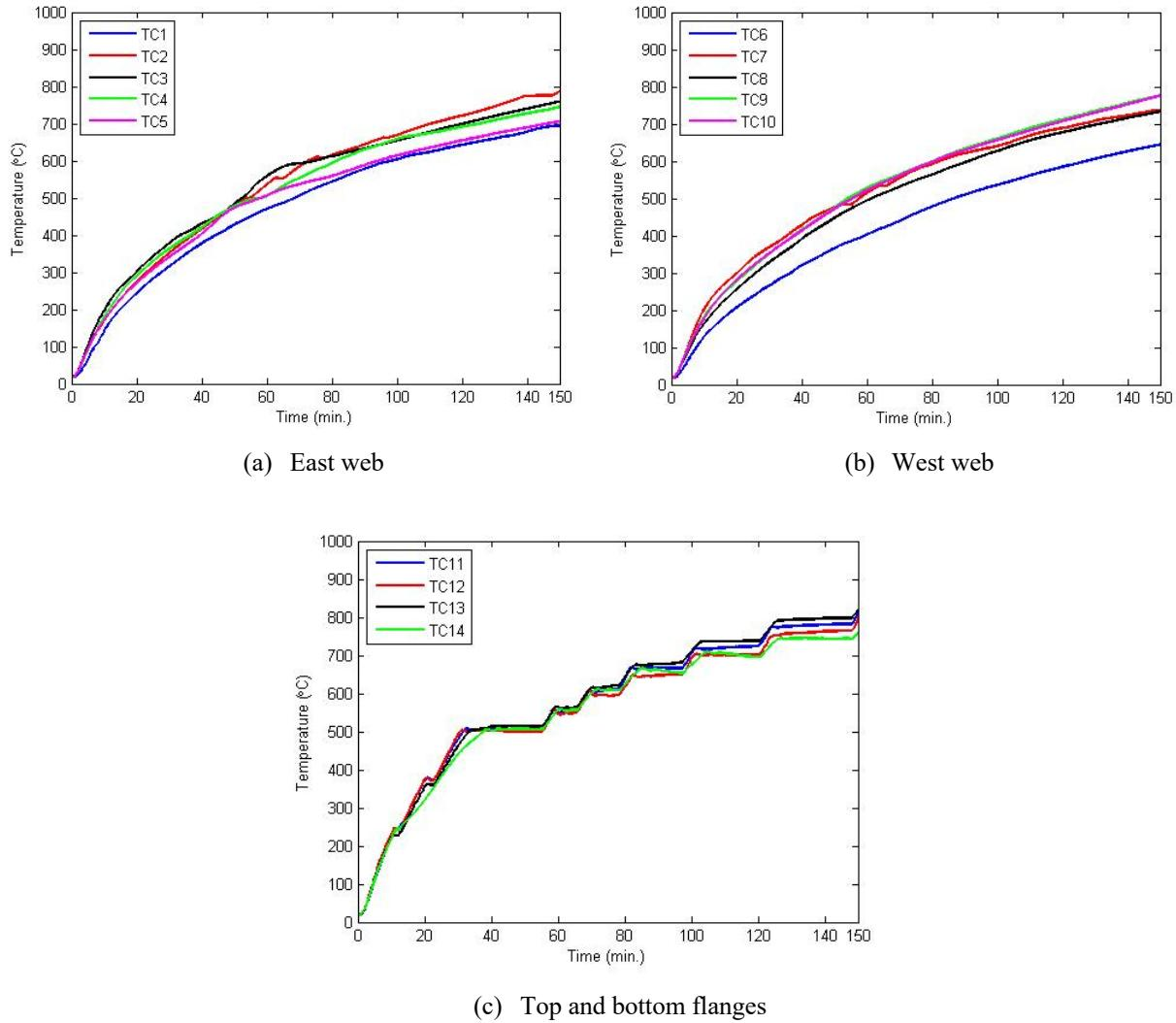
Fig. 2-42. The measured surface temperature of CW5
