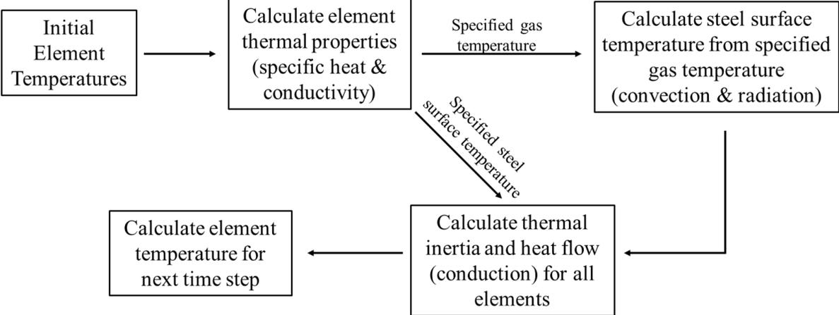
Fig. 4-3. Schematic flowchart of algorithm for 2D heat transfer
