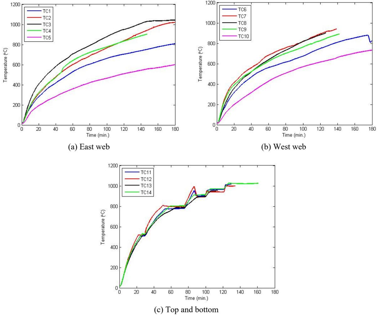
Fig. 2-16. The surface temperature of CW1 (Test 2)
