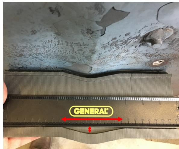
(d) Size of local buckling in CW1 with steel plate slenderness of 24
