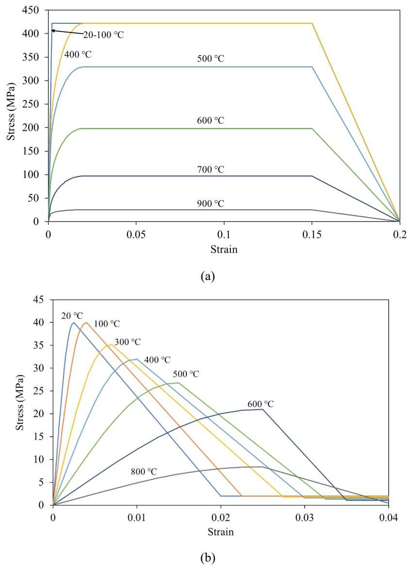
Fig. 4-8. Eurocode stress-strain-temperature curves for (a) 420 MPa steel and (b) 40 MPa concrete
