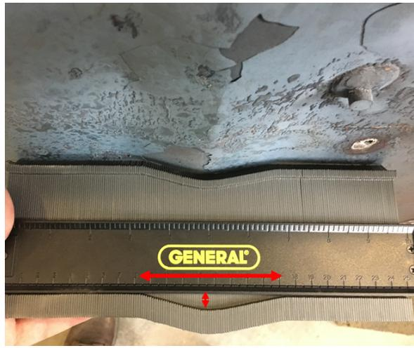
(d) Size of local buckling in CW1 with steel plate slenderness of 24
