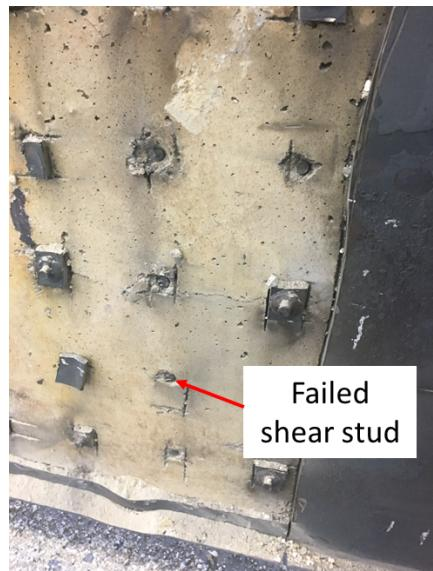
Fig. 2-19. Failed shear studs after the fire test
