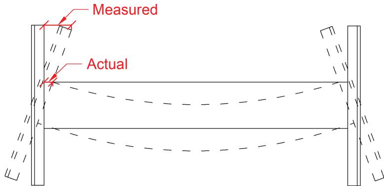
Fig. 2-22. Measured and actual axial displacement of the specimen (plan view)
