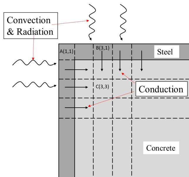
Fig. 4-2. Representation if the three modes of heat transfer: convection, conduction & radiation
