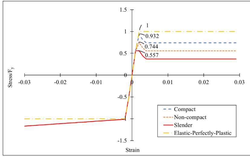
Fig. 4-9. Effective stress-strain curves for compact ( $\lambda=50$ ), non-compact ( $\lambda=67$ ) and slender ( $\lambda=100$ ) sections for steel ( $F_y=358$  MPa) at ambient temperature
