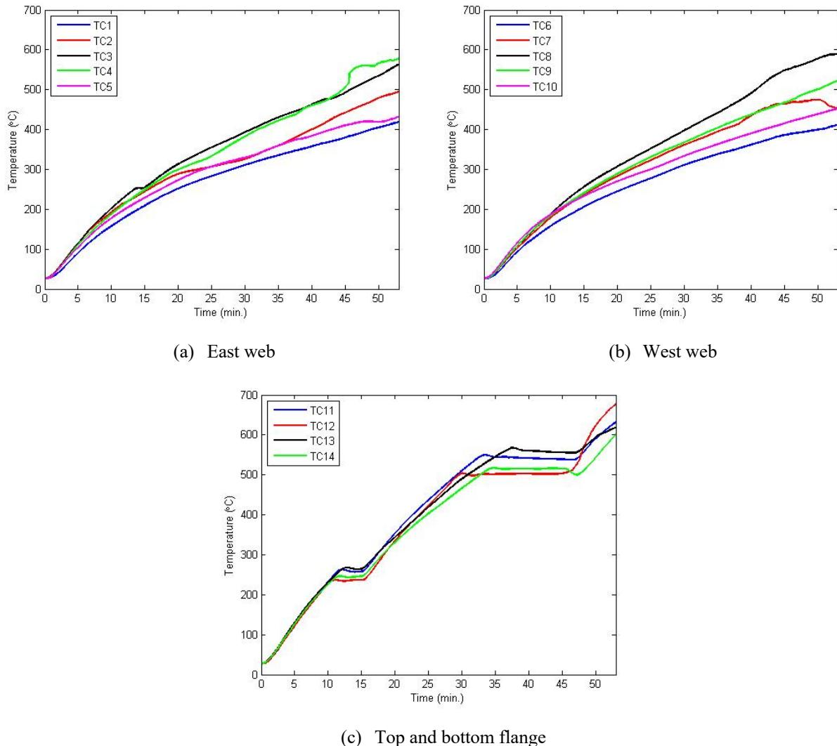
Fig. 2-34. The measured surface temperature of CW4 (Test1)
