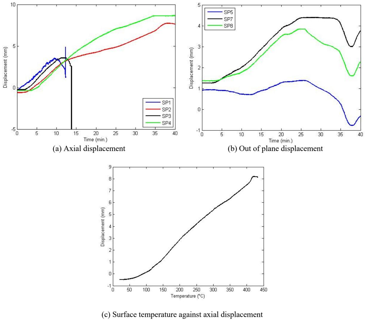
Fig. 2-14. Measured axial and out of plane displacements of CW1 (Test 1)
