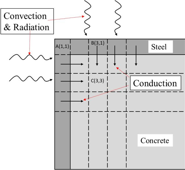
Fig. 4-2. Representation of the three modes of heat transfer: convection, conduction & radiation
