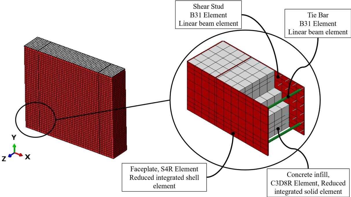
Fig. 3-1. 3-Dimensional model of the Concrete Filled Composite Plate Shear Walls
