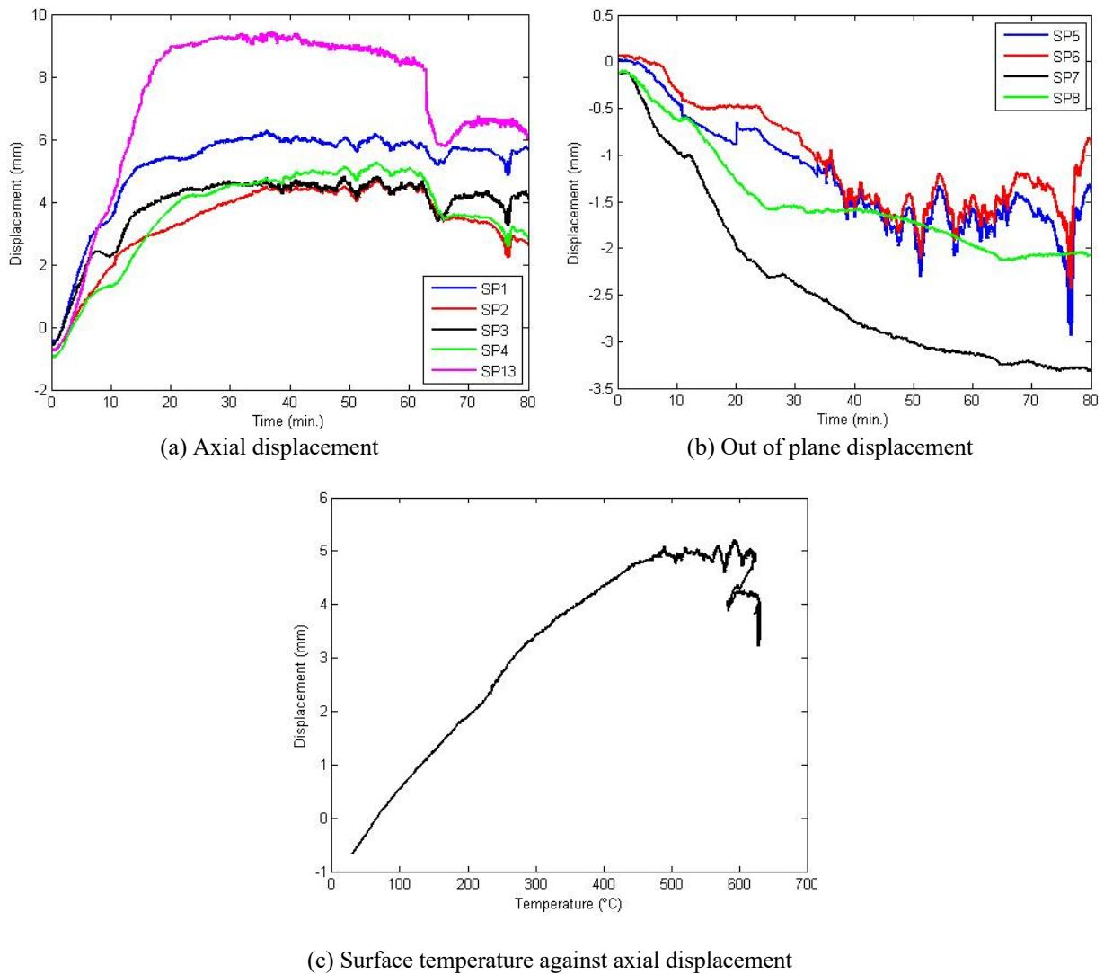
Fig. 2-32. Measured axial and out of plane displacements of CW3
