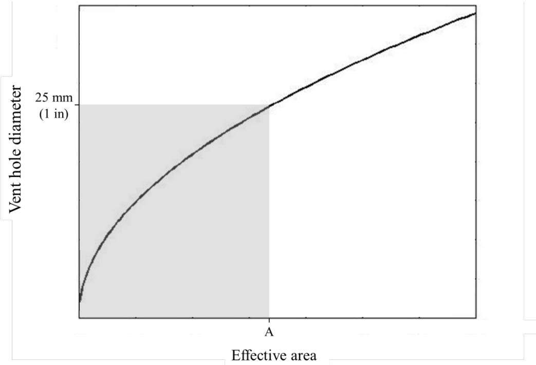
Fig. 5-4. The covered range of effective area by using a minimum vent hole size
