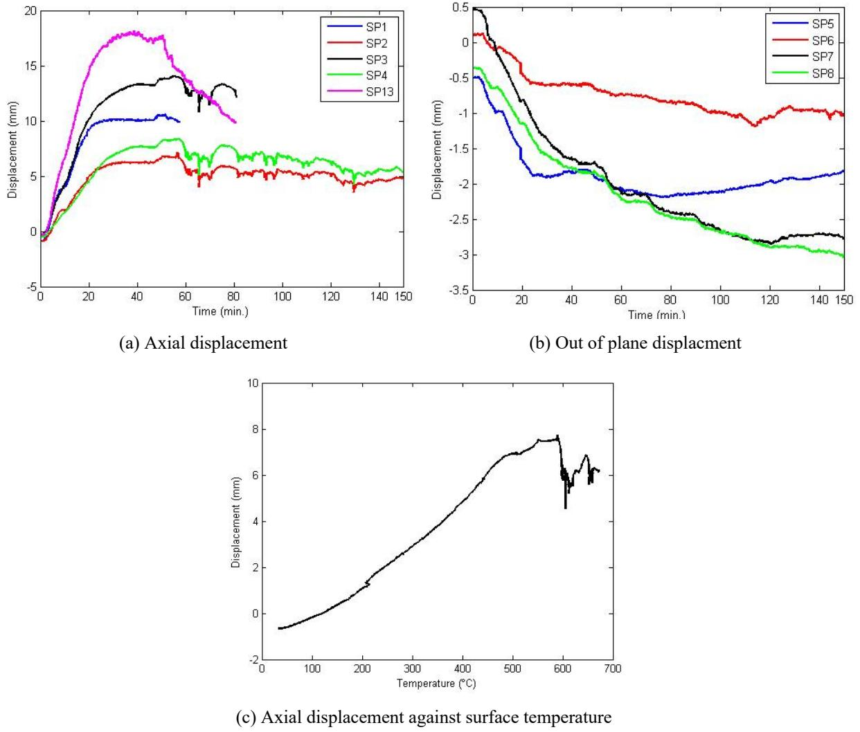
Fig. 2-39. Measured axial and out of plane displacements of CW4 (Test2)
