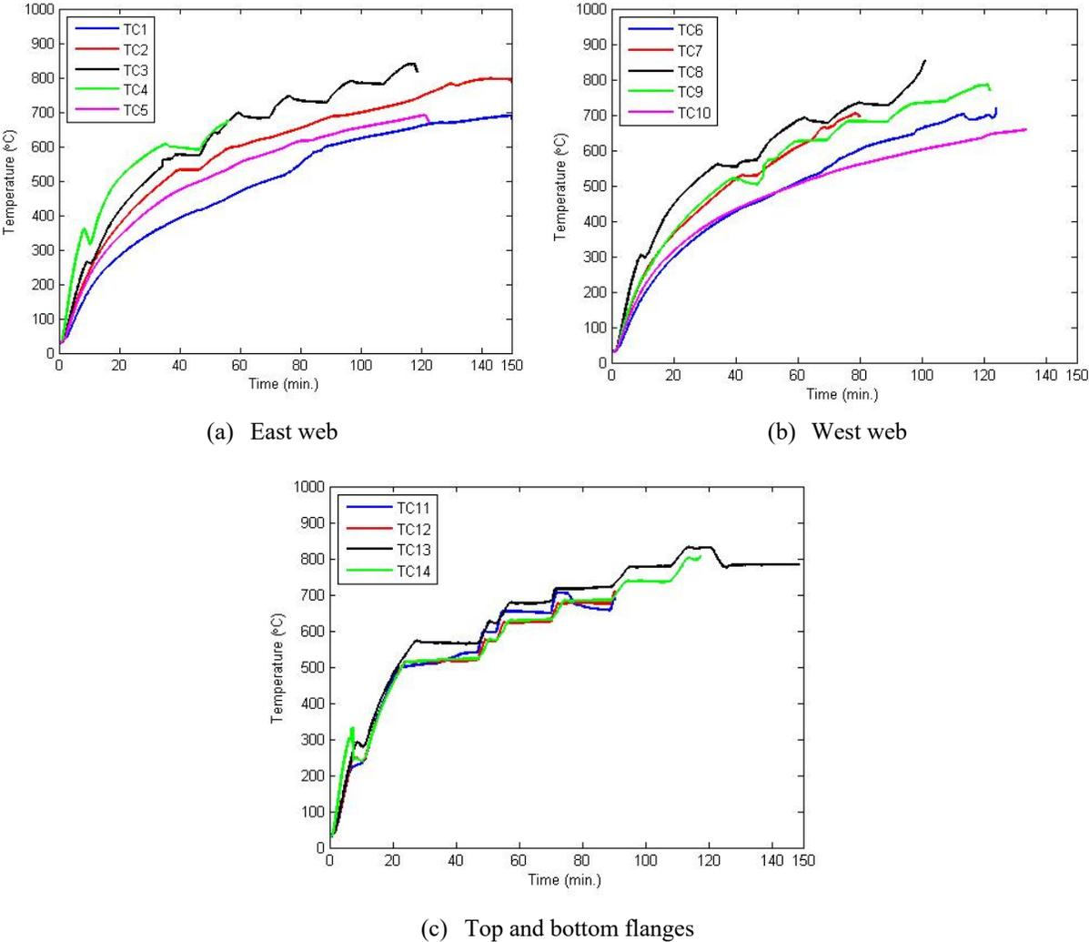
Fig. 2-38. The measured surface temperature of CW4 (Test2)
