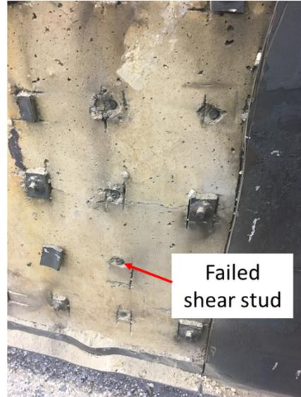
Fig. 2-19. Failed shear studs after the fire test
