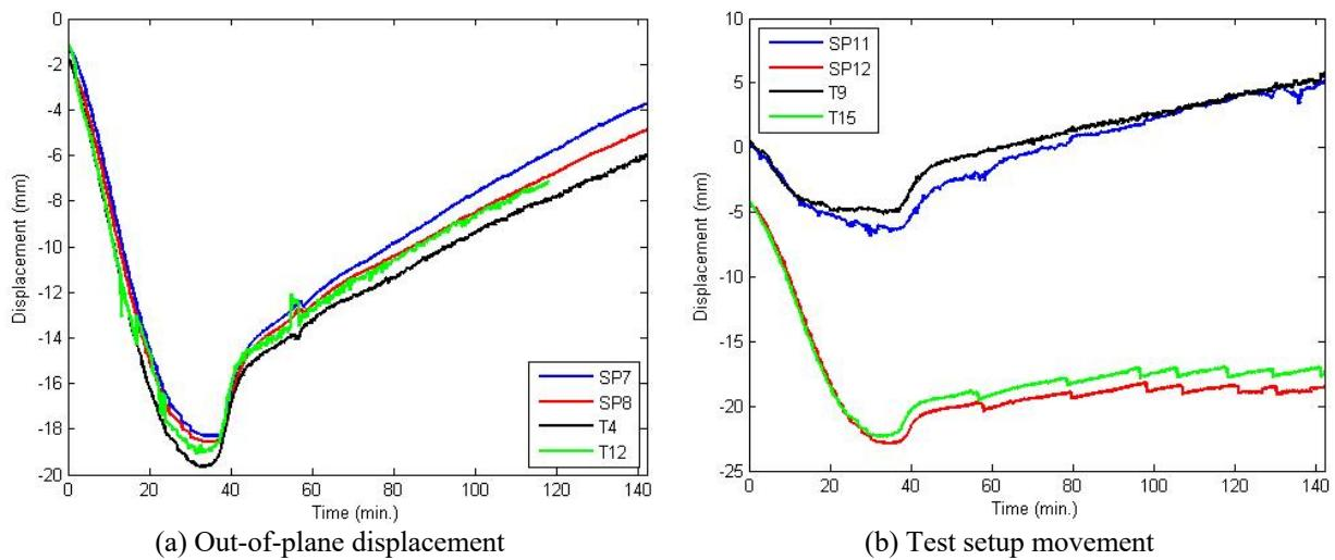
Fig. 2-27. Comparison of measured displacement by string potentiometer and OptiTrack.
