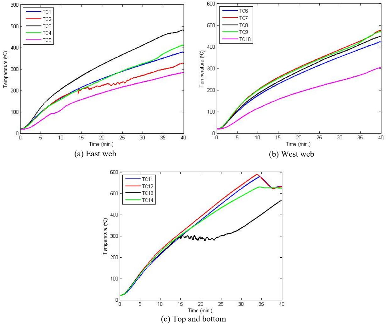
Fig. 2-13. The surface temperature of CW1 (Test 1)
