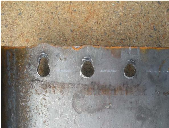
Figure 113. Bearing deformations of the bolt holes in the beam's web.
