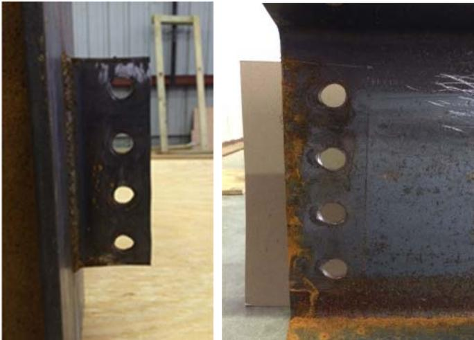
Figure 134. Bearing deformations in test 7 (center column, right side).
