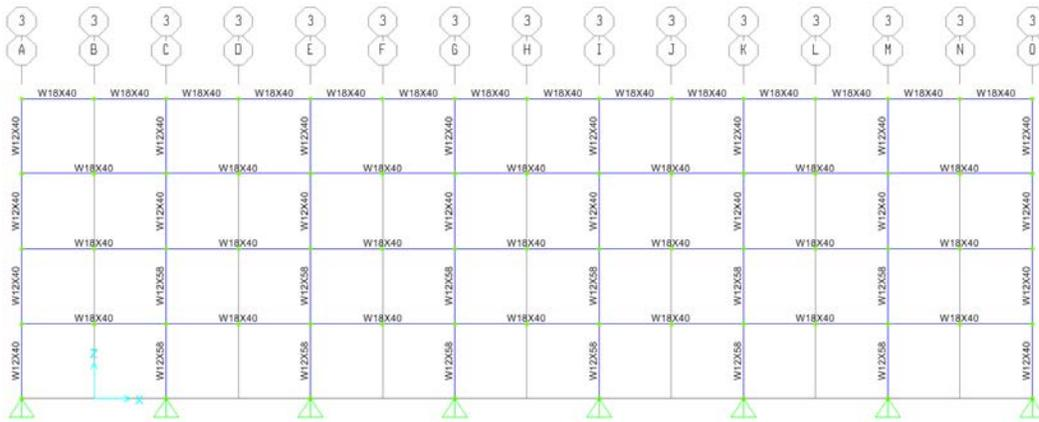
e. Elevation view of NS external frame (left) and internal frame (right)
