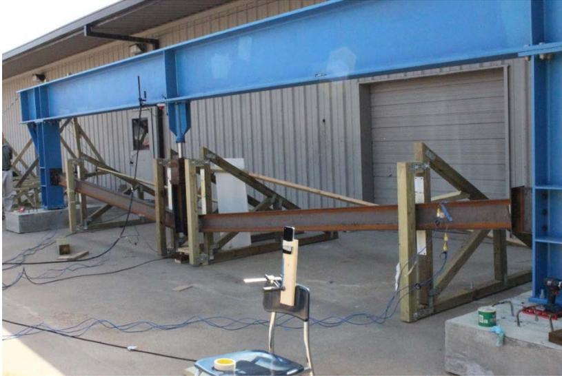
Figure 110. Test 2 undergoing large deformations.
