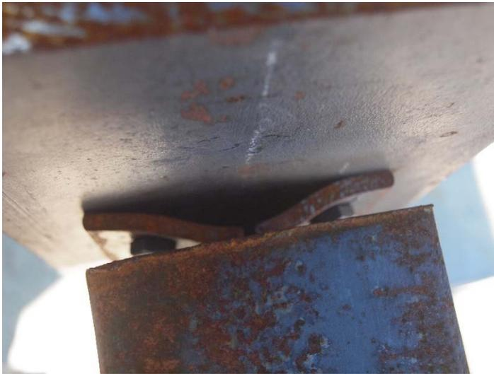
Figure 118. Test 3 prying deformations.
