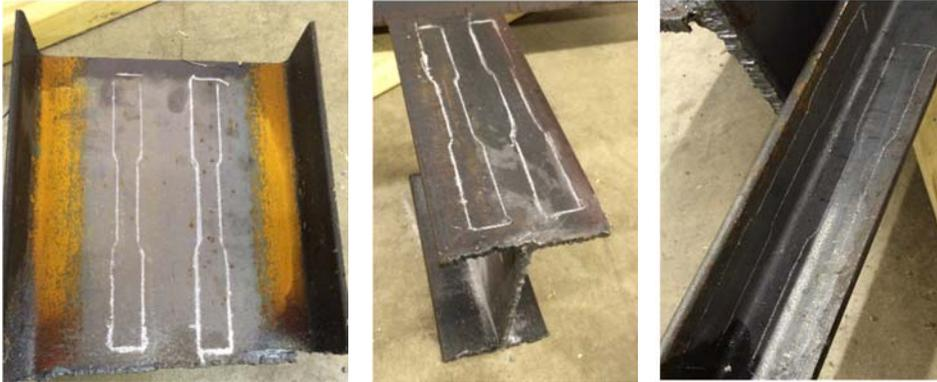
Figure 106. Base material for tensile coupons.
