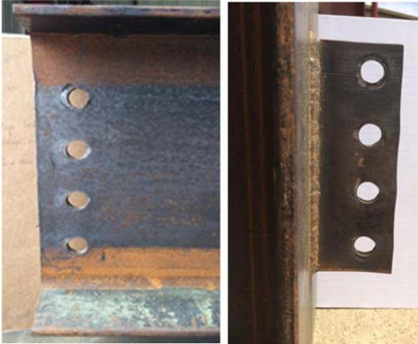
Figure 139. Test 8 bearing deformations.
