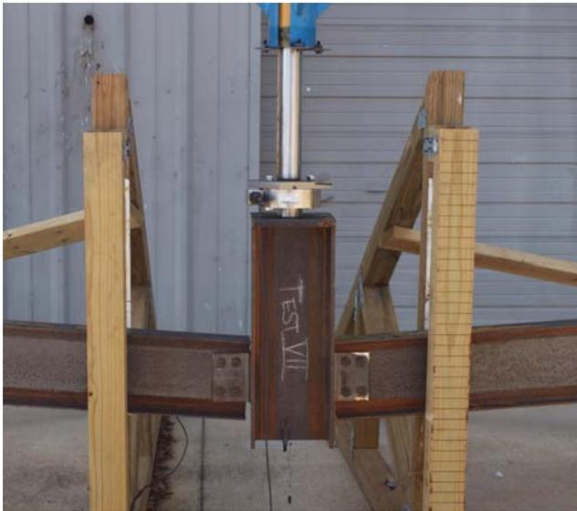
Figure 142. Test 9 central (missing column) under large deformations.
