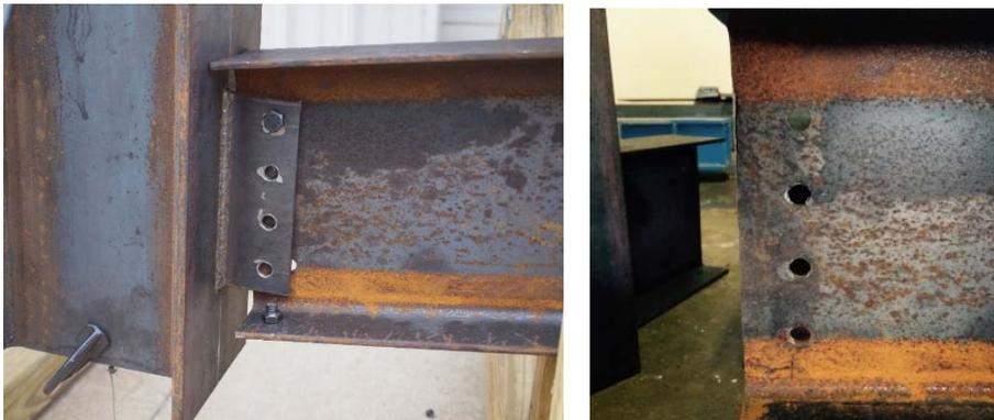
Figure 123. Test 5 shear tab with failed bolts (left), bearing deformations (right).
