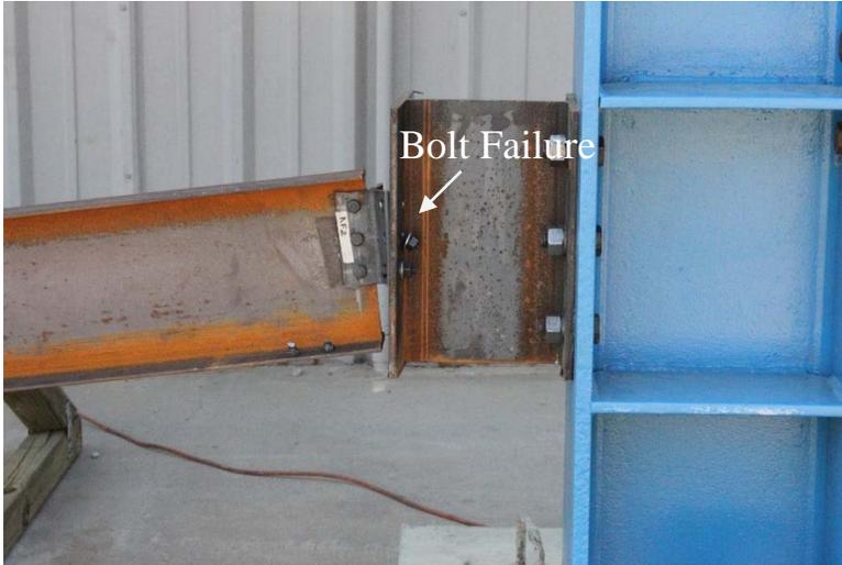
Figure 112. Failure of bolts during Test 2.
