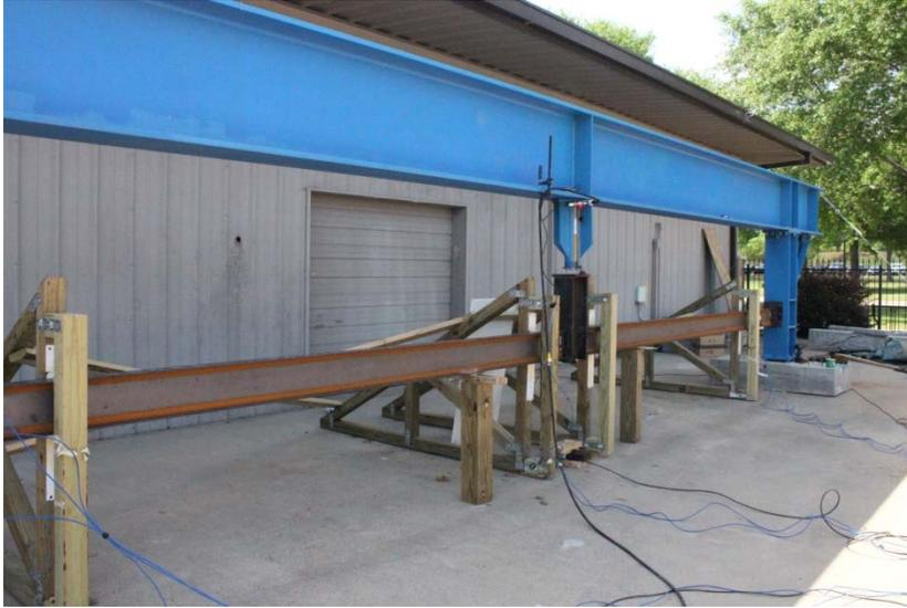
Figure 100. Photo of test frame and specimen showing lateral braces.
