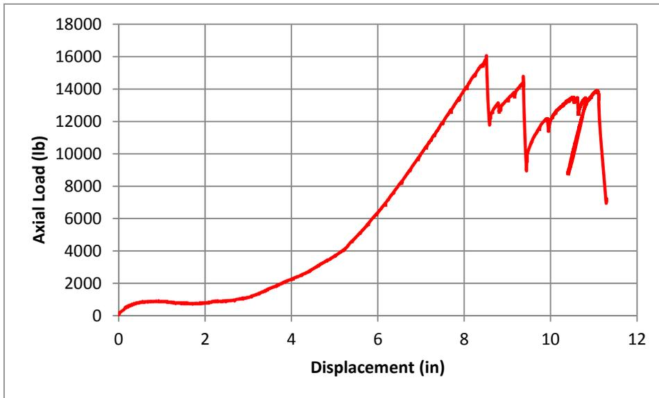
Figure 128. Test 6 axial force vs. displacement.
