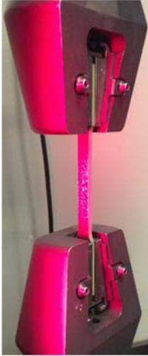
Figure 108. Material coupon loaded in Instron 5582 testing machine.
