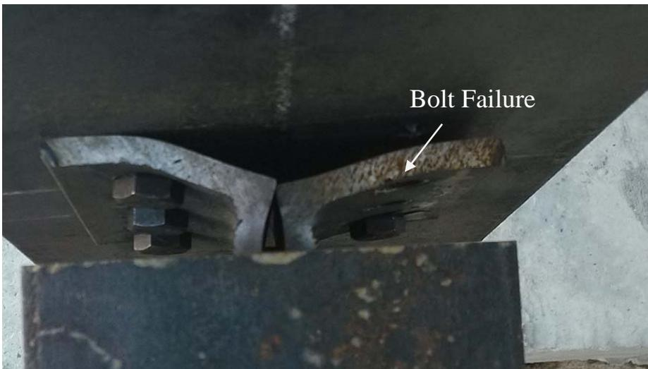
Figure 111. Failure of top two bolts on right angle, Test 1.
