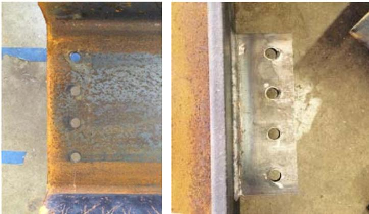
Figure 129. Test 6 bearing deformations.
