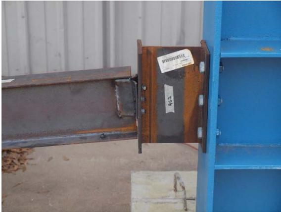
Figure 119. Test 4 bolt fracture.
