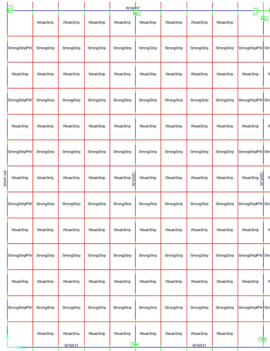
Figure 85. Typical shell element layout of one bay in American Zinc building.
