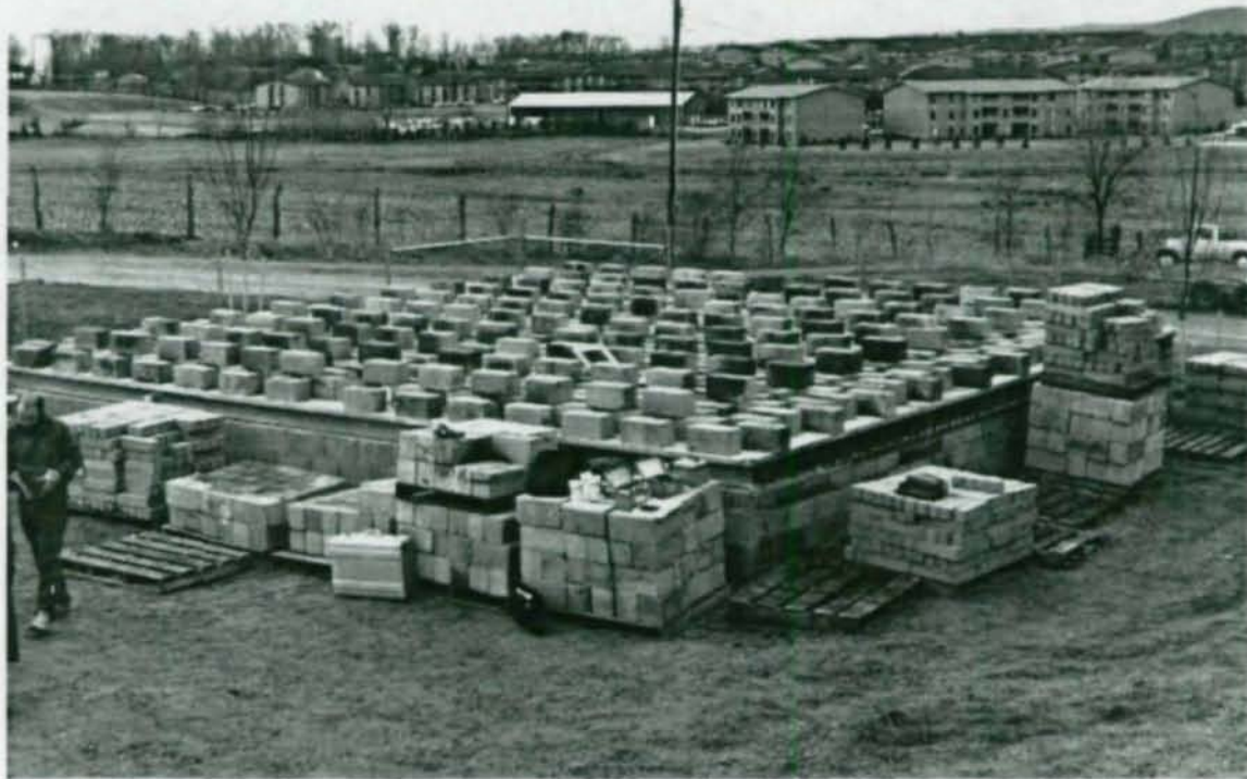
Figure 3.7 Load Test of Experimental Floor
