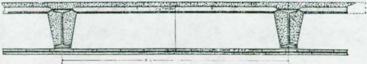
ROEBLING SYSTEM B, TYPE 1, FLAT SLAB CONSTRUCTION Adapted for Public Buildings, Offices, Theatres, Churches, Schools, Hospitals, Hotels, Residences, etc. Capacity in 6 ft. spacing of beams, 1500 lbs. per square foot
