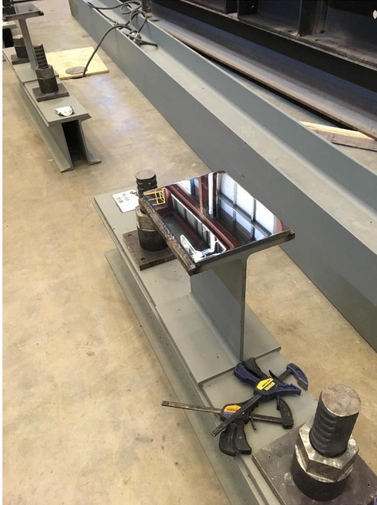
Fig. H-2: Typical bearing support
