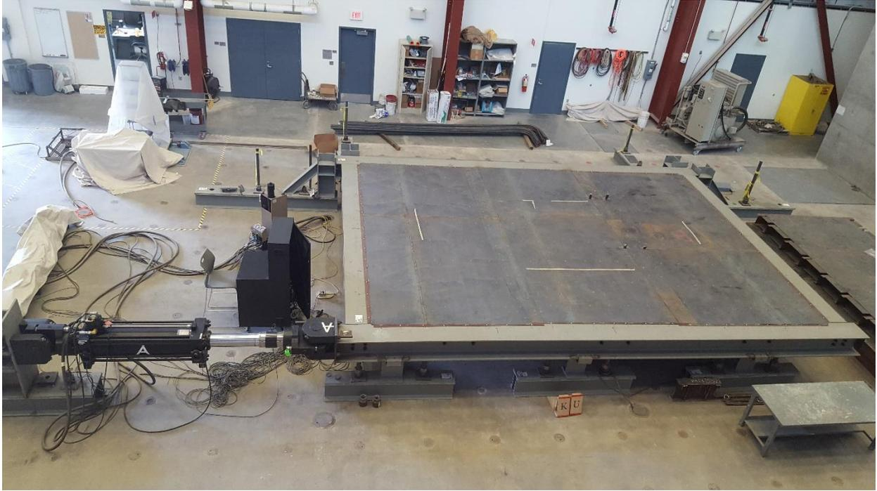
Fig. H-5: Final floor assembly for diaphragm testing
