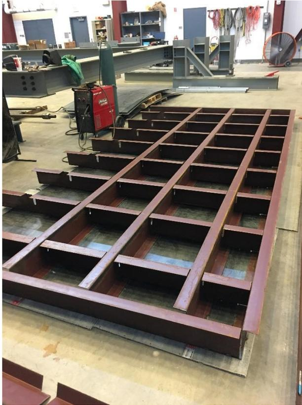
Fig. 7- 3: Orthogonally arranged purlins
