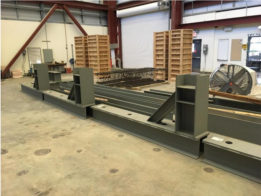
Fig. K-1. Typical brace assembly
