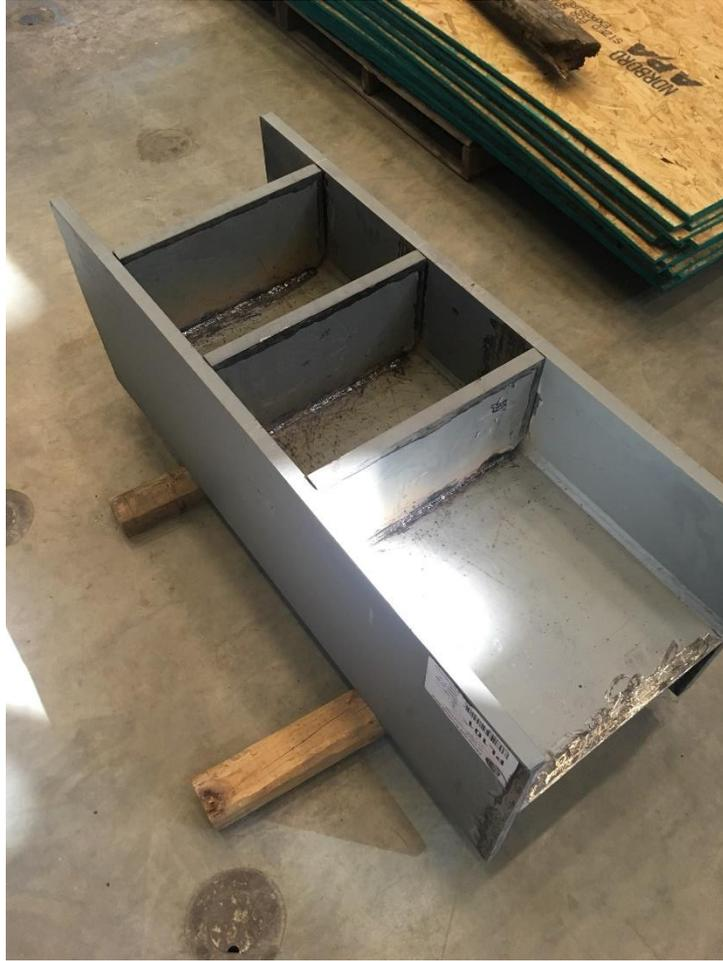
Fig. K-3. Actuator brace assembly
