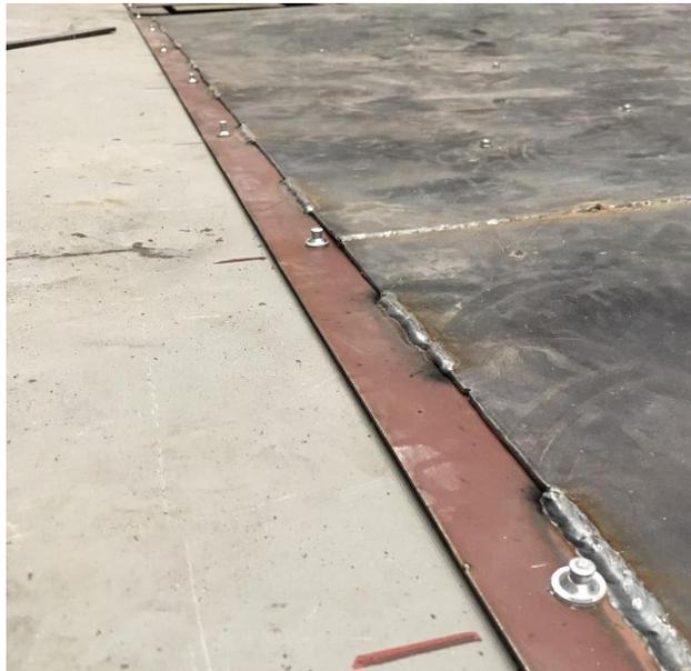
Fig. 7- 8: Perimeter purlins nailed to the flanges of the test frame girders using Hilti brand powder actuated fasteners
