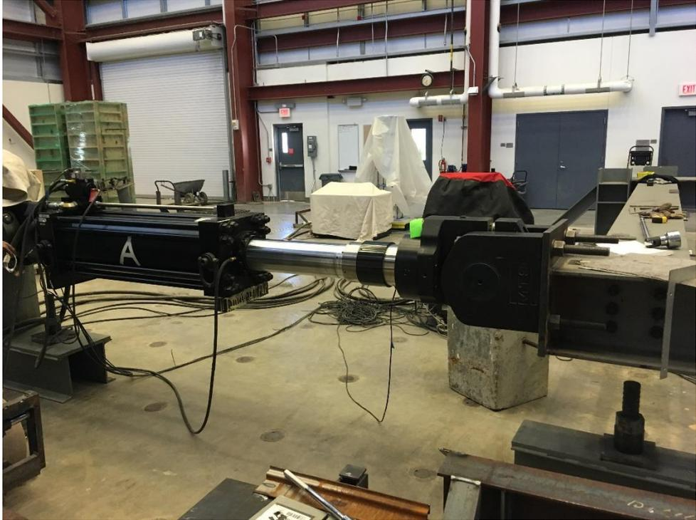
Fig. H-4: 980 kN (220 kip) Actuator attachment
