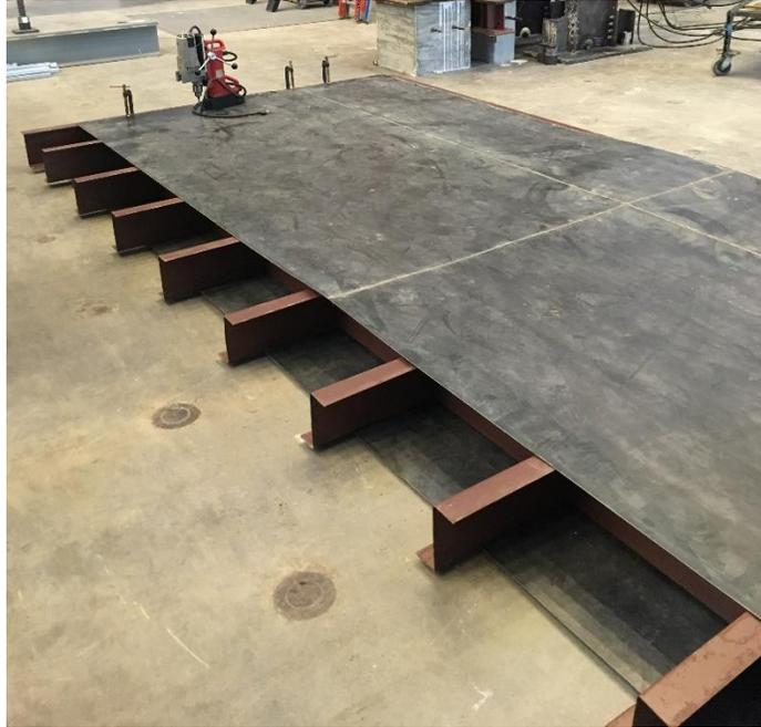
Fig. M -9. Top plate set in place to form single panel
