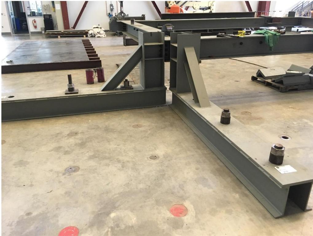
Fig. H-1: Typical frame corner brace
