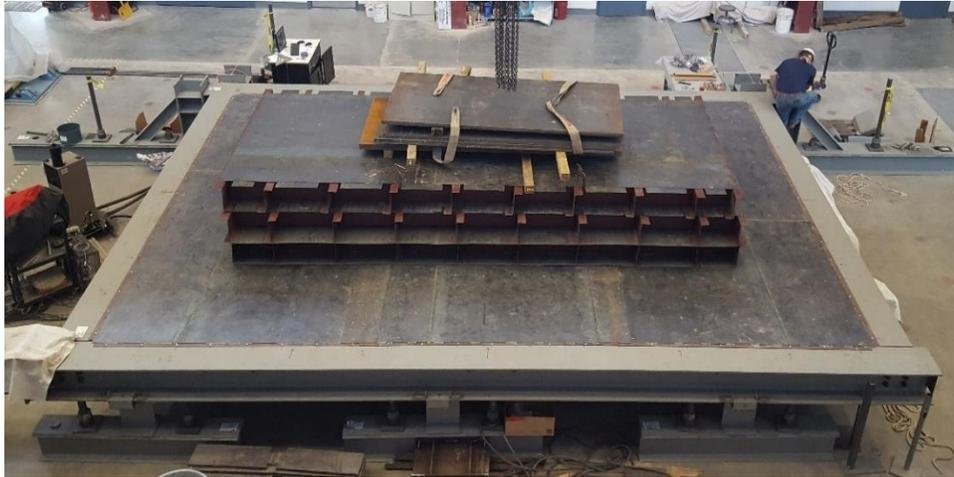
Fig. 4- 4: Floor diaphragm assembly showing preliminary gravity loads
