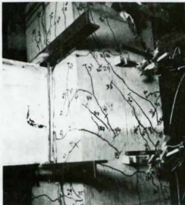
Fig. 4.7 A view of joint 2 after cycle U1. (Upper left flange in compression)
