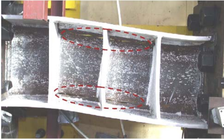
Figure 1.5 Web fractures initiating from the ends of stiffener-to-web welds in UTA short links (Specimen 4A, Arce, 2002)
