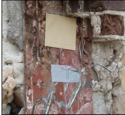
Figure 3.2- Strain Gauge Attached to a Column with a Cover Shield Applied.
