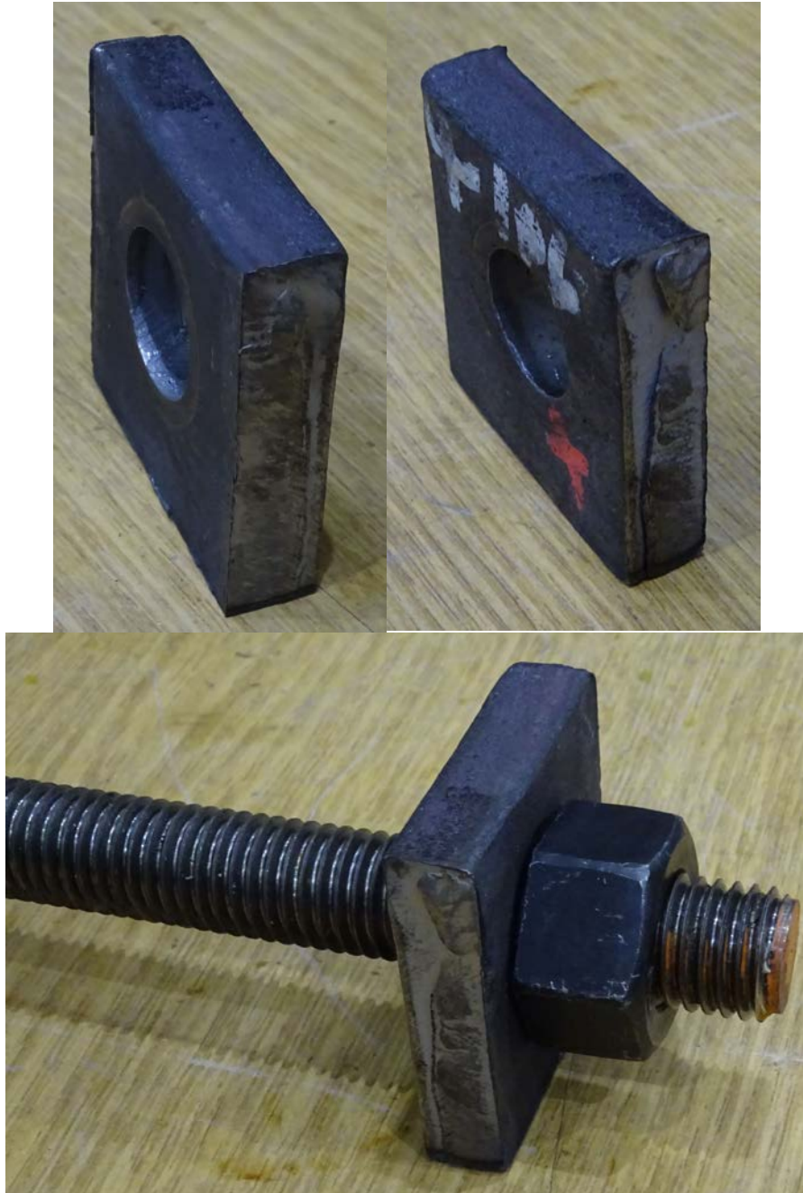
Figure B.13: Test #13 - 5% Relative Deformation
