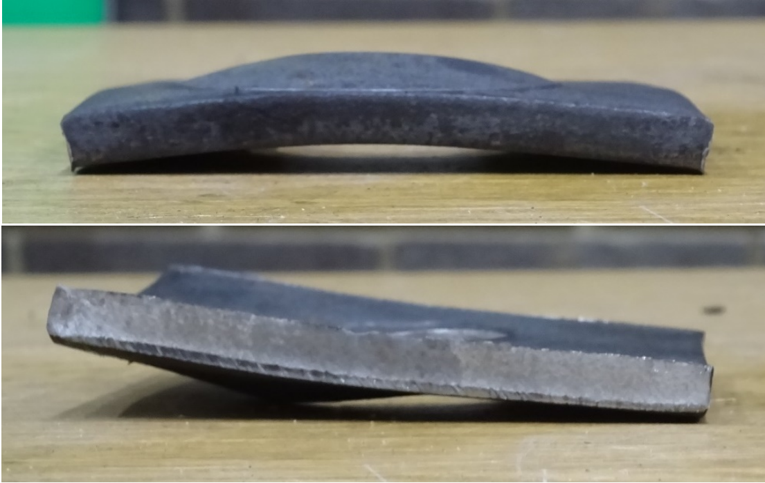
Figure 3.15: 1/4" Plate Washer, Offset - 1" Gr. 36 Rod
