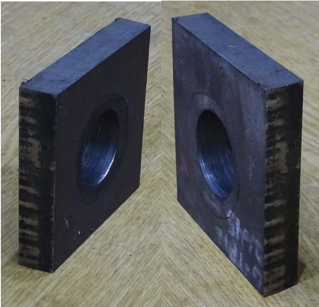
Figure B.52: Test #52 - 6% Relative Deformation
