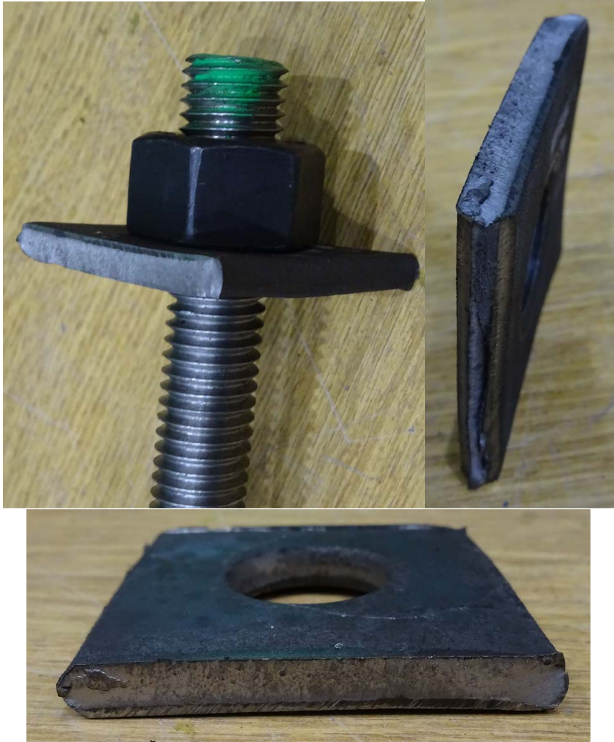
Figure B.5: Test #5 - 25% Relative Deformation
