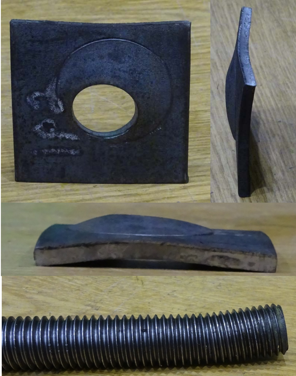
Figure 3.17: 1/4" Plate Washer, Offset - 1" Gr. 55 Rod
