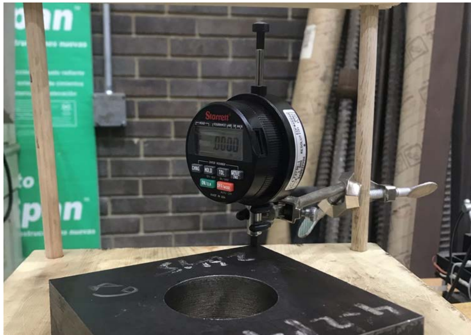
Figure 3.2: Close-up of Affixed Dial Gauge
