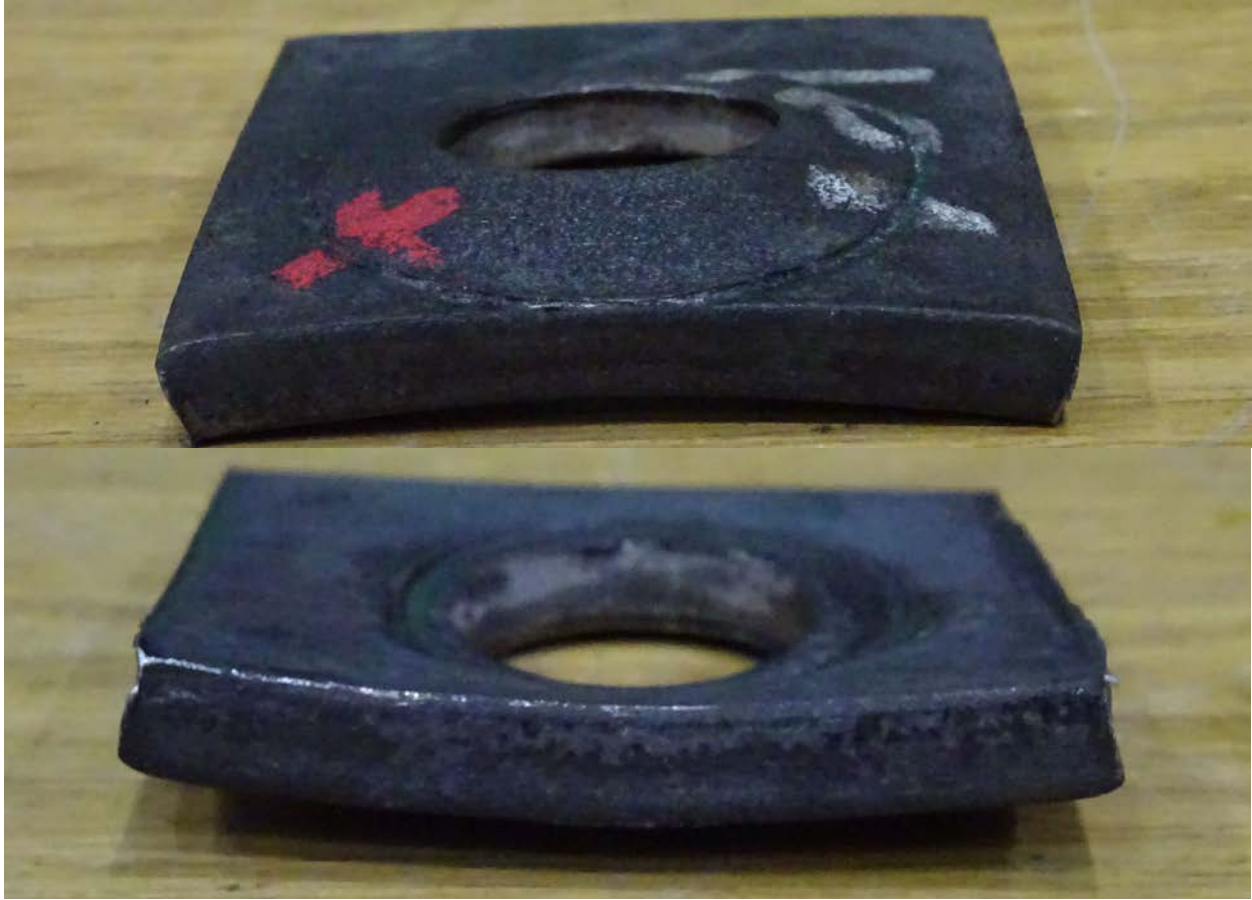
Figure 3.13: 1/4" Plate Washer, Offset - 0.75" Gr. 105 Rod
