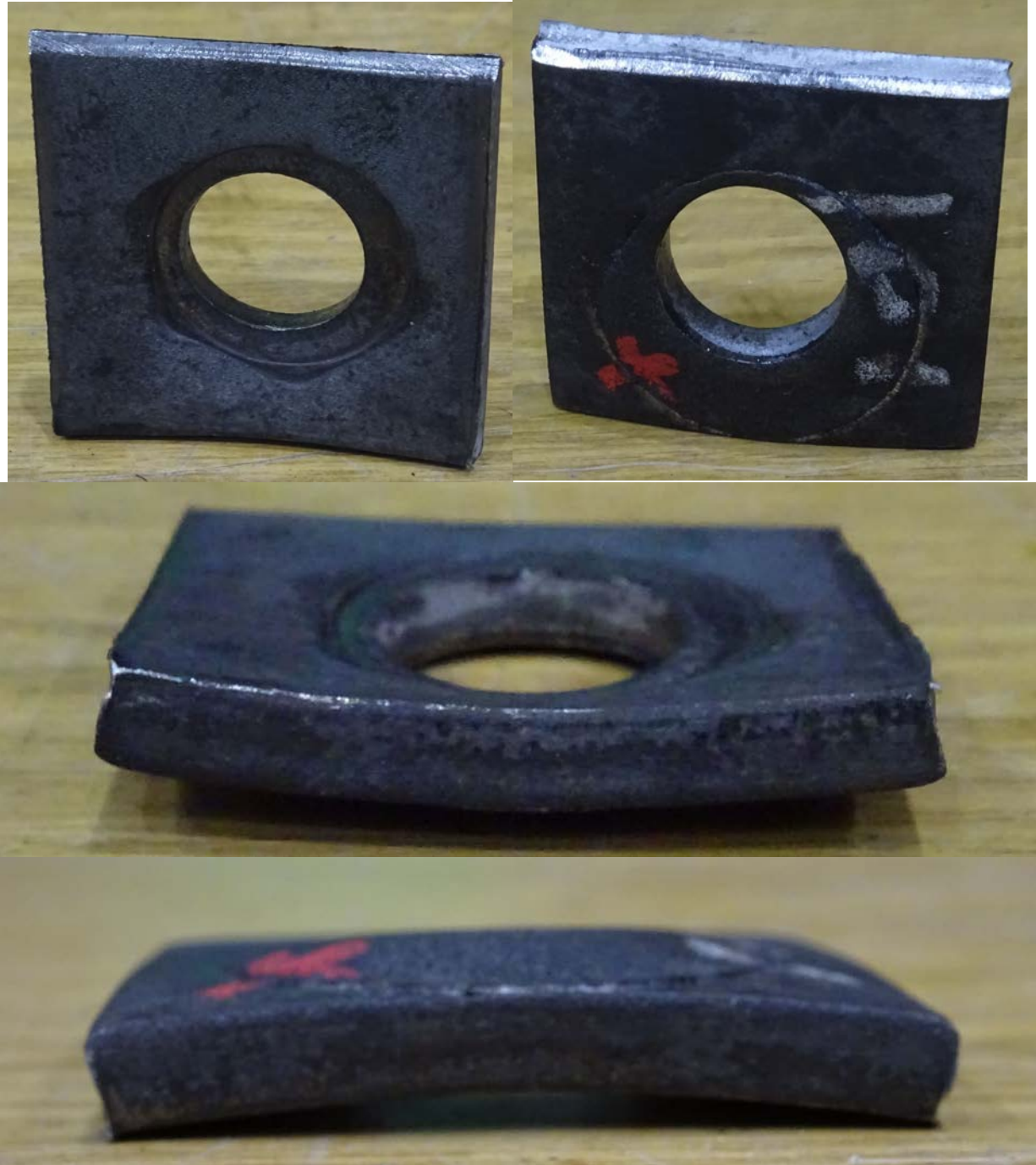
Figure B.17: Test #17 - 71% Relative Deformation
