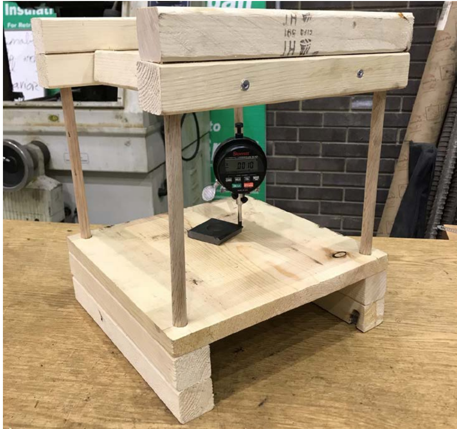
Figure 3.1: Assembly of Stage, Dowels and Affixed Dial Gauge
