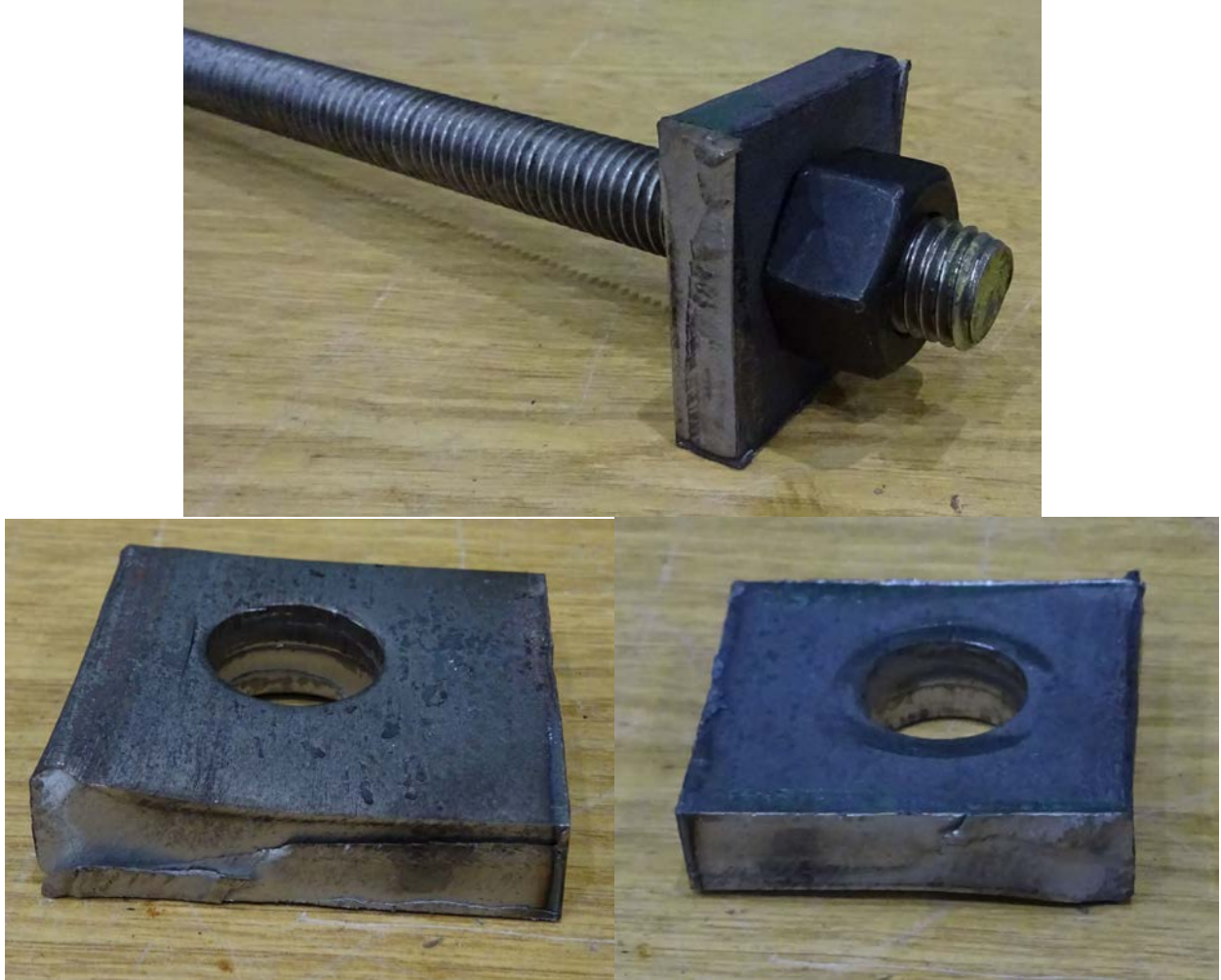
Figure B.8: Test #8 - 17% Relative Deformation
