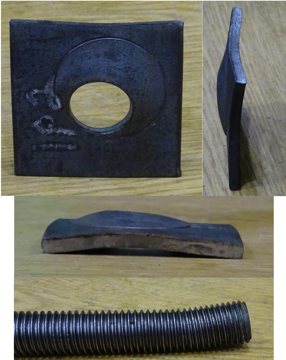
Figure B.29: Test #29 - 138% Relative Deformation and Rod Bending
