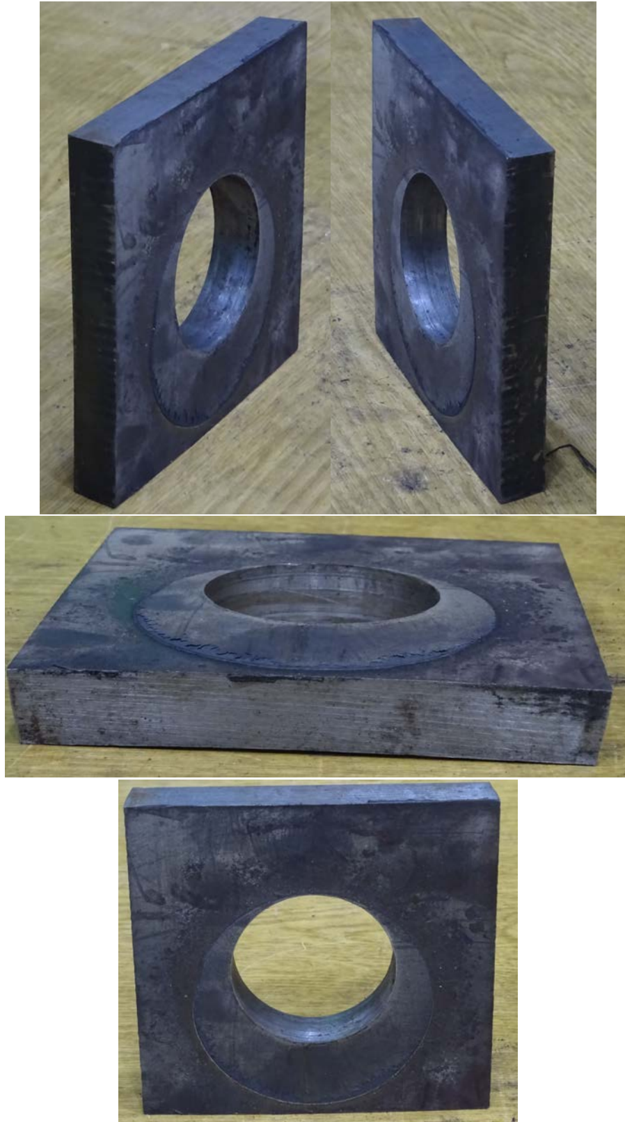
Figure B.94: Test #90 - 17% Relative Deformation
