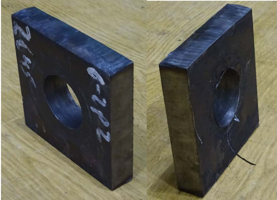
Figure B.66: Test #62 - 6% Relative Deformation
