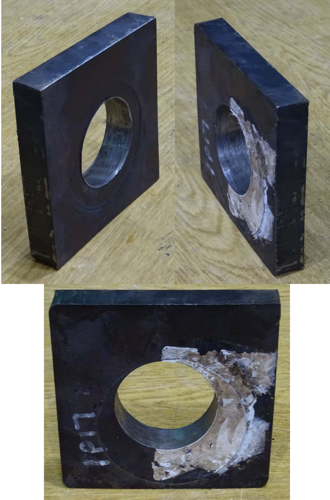
Figure B.79: Test #75 - 12% Relative Deformation
