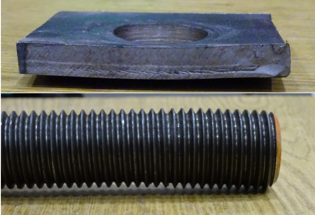
Figure 3.25: 1/2" Plate Washer, Offset - 1.5" Gr. 105 Rod
