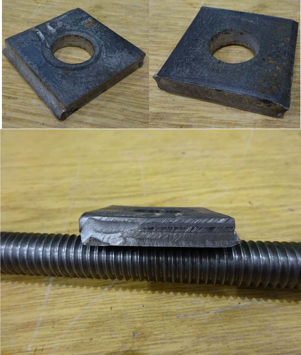
Figure B.3: Test #3 - 6% Relative Deformation
