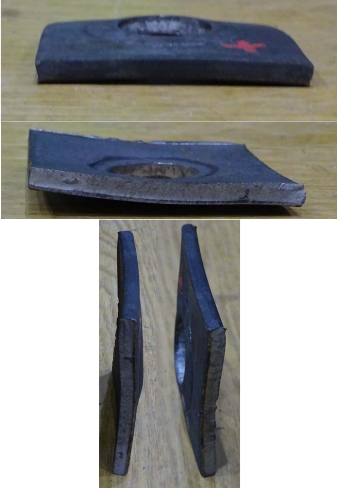
Figure B.23: Test #23 - 97% Relative Deformation
