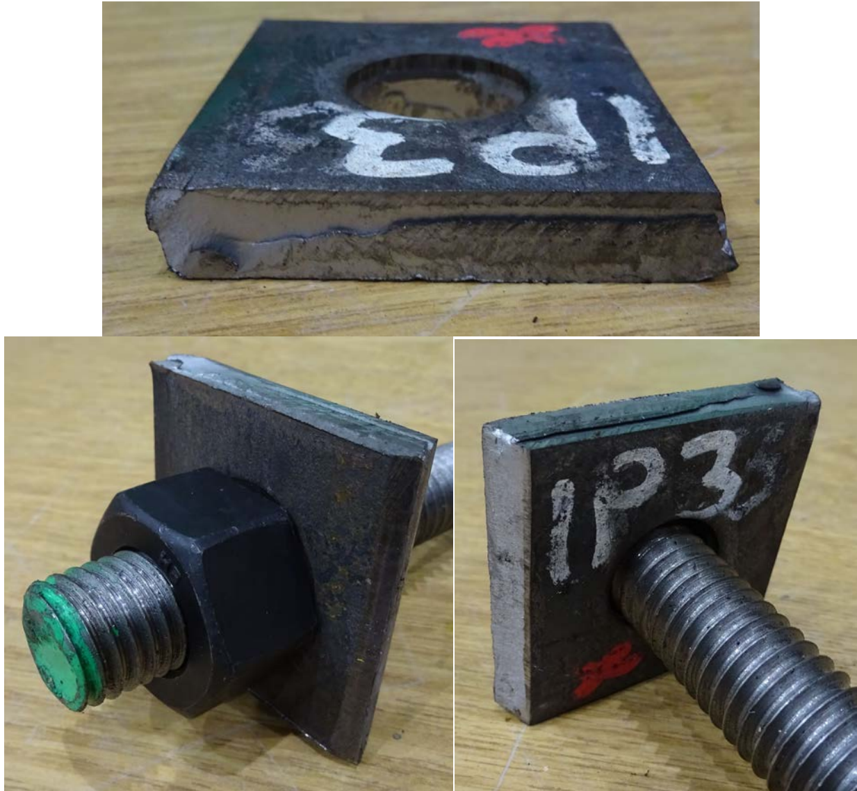
Figure B.4: Test #4 - 4% Relative Deformation
