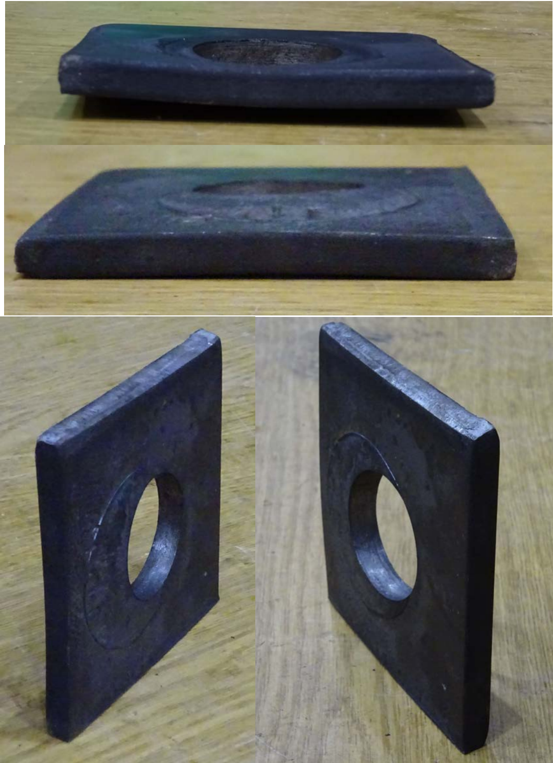
Figure B.47: Test #47 - 45% Relative Deformation
