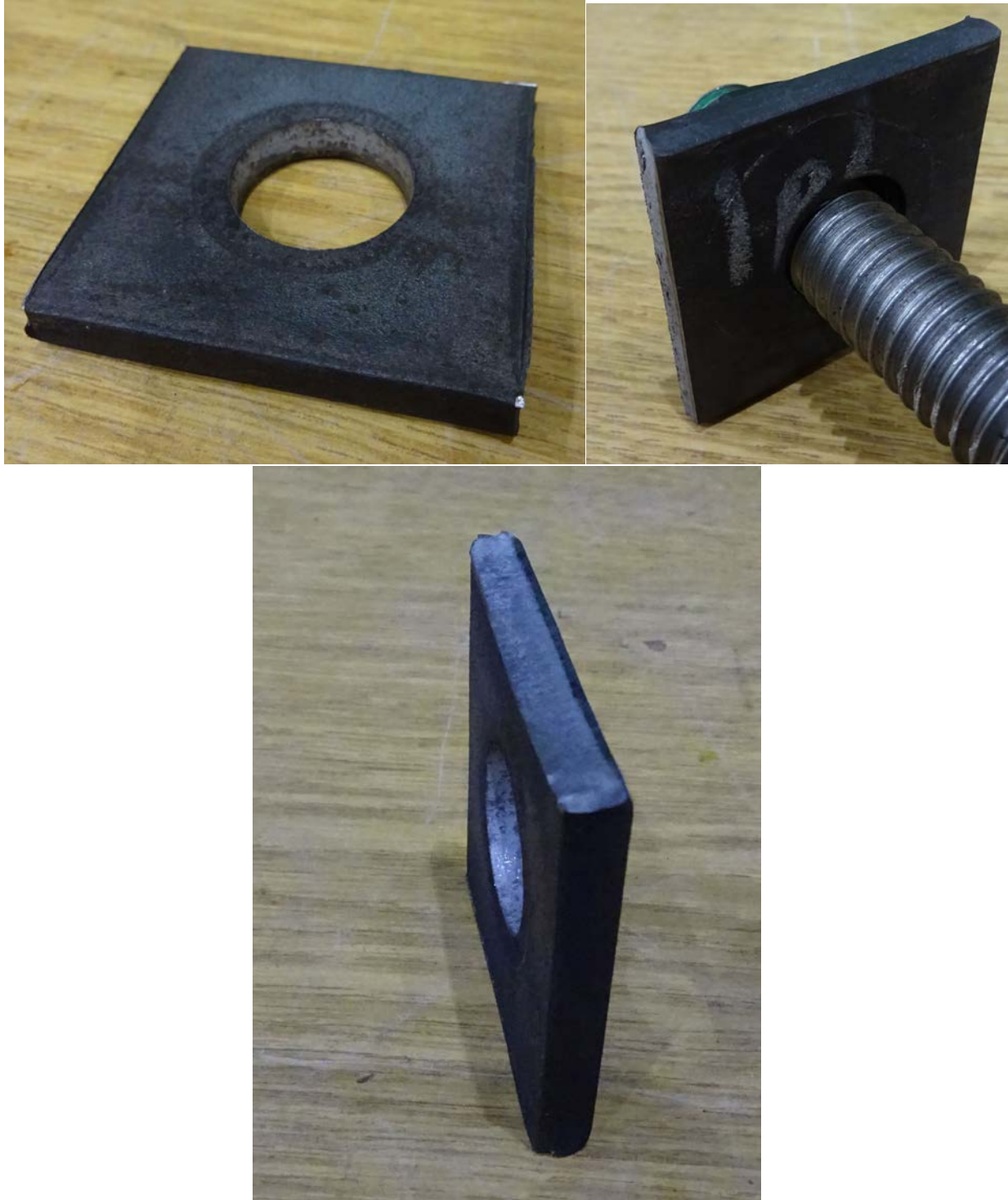
Figure B.6: Test #6 - 11% Relative Deformation
