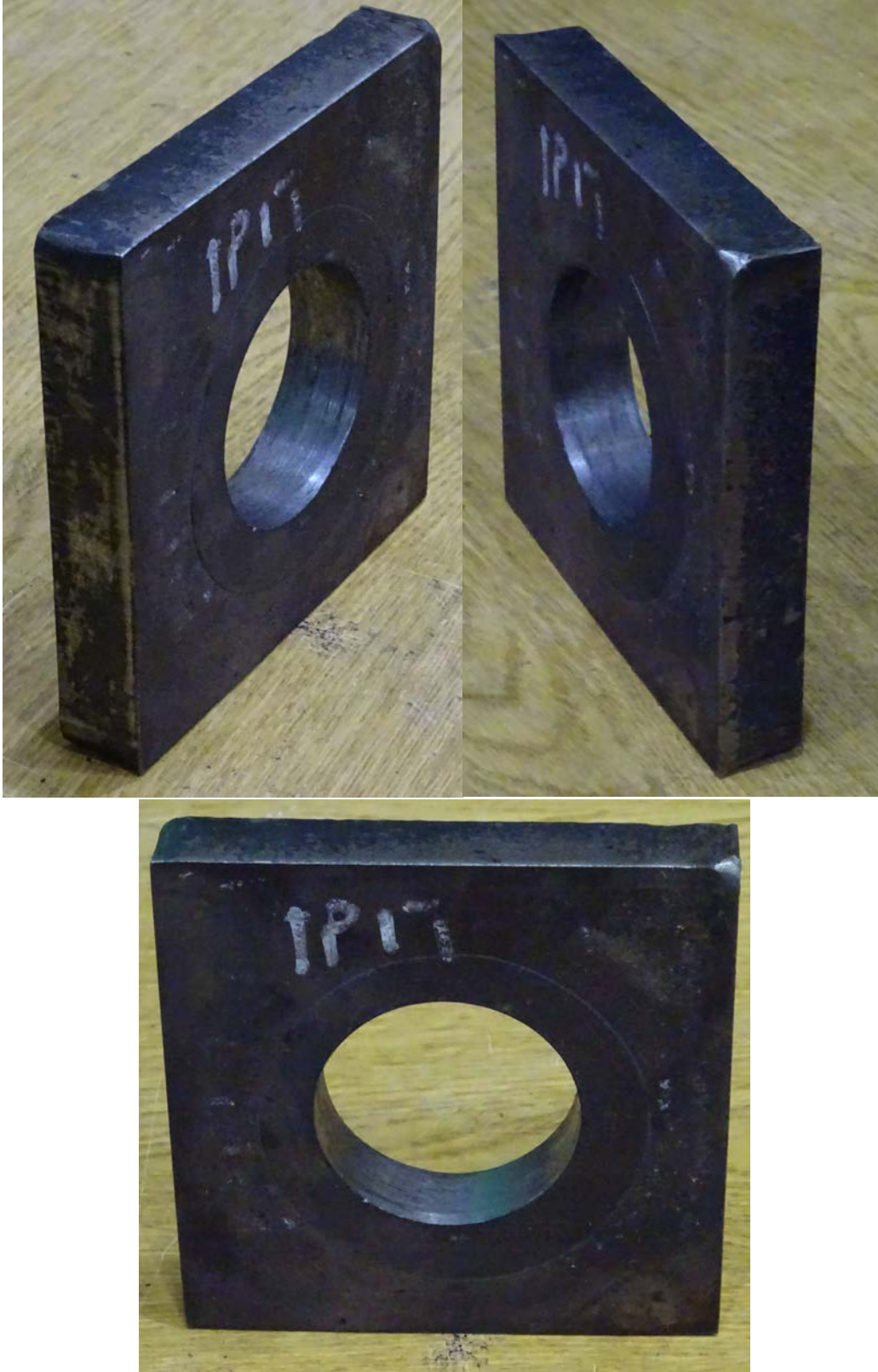
Figure B.80: Test #76 - 9% Relative Deformation
