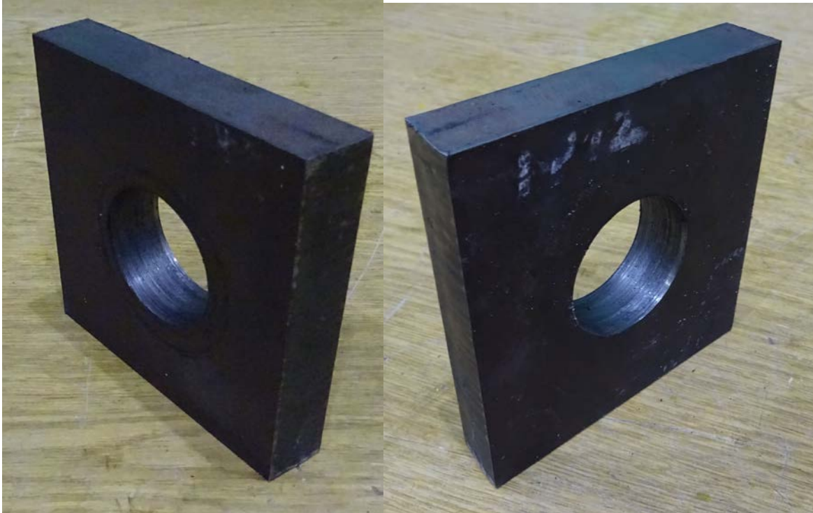
Figure B.38: Test #38 - 4% Relative Deformation
