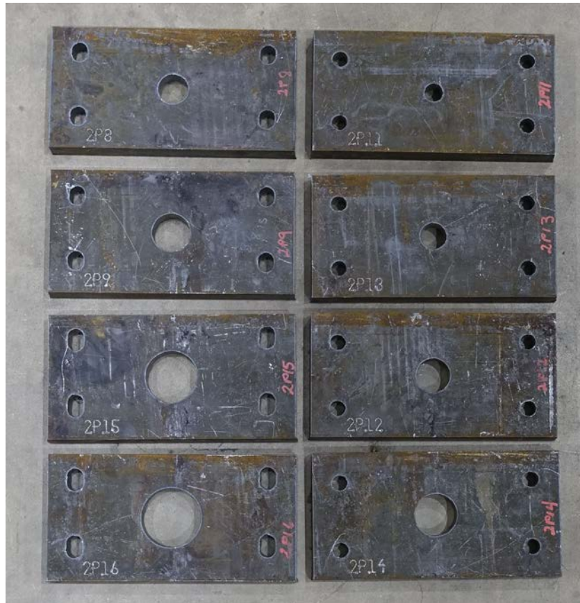
Figure 2.2: Bottom (left) and Top (right) Reaction Plates
