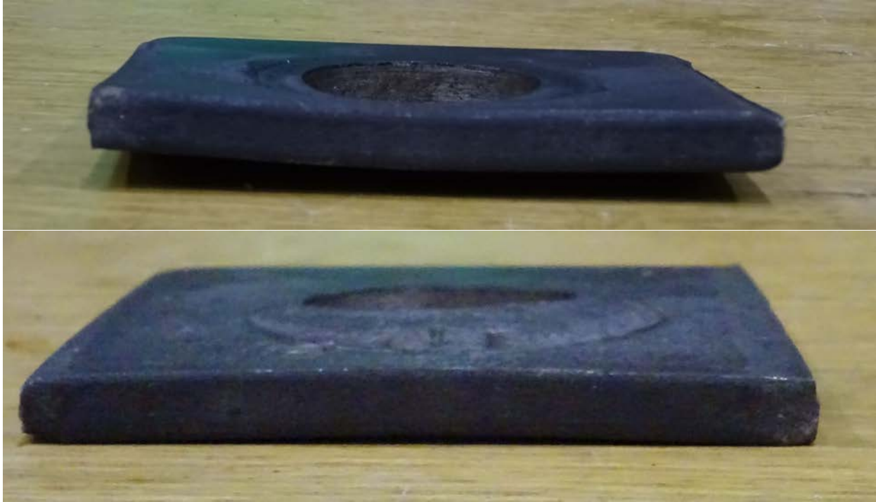
Figure 3.23: 3/8" Plate Washer, Offset - 1.5" Gr. 55 Rod
