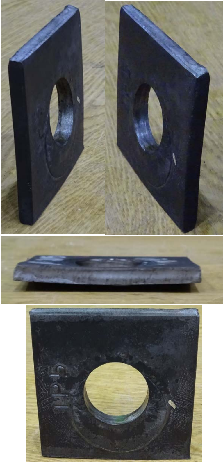
Figure B.42: Test #42 - 52% Relative Deformation
