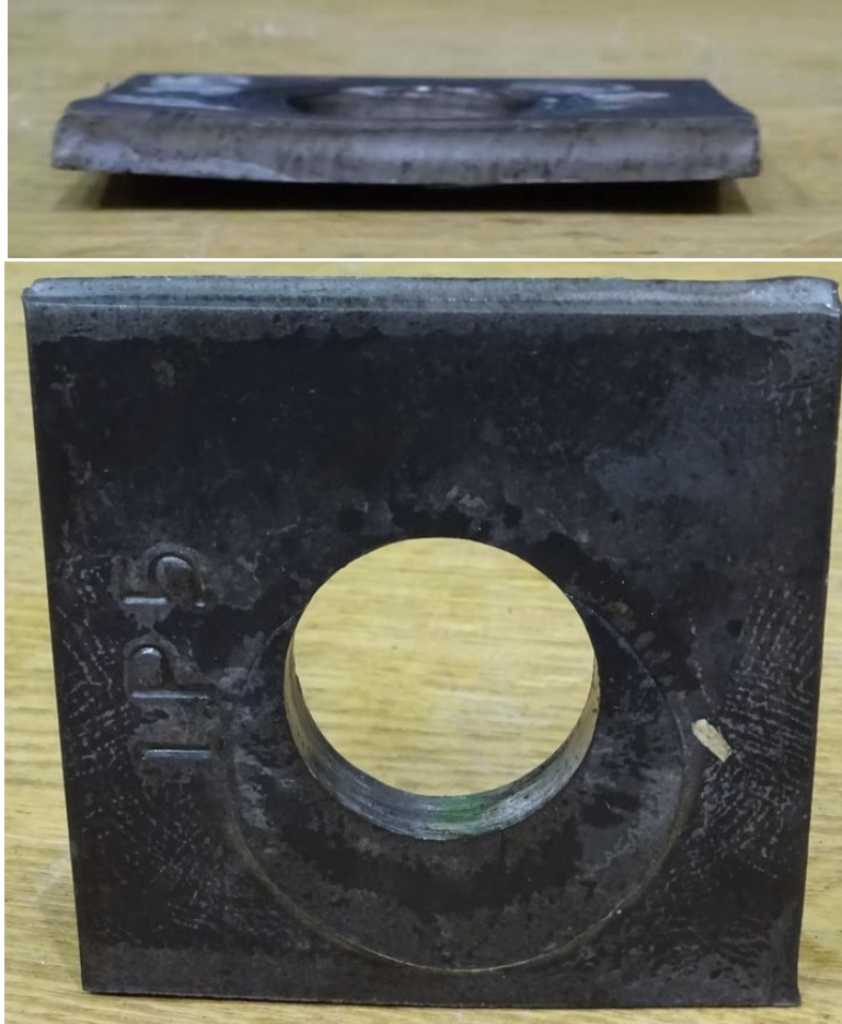
Figure 3.21: 3/8" Plate Washer, Offset – 1.5" Gr. 36 Rod
