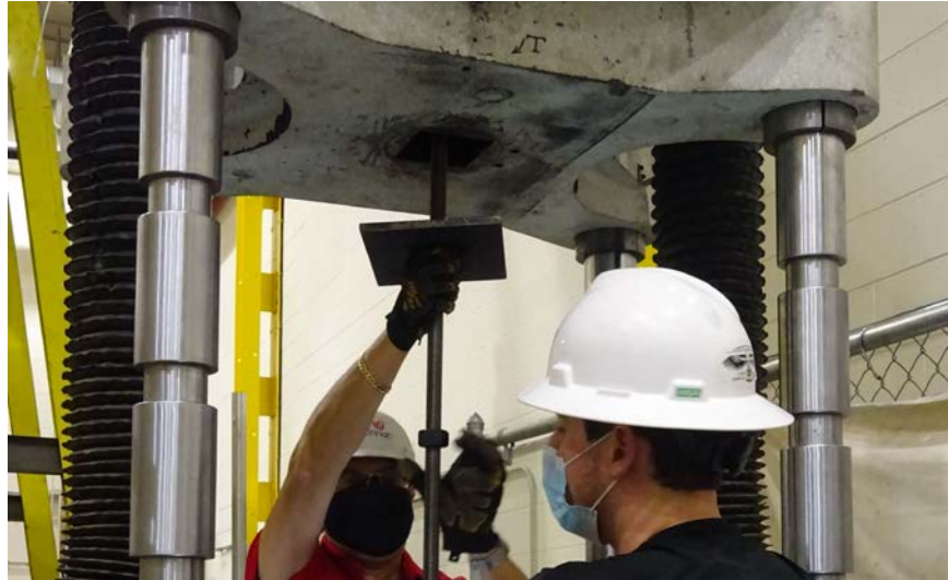
Figure 2.7: Fastening of Safety Plate to Anchor Rod
