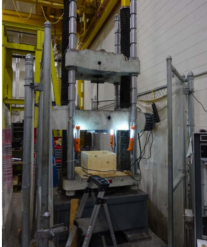
Figure 2.1: Tinius Olsen Super-L Universal Testing Apparatus
