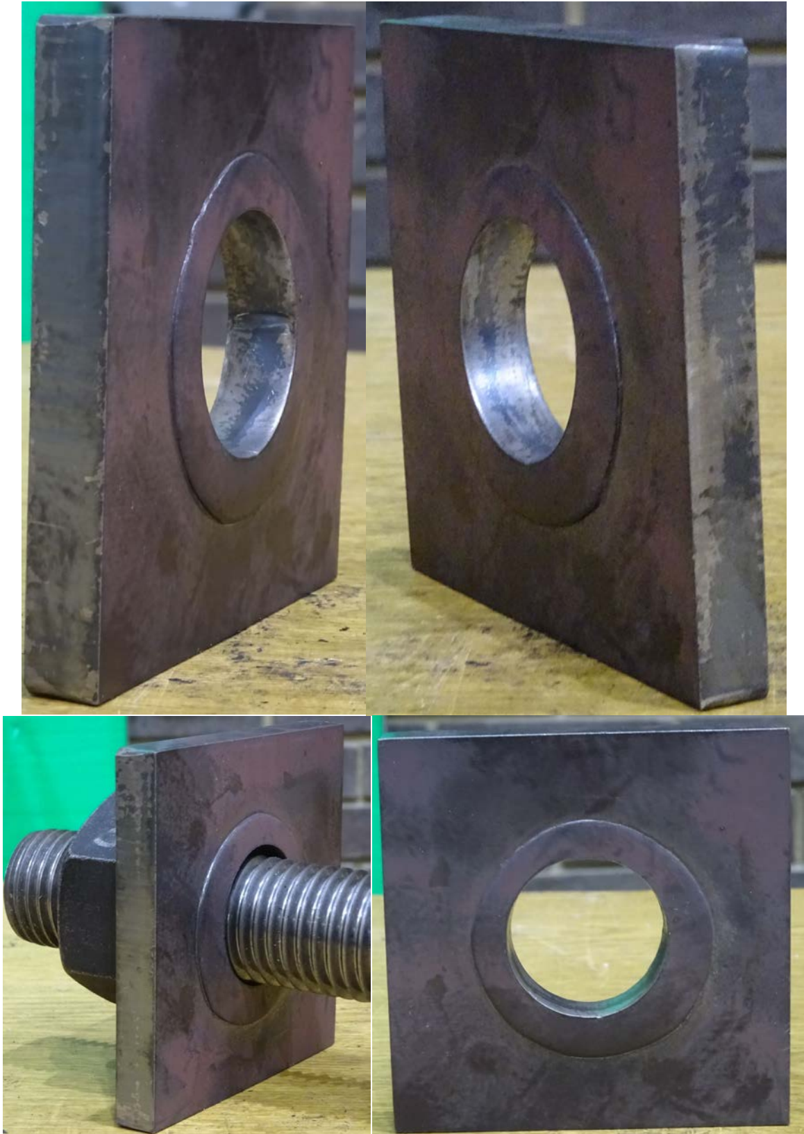
Figure B.56: Test #2A - 14% Relative Deformation
