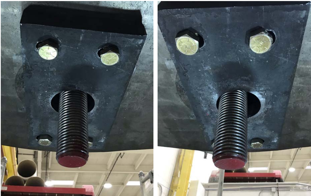
Figure 2.6: Anchor Rod in Centered (left) and Offset (right) Orientations
