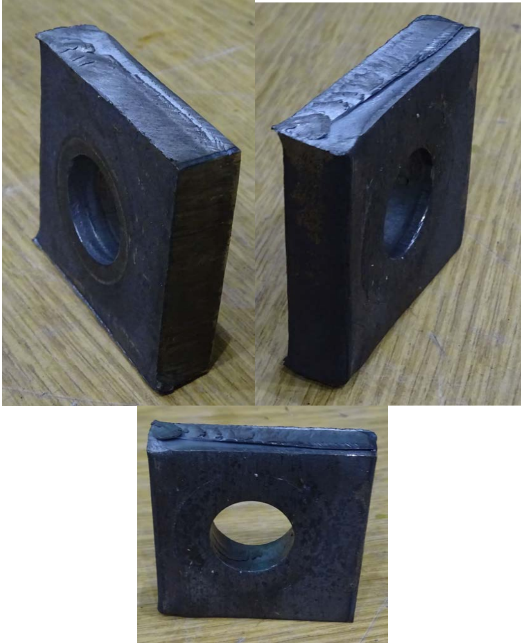
Figure B.14: Test #14 - 9% Relative Deformation
