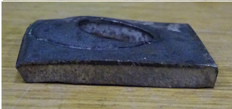
Figure B.18: Test #18 – 68% Relative Deformation
