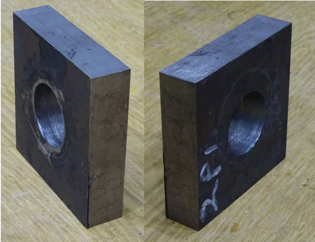
Figure B.49: Test #49 - 2% Relative Deformation
