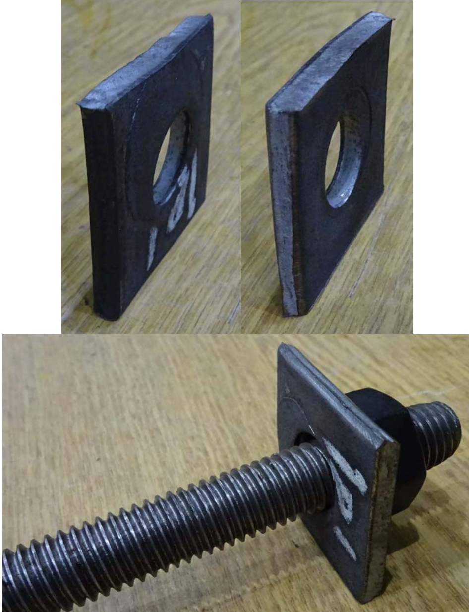
Figure B. 12: Test #12 - 28% Relative Deformation
