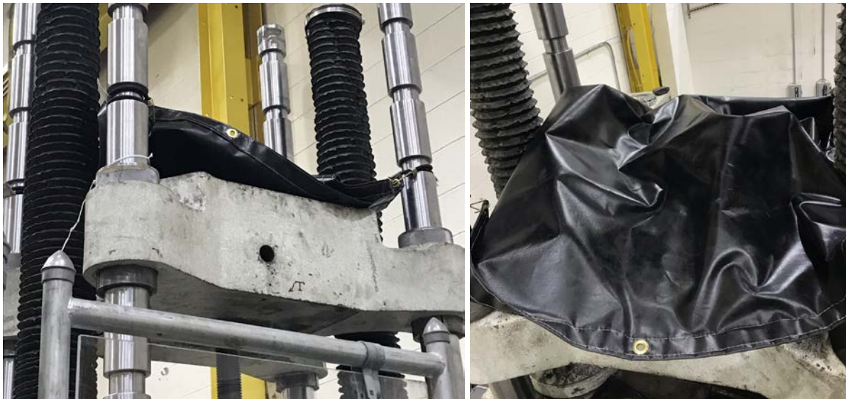
Figure 2.8: Heavy Tarp Affixed to Top Crosshead
