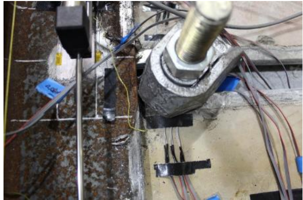
Complete disengagement of Clamp 4
