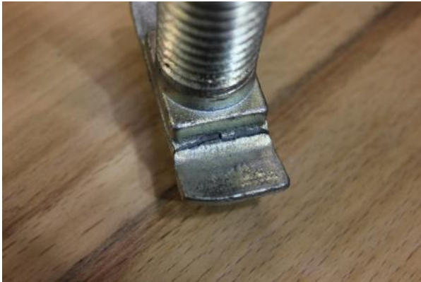
Head fracture in Bolt 4
