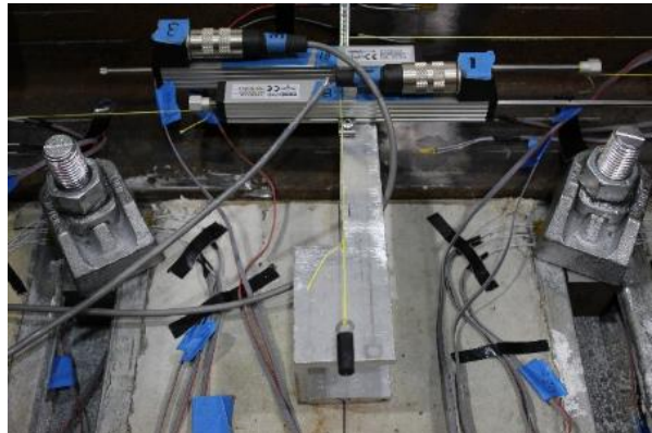
Clamps 1 and 3 rotating in opposite directions
