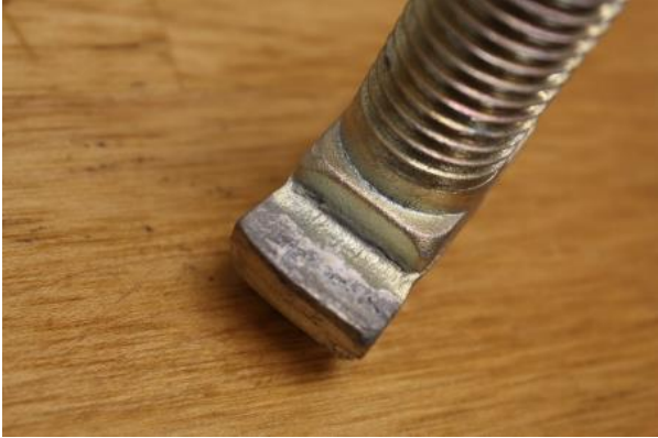
Crack in the bolt head
