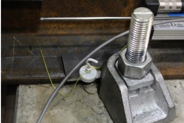
Rotation and slip of shim under Clamp 1
