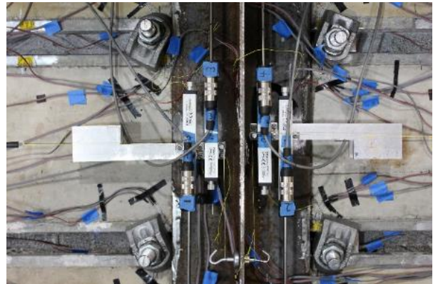
Complete detachment of clamps with beam
