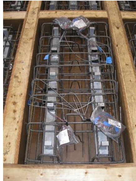
(b) Heavy reinforcement pattern
