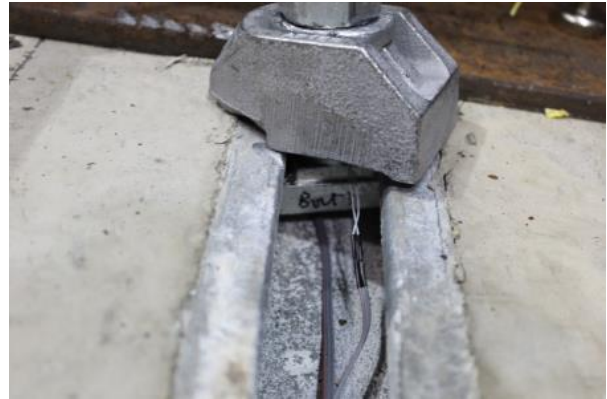
Complete disengagement of Clamp 3
