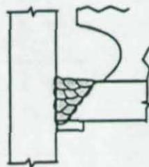
4. Multipass groove weld in moment resisting connection
