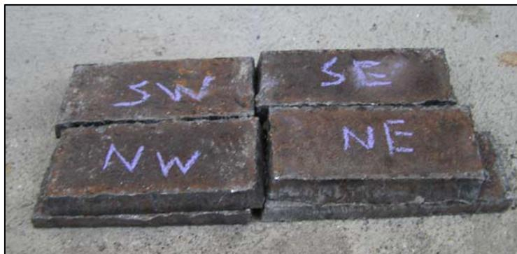
**Figure 3.4** – Steel shim stacks used for friction Tests #1 and #2
