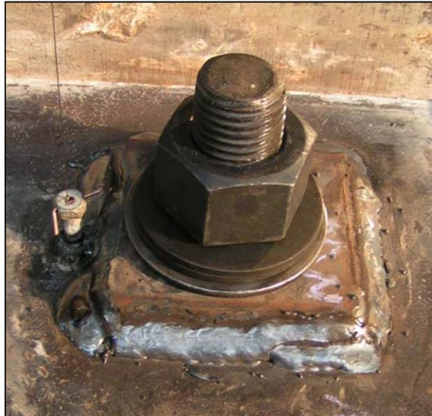
**Figure 3.9** – Welded plate washer detail (shown here for Test #5)
