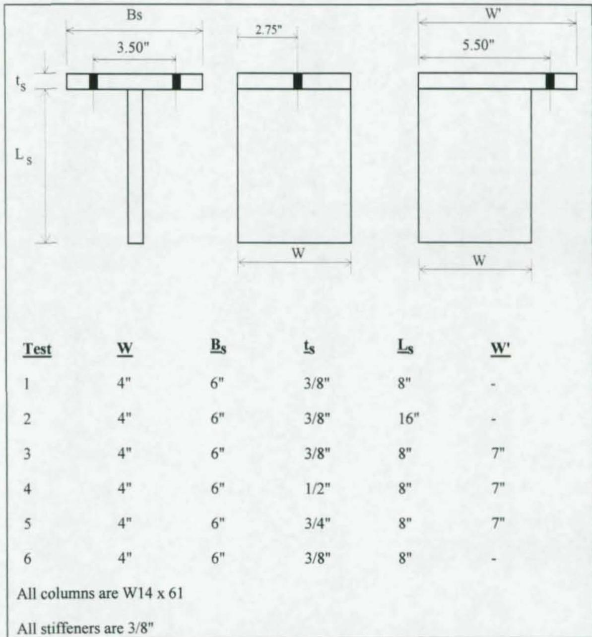
Figure 1. Seat Dimensions for Phase Three
