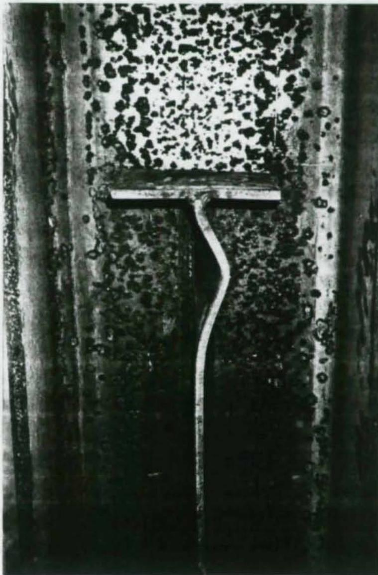
Photograph of Buckled Stiffener--Test Two, Part Two
