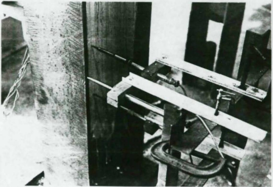
Photograph Showing Three LVDT Arrangement for Part One and Part Two
