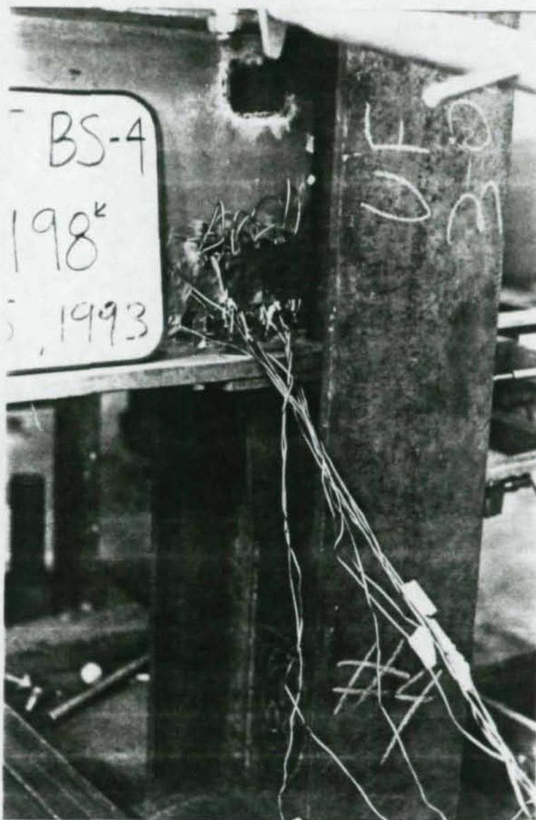
Photograph of Strain Gage Arrangement on Beam Web for Part One
