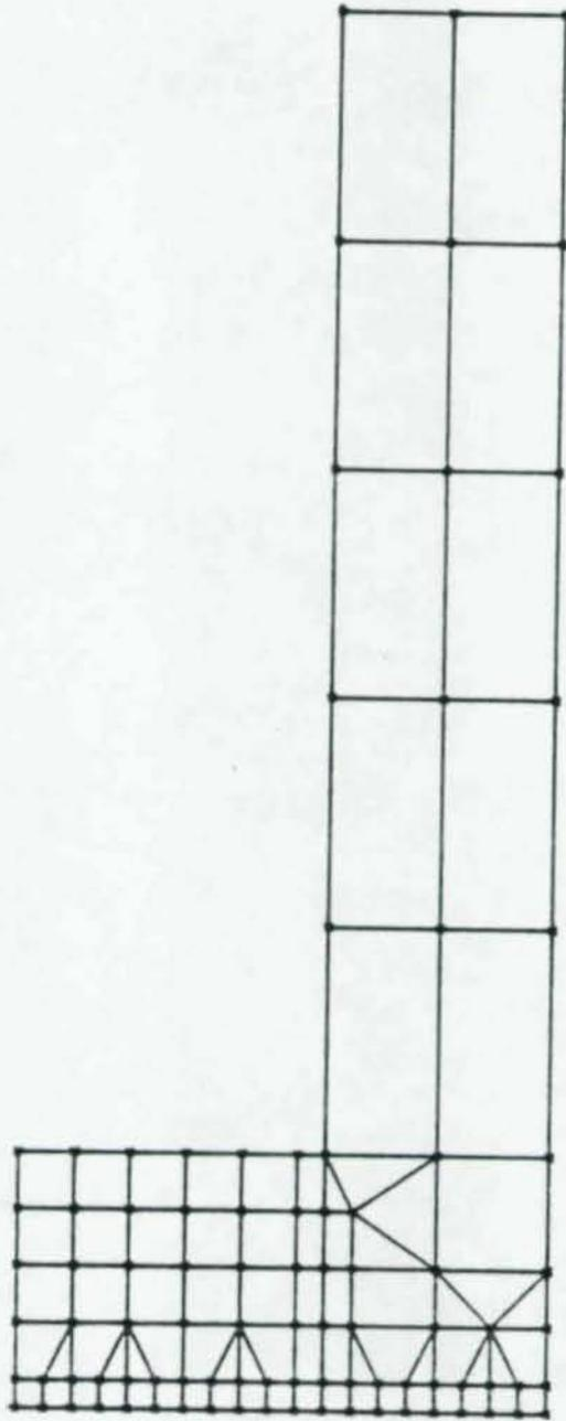
Figure 17. INELAS Finite Element Model of Diagonal Bracing Connection.
