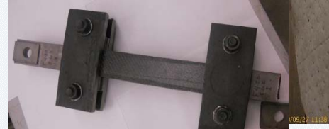
Alemdar, F., Gangel, R., Matamoros, A., Bennett, C., Barrett-Gonzalez, R., Rolfe, S., and Liu, H. (2014). "Use of CFRP Overlays to Repair Fatigue Damage in Steel Plates under Tension Loading," Journal of Composites for Construction , ASCE, 18 (4).
