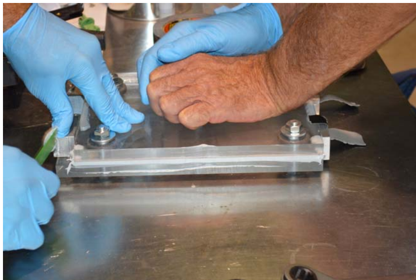
Then seal all the open seals with special sealer.
