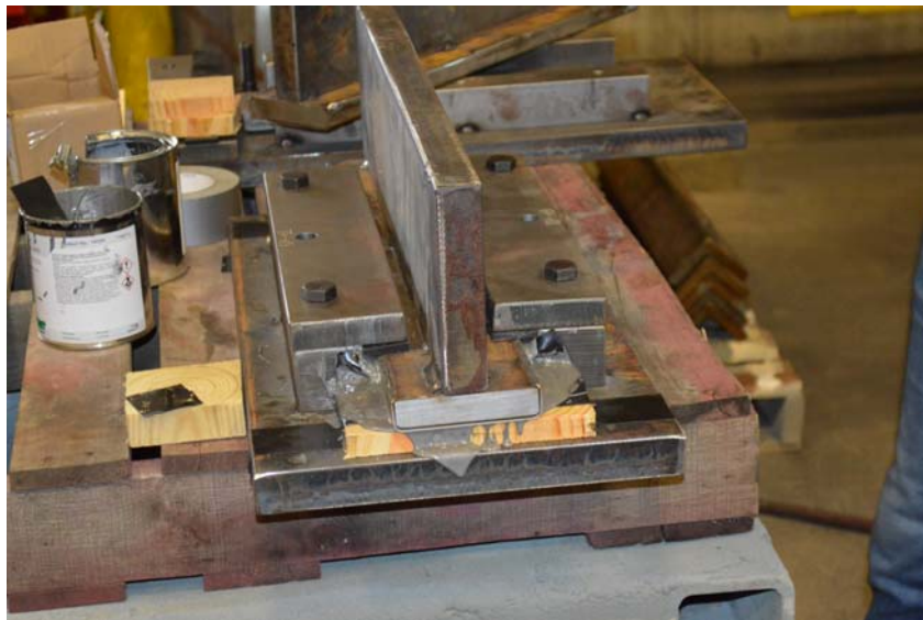
Test - Expansion Joint Used on Gerald Desmond Bridge Long Beach, CA
