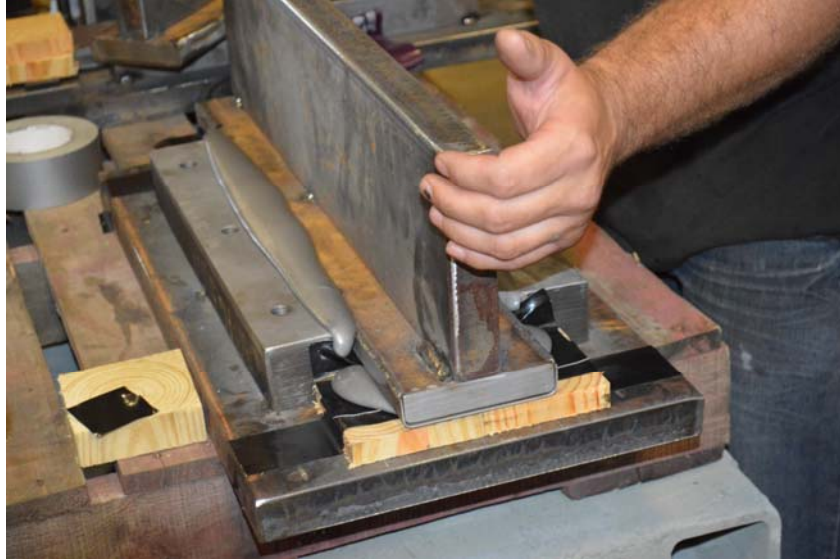
Setting up trial part for expansion joint test - D S Brown
