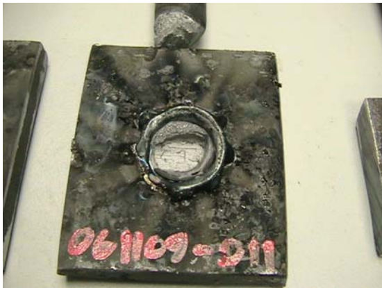
Figure 3. Typical lack of fusion type discontinuity caused by entrapped Zn
