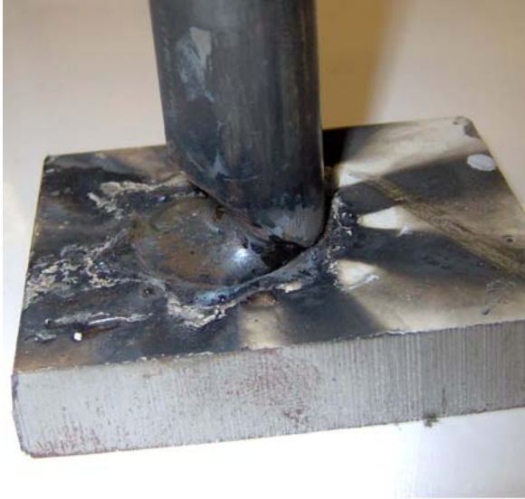
Figure 2. Typical arc blow causing incomplete fusion at the stud/base metal interface. This condition can readily be reproduced by using asymmetrical ground return setup.
