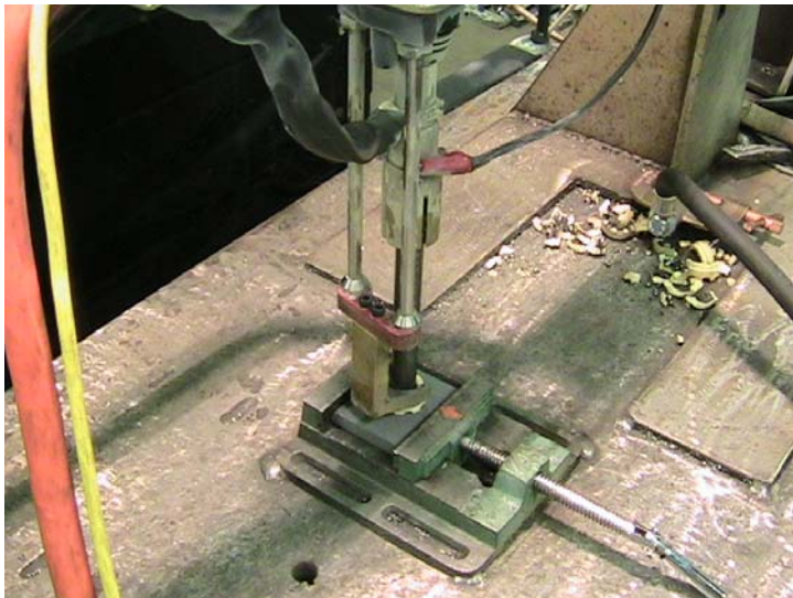
Figure 5b. Setup, latest version. Note the symmetrically grounded vice holding the specimen
