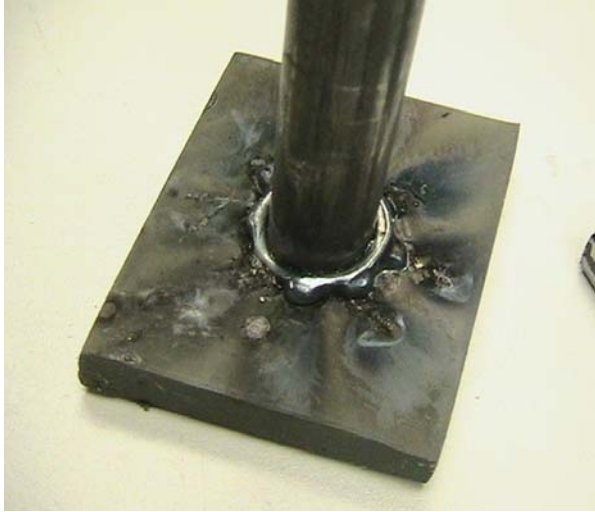
Figure 4. Optimum weld showing full flash and stable parameters (target)
