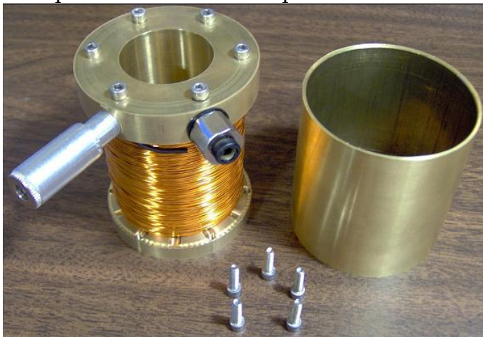
Fig. 13 – Arc Centering Solenoid (ACS) before mounting on the stud welding gun, replacing the support fork/legs.
