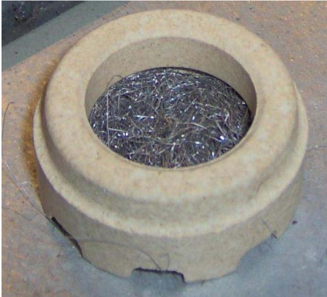
Figure 11. Steel wool packed inside the ferrule before welding
