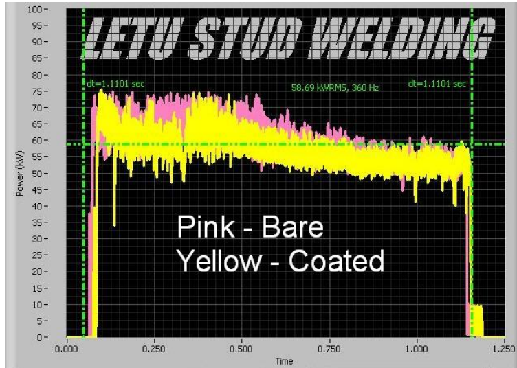
Figure 17. Voltage dropping toward the end of the weld cycle. Also notice no real differences between bare and alkyd paint parameters.
