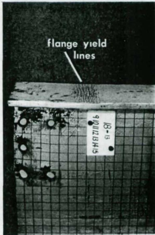
Fig. 3.12 Location of yielding in the compression flange
