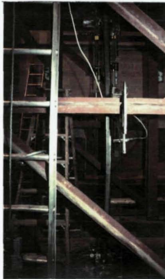
Figure E.6: Buckled Shape Under 10-kip Load - Test 3 - PS
