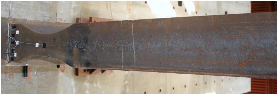
Figure 4.52 Specimen C5: Beam Lateral-Torsional Buckling (End of Test)
