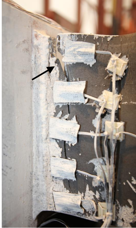
Figure 4.184 Specimen W2: West Beam Bottom Flange Fracture during Excursion to -0.06 rad (2 nd Cycle)
