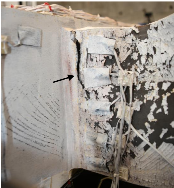
Figure 4.182 Specimen W2: East Beam Top Flange Partial Fracture during Excursion to -0.06 rad (2 nd Cycle)
