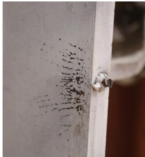
(b) Flange Local Bending
