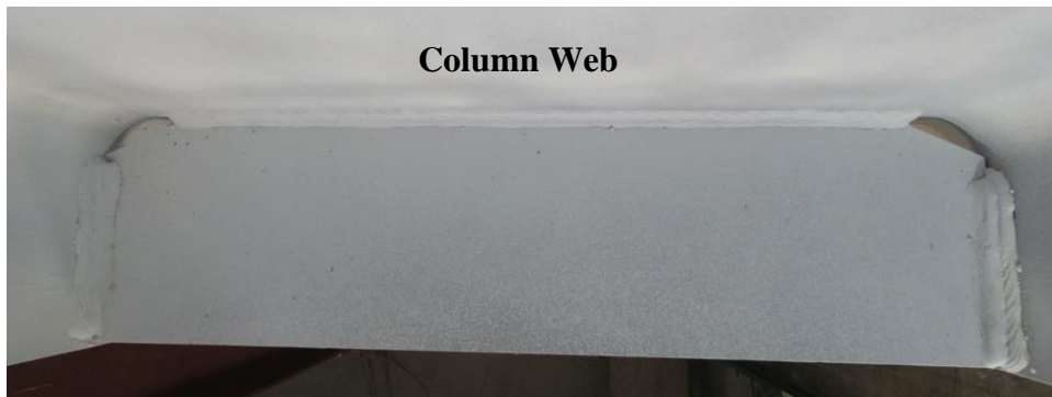
(b) East Top Flange Continuity Plate
