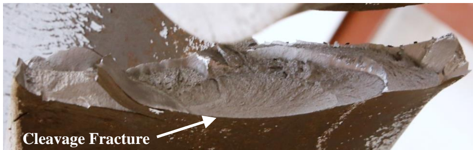
(b) Fracture Surface
