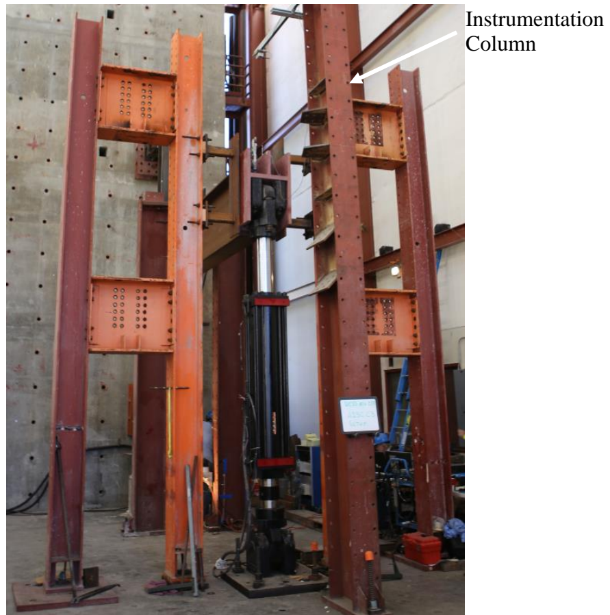
Figure 3.3 Lateral Bracing at Loading End (Phase 1)
