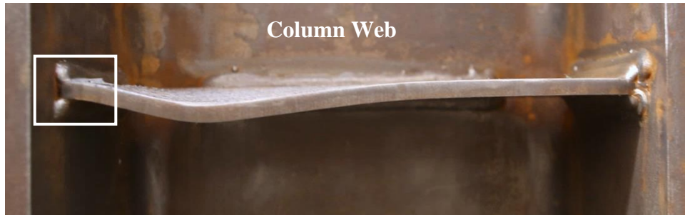
(a) East Bottom Flange Continuity Plate
