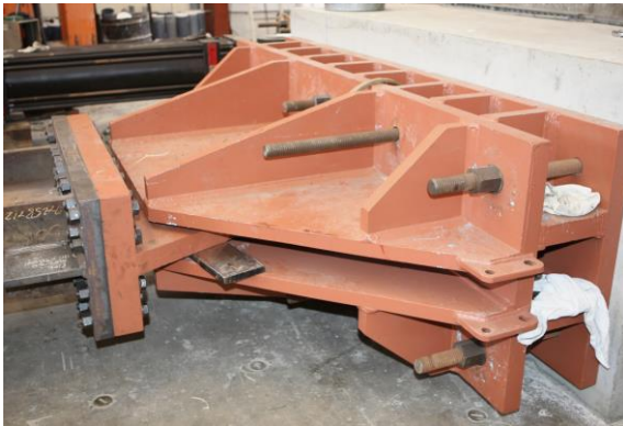
(a) Column Base Support Clevis
