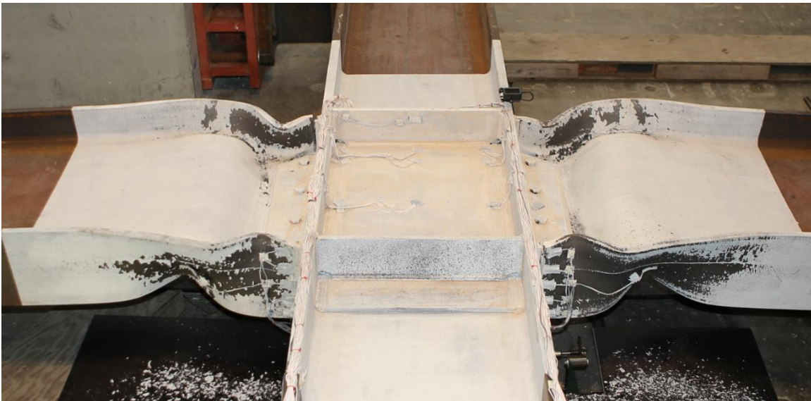
Figure 4.185 Specimen W2: Connection at End of Test
