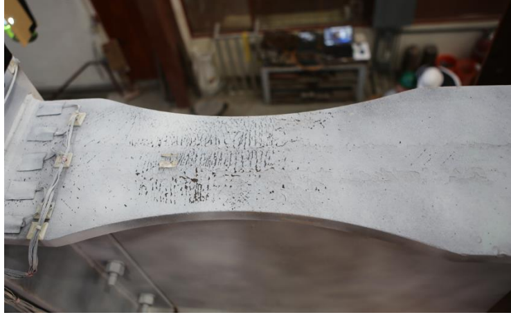
Figure 4.115 Specimen C7: Beam Top Flange Yielding at -0.015 rad (2 nd Cycle)
