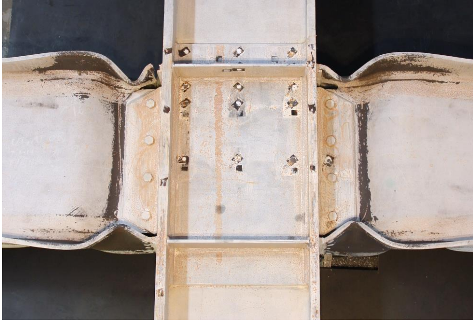
Figure 4.220 Specimen W3: Connection at End of Test
