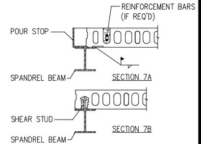
5 PLANK TO SPANDREL CONNECTION
