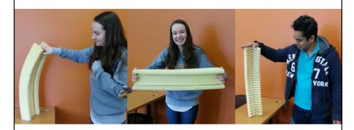
Instructions include dimensions for a channel, angle, and "W-shape". The "W-shape" can be used to demonstrate lateral torsional buckling.
