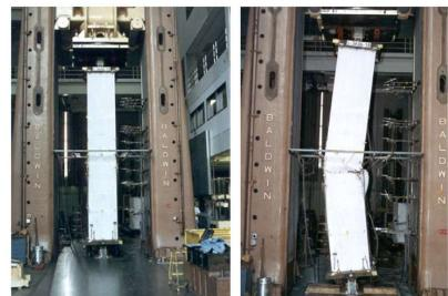
Wait! Which came first, local buckling or flexural buckling?
