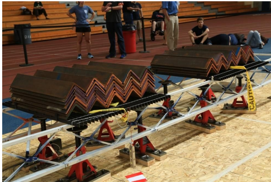
Vertical load station
