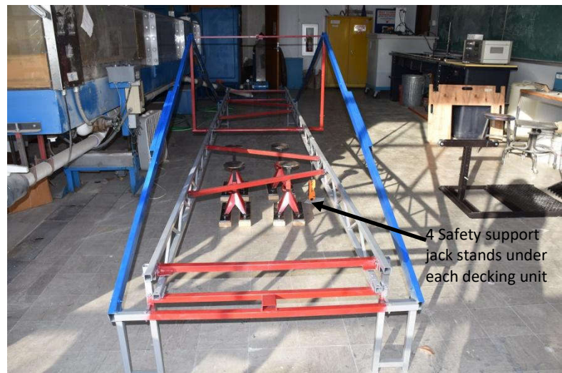
Figure 2. Jack stands under bridge at load location.
