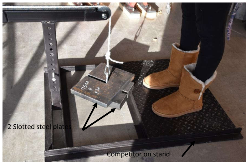
Figure 8. Load applied to lateral load stand.
