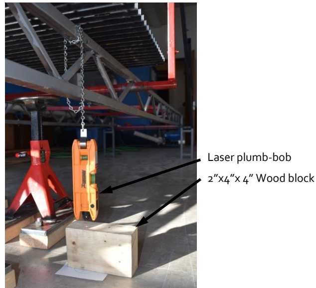
Figure 9. Laser plumb-bob position.
