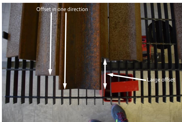
Figure 15b. Improper stacking of loading angles.
