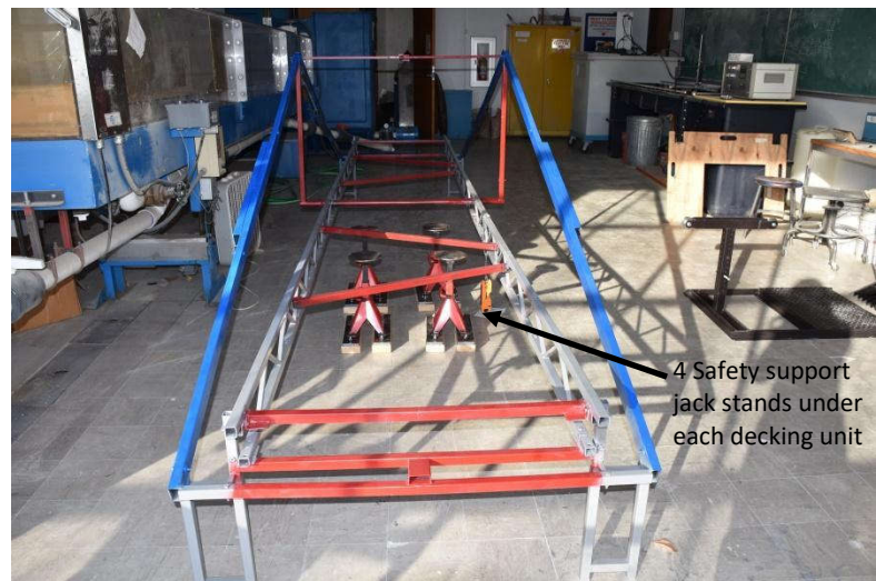
Figure 2. Jack stands under bridge at load location.
