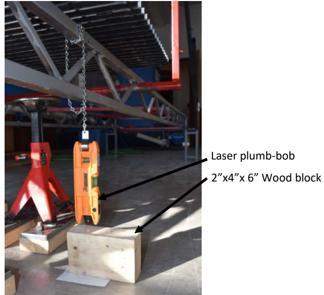
Figure 9. Laser plumb-bob position.
