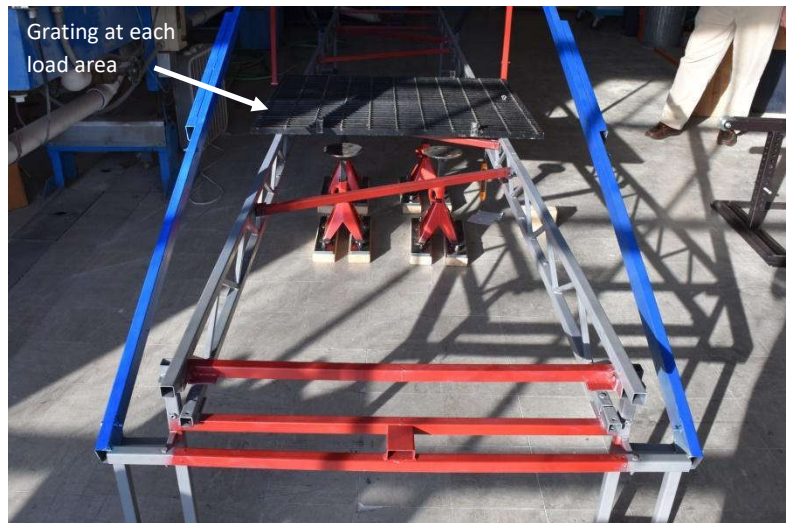
Figure 4. Grating in position.
