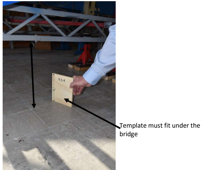
Figure 1. Plywood template for ground clearance.
