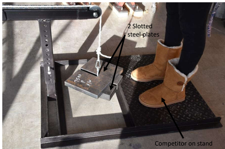
Figure 8. Load applied to lateral load stand.
