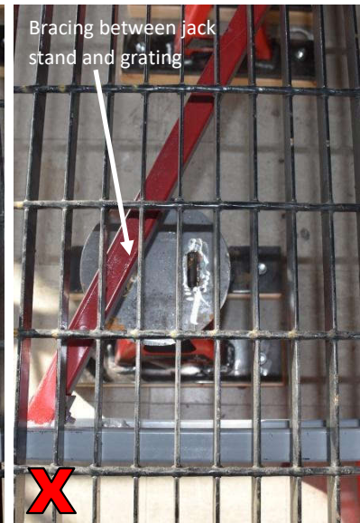
Figure 6b. Incorrect position.
