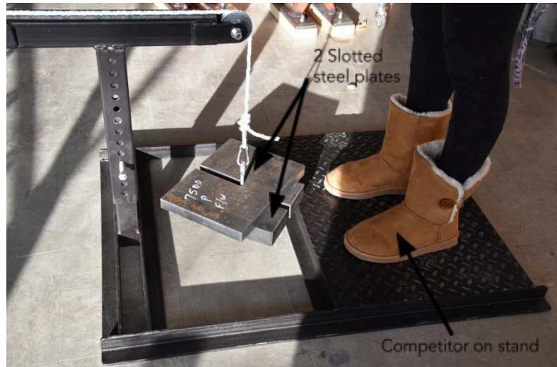
Figure 8. Load applied to lateral load stand.
