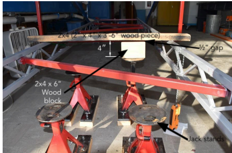
Figure 3. Jack stand height adjustment.
