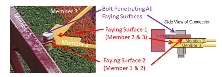
**Example 4(a) and 4(b):** <u>Prohibited connections</u> where all contact points are not treated as faying surfaces as specified in 9.4.2.1. Since any point of contact between members creates a faying surface, these points of contact need to be penetrated by at least one loose bolt secured by a loose nut. There are also more than 2 faying surfaces associated with each member being connected (9.4.2).
