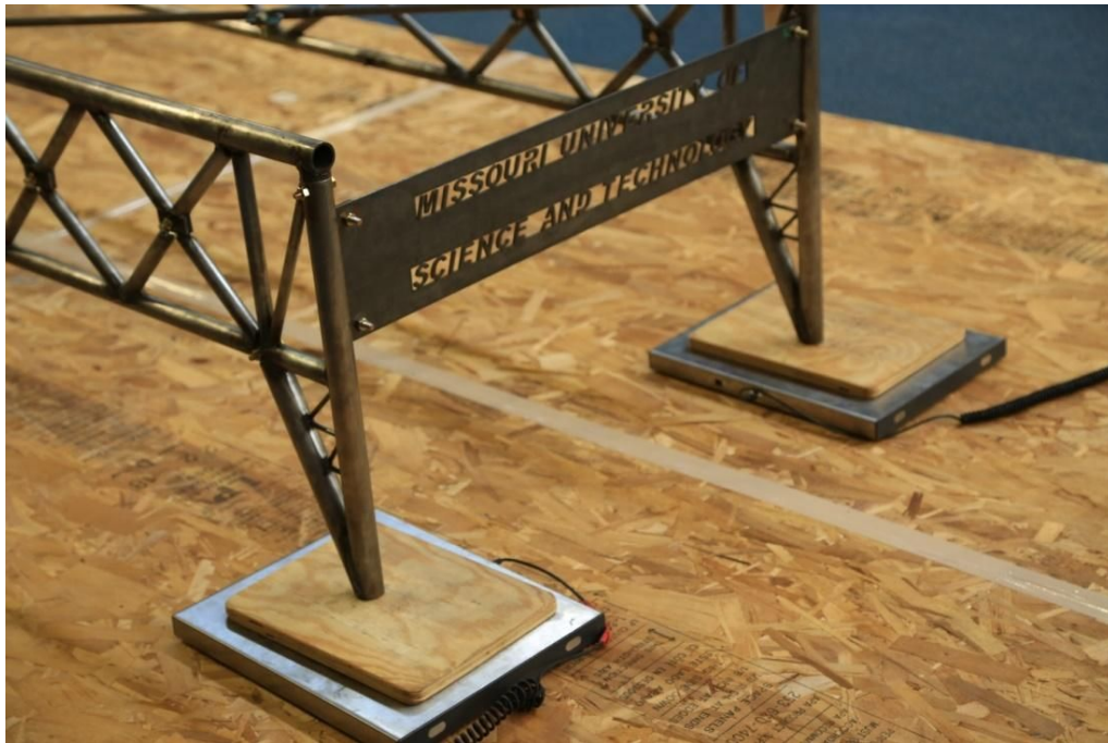
Bridge on the scales to measure weight
