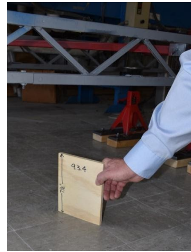
Plywood templates for passageway and ground clearance checks
