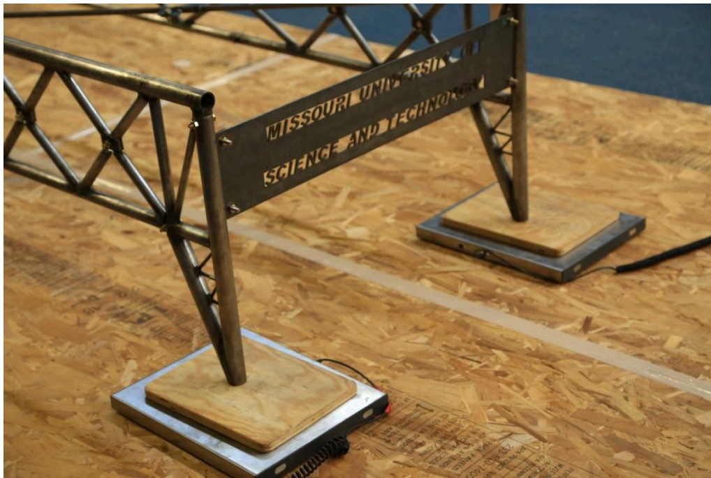
Bridge positioned on scales to measure weight
