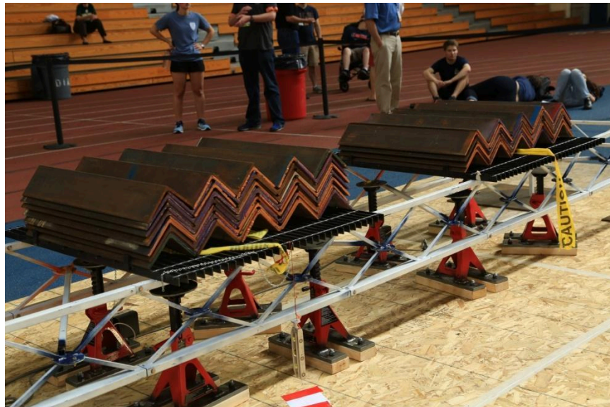
Vertical load station with safety supports, grating, and loading angles
