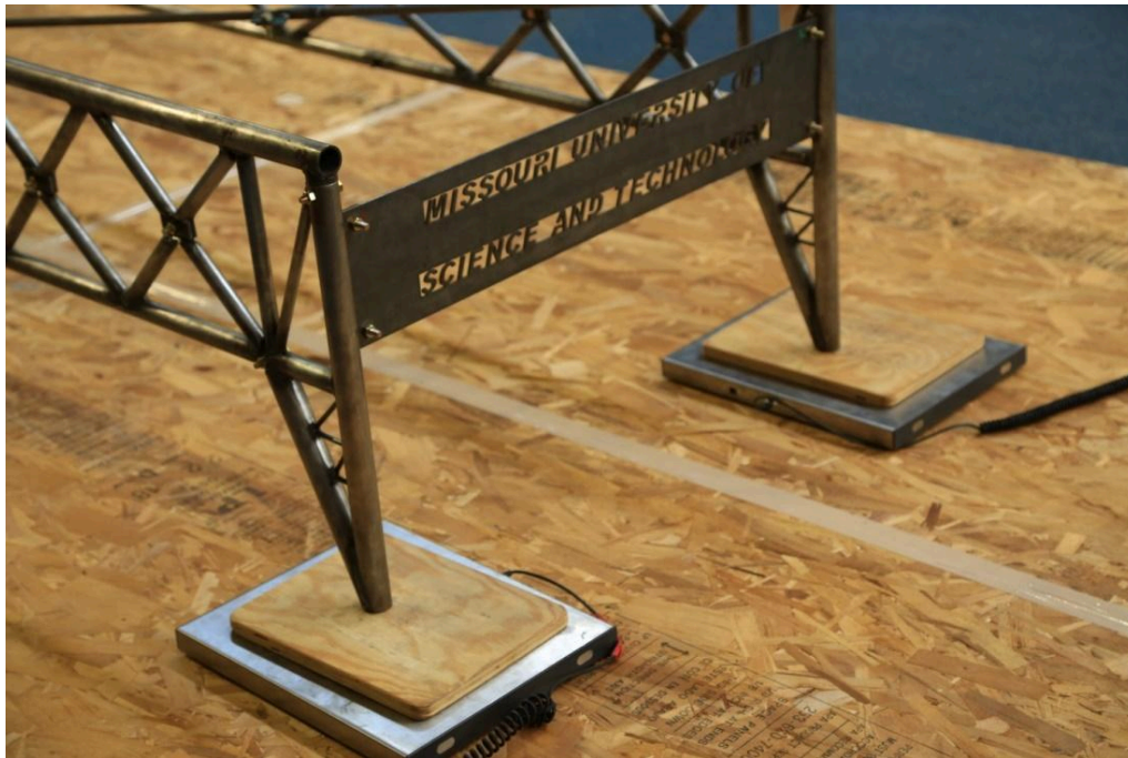
Bridge positioned on scales to measure weight
