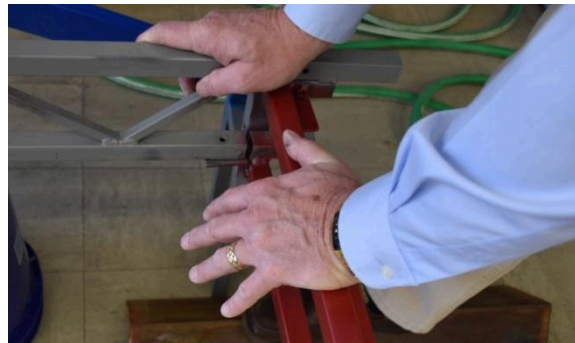
Pushing down on bridge is not permitted
