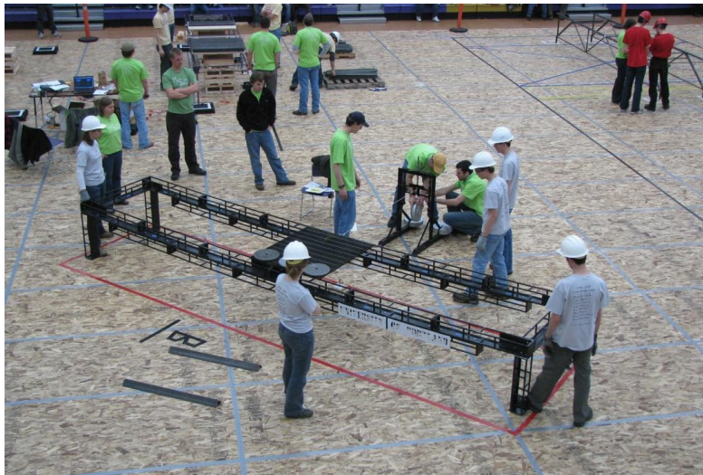
Lateral load test station
