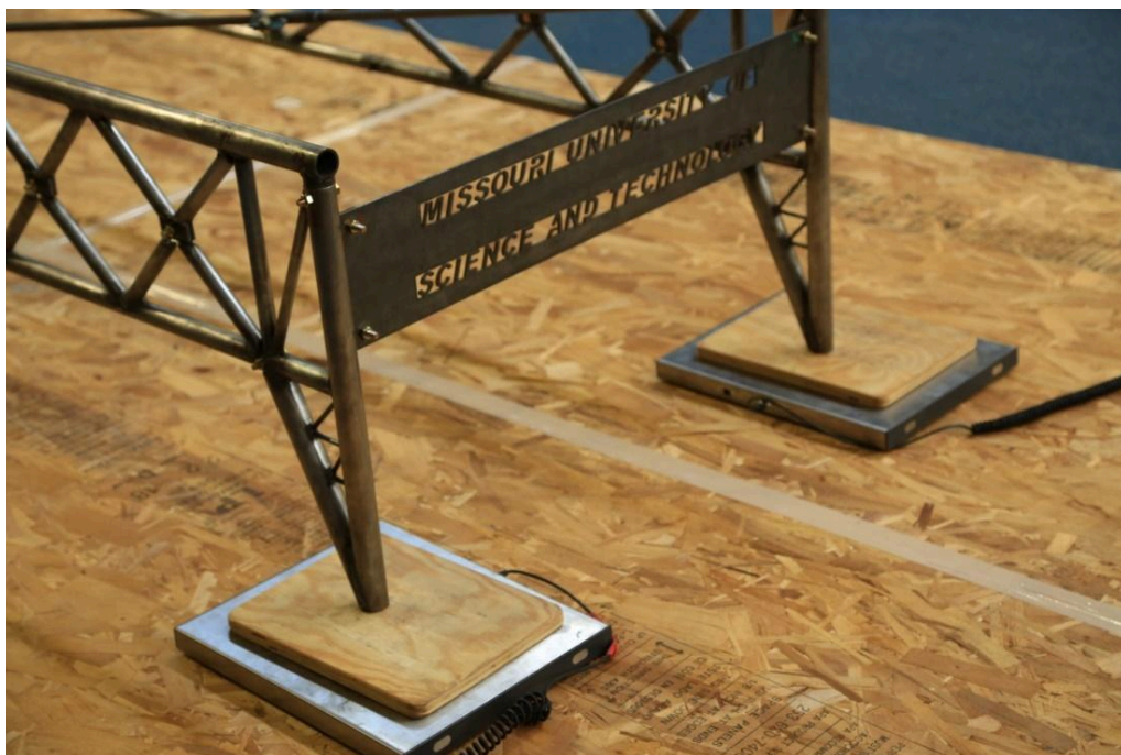
Bridge positioned on scales to measure weight
