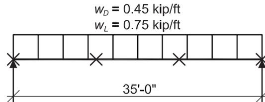
*Beam Loading & Bracing Diagram
