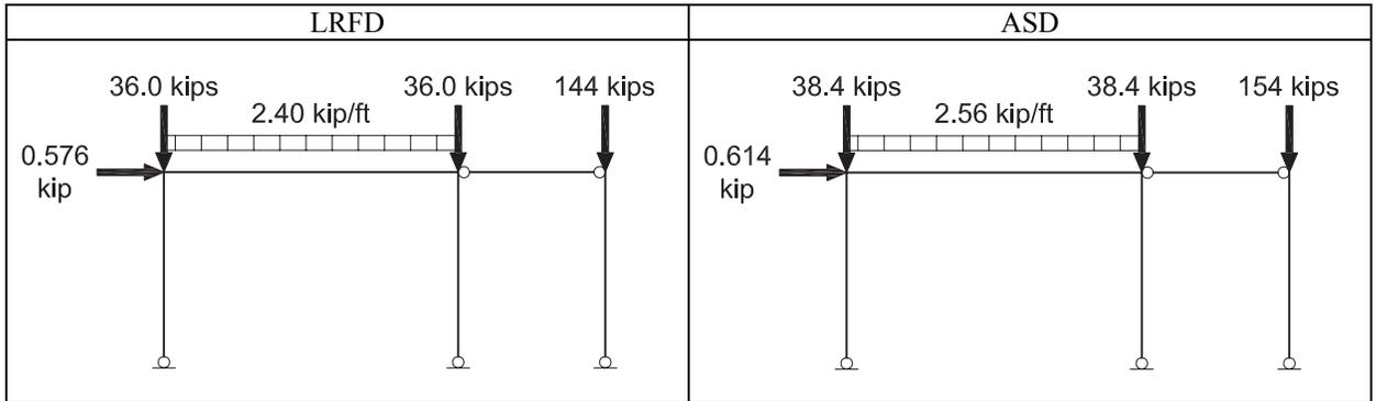
Per AISC Specification Appendix 7, Section 7.2.2, conduct the analysis using the full nominal stiffnesses.
