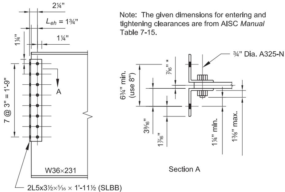
\* This dimension (see sketch, Section A) is determined as one-half of the decimal web thickness rounded to the next higher 1/16 in. Example:  $0.760/2 = 0.380$ "; use 7/16 in. This will produce spacing of holes in the supporting beam slightly larger than detailed in the angles to permit spreading of angles (angles can be spread but not closed) at time of erection to supporting member. Alternatively, consider using horizontal short slots in the support legs of the angles.
