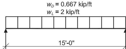
*Beam Loading & Bracing Diagram*
