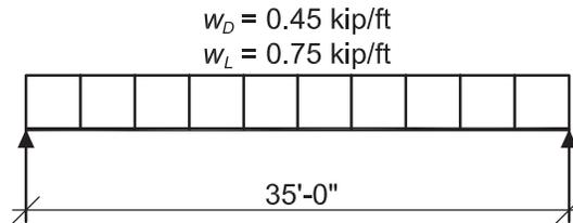
*Beam Loading & Bracing Diagram
