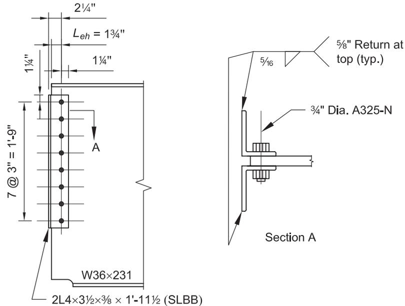
Note: Bottom flange coped for erection.
