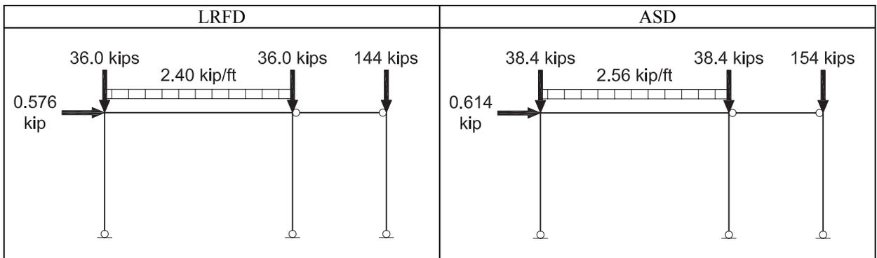
Per AISC *Specification* Section C2.3, conduct the analysis using 80% of the nominal stiffnesses to account for the effects of inelasticity. Assume, subject to verification, that  $\alpha P_r/P_y$  is no greater than 0.5; therefore, no additional stiffness reduction is required.
