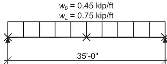
*Beam Loading & Bracing Diagram
