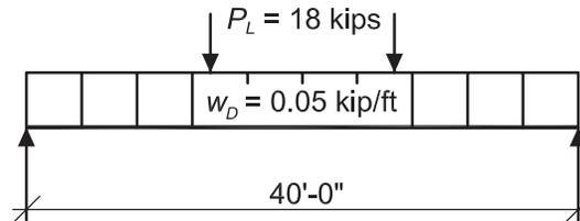
Beam Loading & Bracing Diagram
