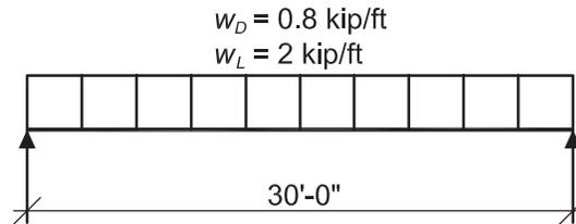
Beam Loading & Bracing Diagram
