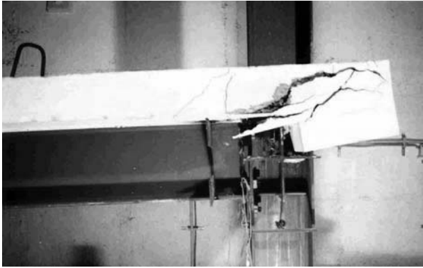
Figure 10 - Hysteresis loops and failure mode of an external node with a steel column.
