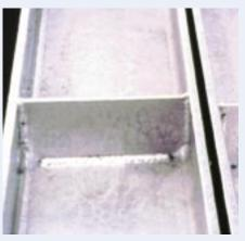
Cropped corners allow molten zinc to flow in and out of tight spaces, avoiding "pooling" in these areas causing excessively thick coatings that may flake during rough handling.
