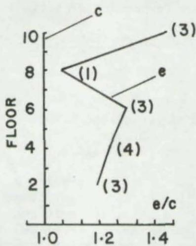
(f) MAX. RATIOS OF AXIAL FORCES,  $e/c$ , OF BRACINGS, ( ),  $c=N-S$ ,  $P-\Delta(DL)$ ;  $e=N-S$ ,  $E-W$ ,  $VE$ ,  $P-\Delta(DL+VE)$  FOR (I)
