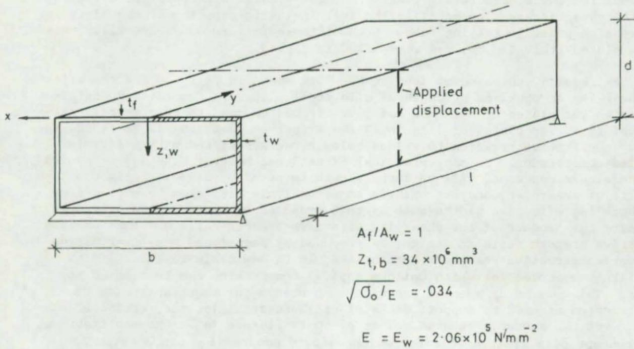
Fig 1 Cross section used for parametric study (webs remain elastic)
