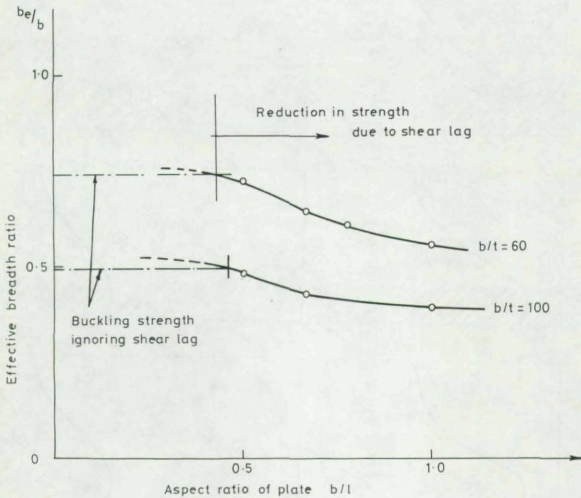
Fig 4 Effect of shear lag on buckling strength of mild steel plates in compression.
