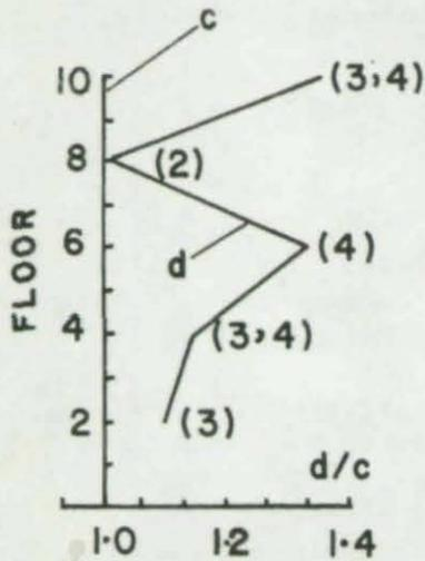
(e) MAX. RATIOS OF AXIAL FORCES,  $d/c$ , OF BRACINGS, ( ),  $c=N-S$ ,  $P-\Delta(DL)$ :  $d=N-S$ ,  $E-W$ ,  $P-\Delta(DL)$  FOR (I)
