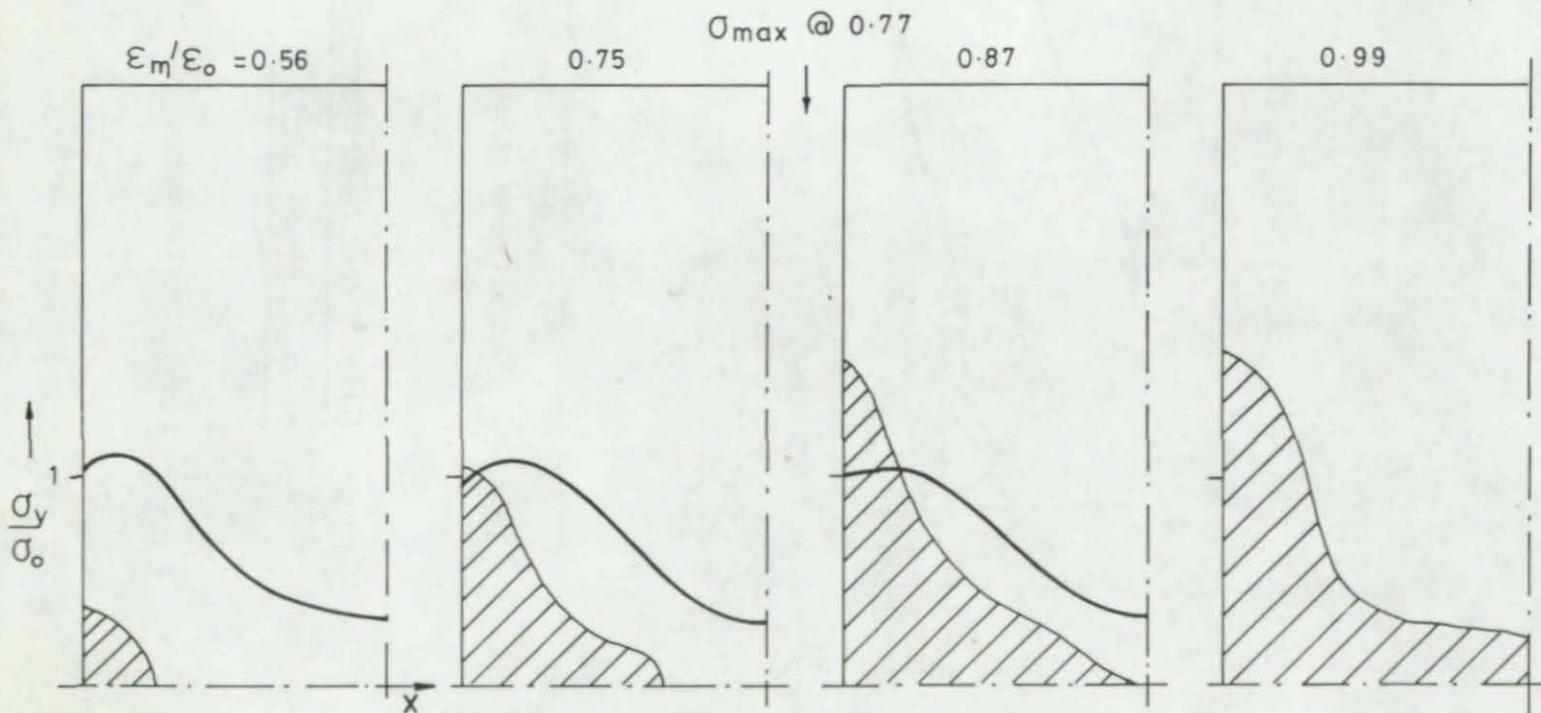
CASE 2. LONGER PLATE  $b/l = 0.5$ ;  $b/t = 60$ ;  $\omega_0 = b/200$
