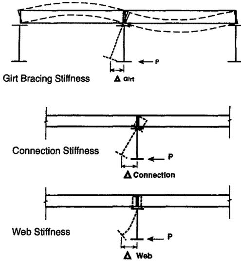
Figure 4 - Sources of Flexibility in Bracing Load Path
