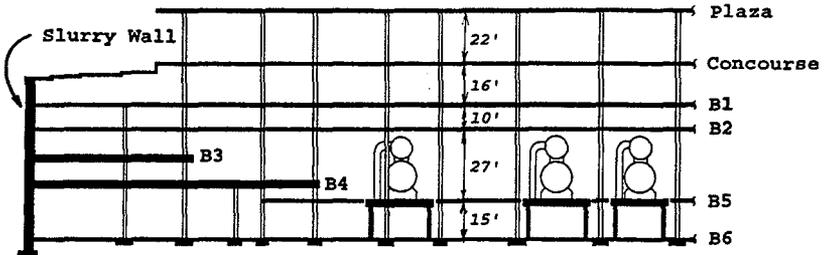
FIGURE 2: Section through sub-grade levels at the site of the explosion
