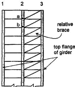
Fig. 4 Relative Bracing
