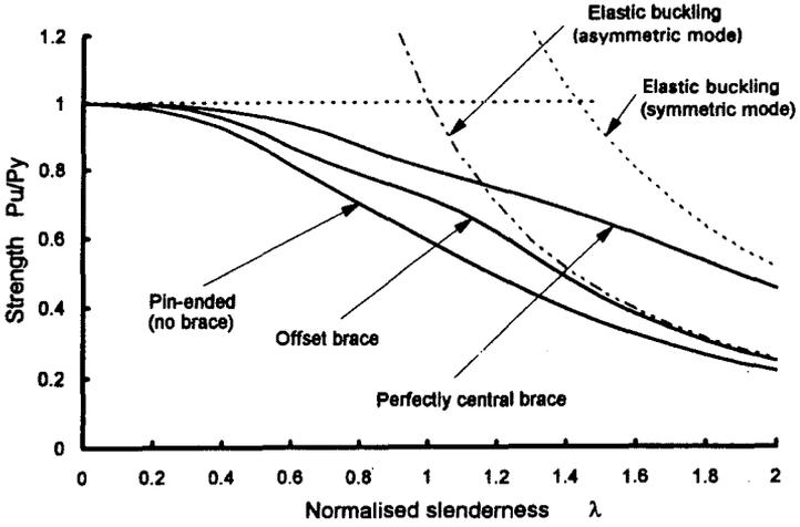
Fig. 2 Column curves for compression members with and without a central brace
