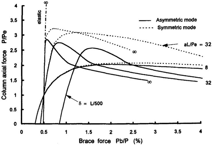
Fig. 7 Variation of bracing force with applied axial force, inelastic behaviour,  $\lambda = 1$
