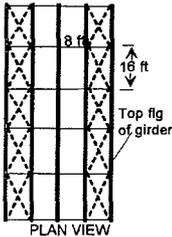
Same as Example 1 except the bracing system is a relative system - a top flange horizontal truss. Each truss stabilizes 2-1/2 girders. The unbraced length of the girder flange is 16 ft which was checked in Example 1.
