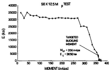
Figure 6: E vs. M :  $M_p$  TEST
