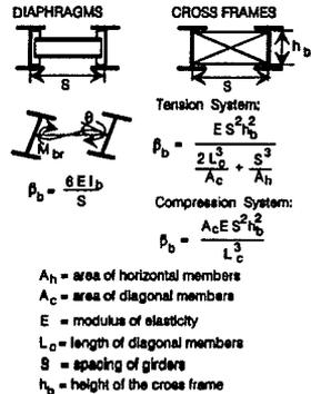
Figure 1 Diaphragm and cross frame stiffness
