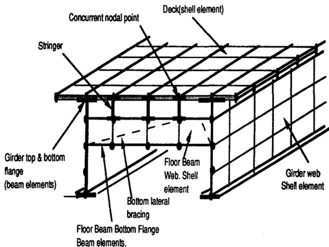
Figure 4. Three Dimensional Model
