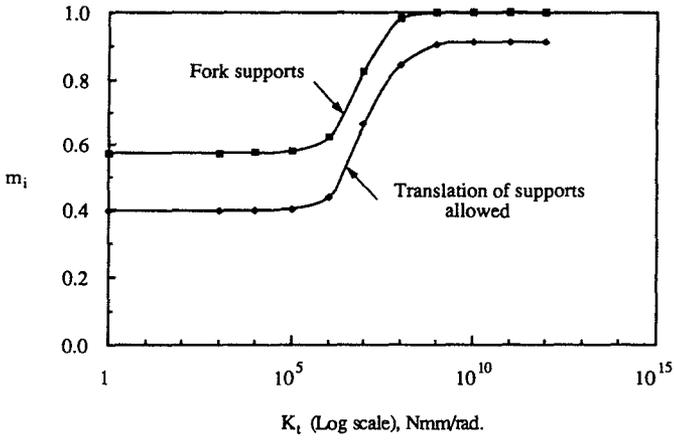
Fig. 3 Effect of torsional restraint stiffness
