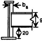
Note: The portion of the web along the depth of the diaphragm can be treated as rigid. Then use Equation 5 to get stiffness of web above and below the diaphragm ( $h_c = h_t = 20$  in)
