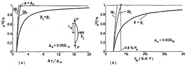
Fig. 2 Braced Column with Initial Out-of-Straightness
