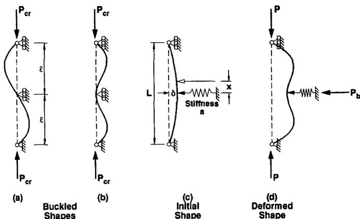
Fig. 1 Pin-ended column with central brace
