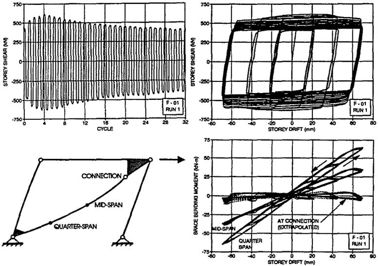
Fig. 8. Full scale braced frame: a) storey shear to storey drift relationship, b) bending moments in the bracing member.
