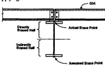
Figure 6 - Directly Braced and Indirectly Braced Column Halves
