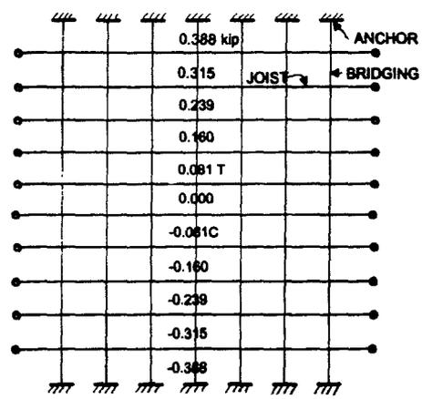
Fig.4 Bracing forces in center row of bridging
