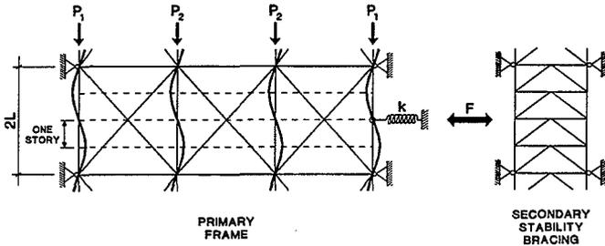
**Fig. 6** Secondary Bracing System Design Concept
