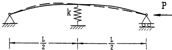
Fig. 3. Deflection before buckling (solid) and after (dashed);  $a_1=L/2, k>k_{id}$
