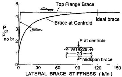
Fig. 7 Midspan Load at Centroid
