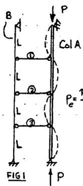
Col A is supported by member B. What  $I_b$  is req'd for full bracing?
