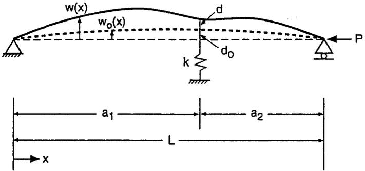
Fig. 2. Imperfect column before loading (dashed) and after loading (solid)
