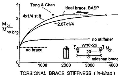
Fig. 14 Torsional Brace at Midspan
