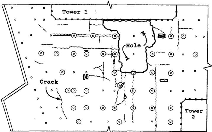
FIGURE 5: Damage at the B1 level
