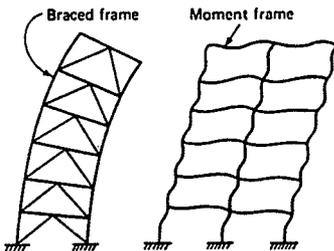
Fig. 8a BRACED FRAME AND MOMENT FRAME DEFLECTION CHARACTERISTICS
