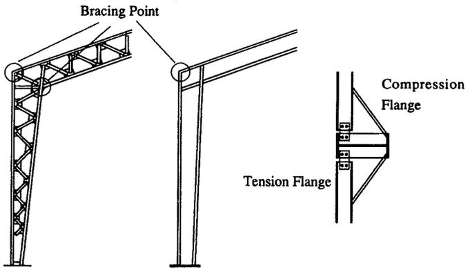
Fig.11 Bracing Point
