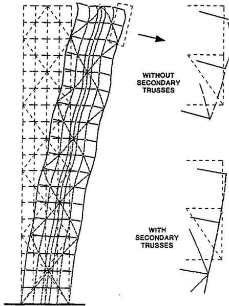
**Fig. 16 Behavior Under Wind Load**
