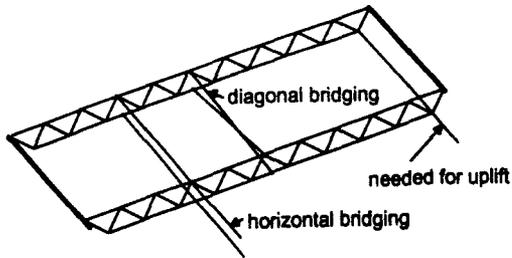
Fig.1 Types of lateral bracing
