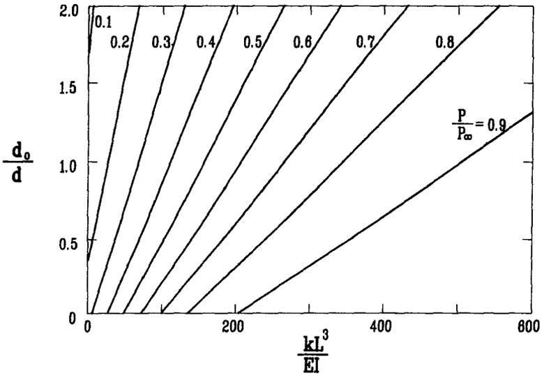
Fig. 4. Effect of bracing stiffness on deflection ratio;  $a_1=0.6L$ , parabolic  $w_0$ .
