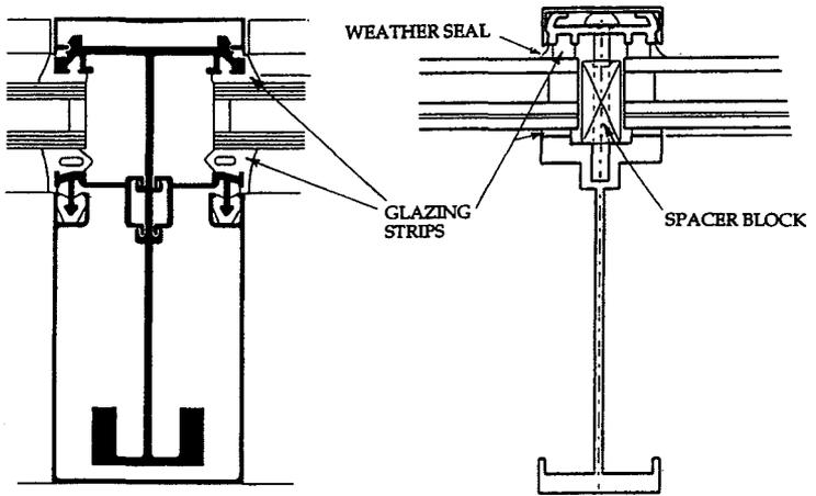
FIGURE 3 - GLASS CLAMPED IN PLACE
