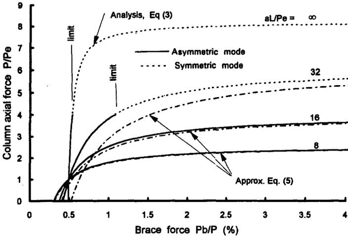
Fig. 6 Variation of bracing force with applied axial force, elastic behaviour,  $\lambda = 1$
