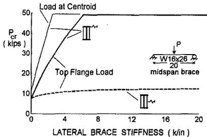
Fig. 8 Effect of Load and Brace Position
