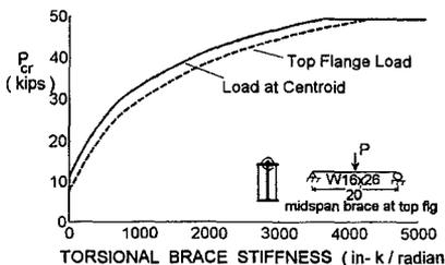
Fig. 17 Effect of Load Position
