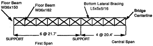
Figure 2. Floor Beams & Bottom Lateral Bracing
