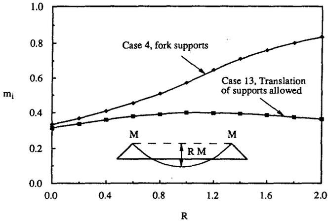
Fig. 4 Variation of inelastic moment resistance ratio with static moment ratio
