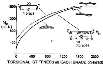
Fig. 18 Multiple Torsional Braces
