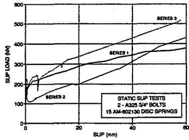
Fig. 2. Static slip tests: a) sample, b) typical response.
