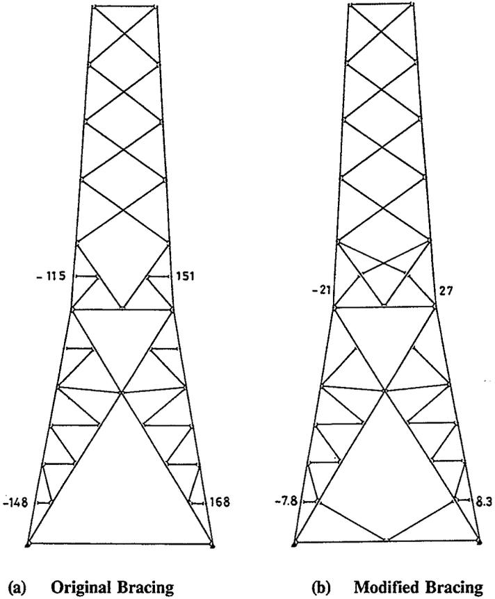
**Fig. (2) A Two-Dimensional Partial Model of the Tower showing Maximum Moments (kN-mm)**
