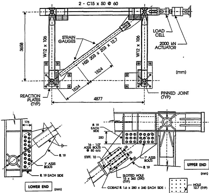
Fig. 6. Full scale braced frame testing: details.
