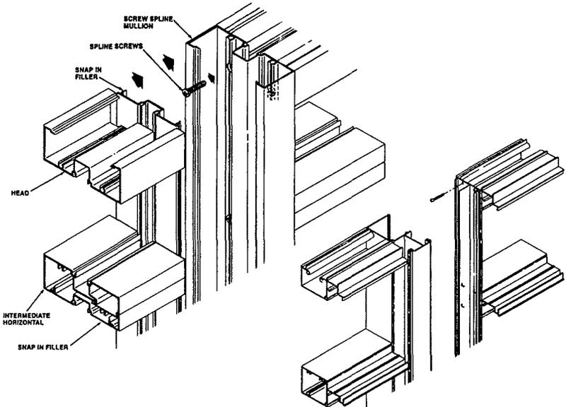
FIGURE 6 - HORIZONTAL MEMBERS ROTATIONALLY WELL ATTACHED
