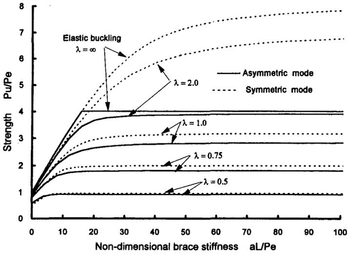
Fig.4 Ultimate strength of columns of  $\lambda = 1$  with central brace of varying stiffness  $aL/P_e$
