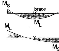
Fig. 13 Double Curvature
