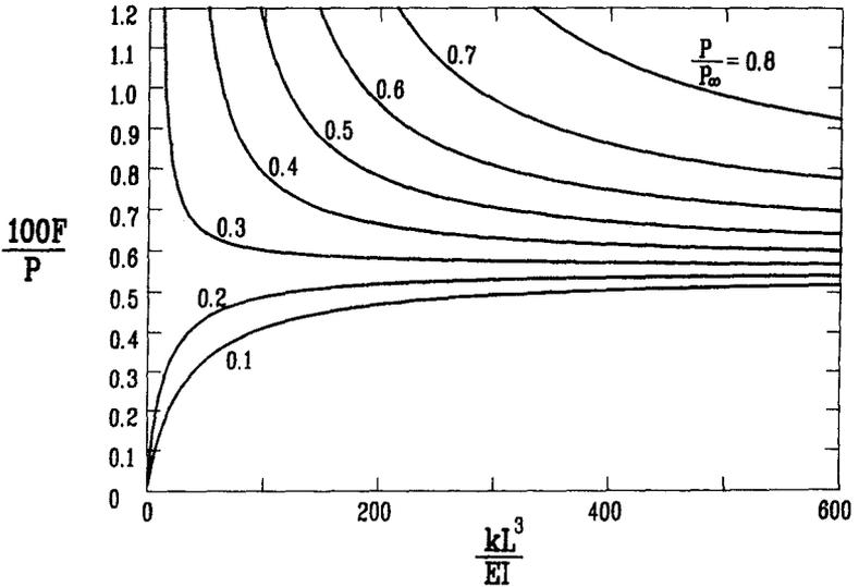
Fig. 5. Effect of bracing stiffness on bracing force;  $a_1=0.6L$ , parabolic  $w_0$ ,  $d_0=L/1000$
