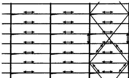
Figure 3 - Bracing Forces in Roof Bracing
