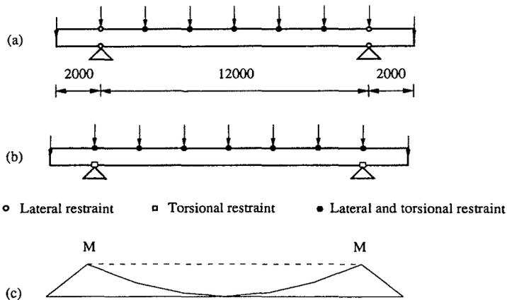
Fig. 2 Restraint and loading conditions. (a) Fork supports
