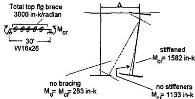
Fig. 16 Effect of Cross Section Distortion
