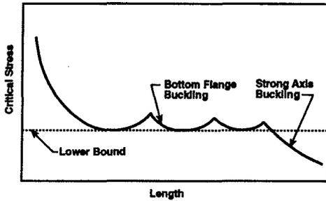
Figure 7 - Strut Purlin Ultimate Stress
