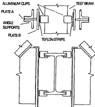
Figure 9: LOAD POINT BRACE
