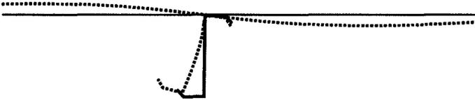
Figure 8 - Lateral Flange Buckling
