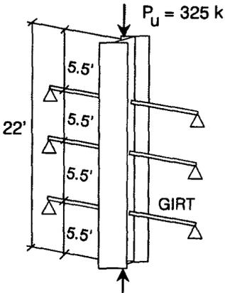
WHAT GIRT STIFFNESS IS NECESSARY TO ADEQUATELY BRACE THE COLUMN?
