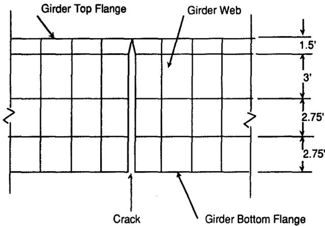
Figure 5. Modeling of the crack
