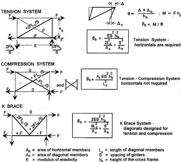
Fig. 21 Stiffness Formulas for Cross Frames
