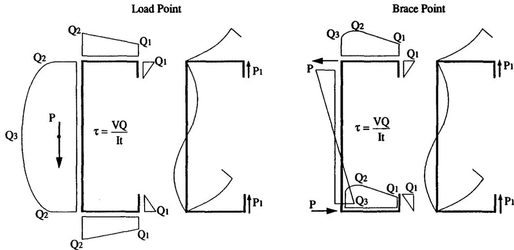
**Distortion at Load and Brace Points**
