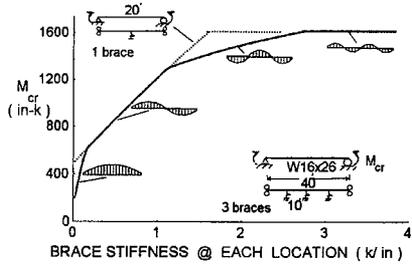
Fig. 11 Multiple Lateral Bracing
