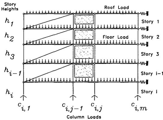
FIG. 2. Frame Bracing Design Parameters
