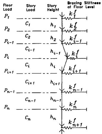
FIG. 4. Frame Model with External Bracing
