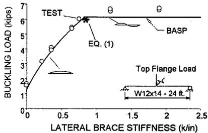
Fig. 12 Lateral Bracing Tests
