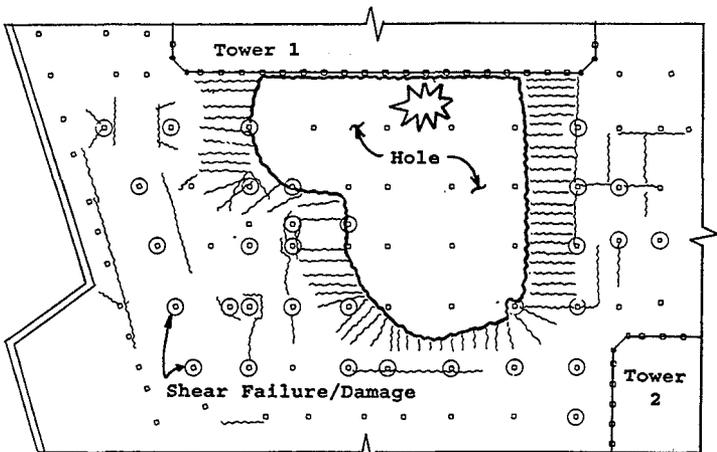
FIGURE 6: Damage at the B2 level
