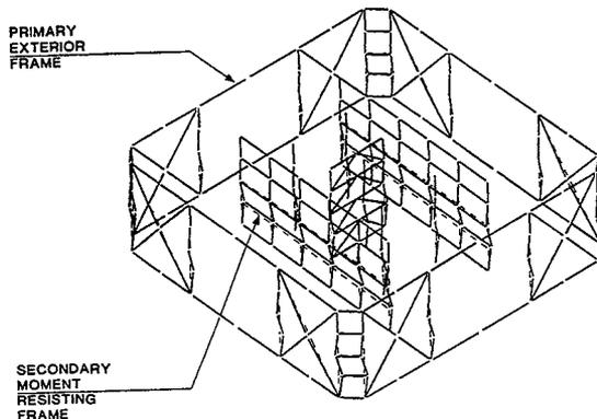
**Fig. 14** Secondary Moment Resisting Frame Buckling Mode
