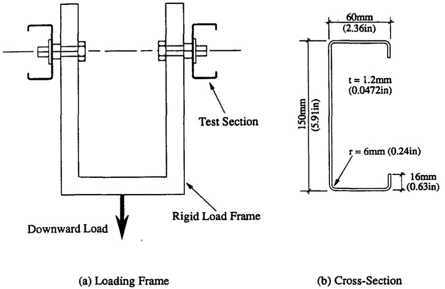
Section and Test Apparatus
