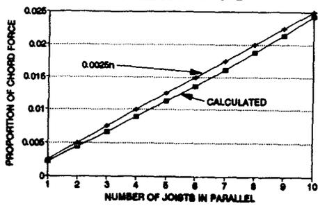
Fig.3 Variation of bracing force with number of joists
