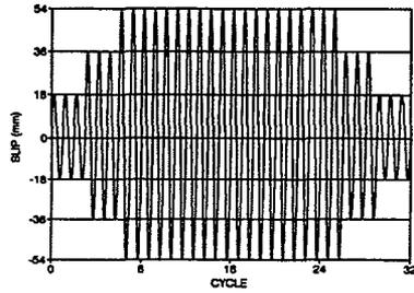
Fig. 3. Dynamic cyclic tests: a) specimen before testing, b) loading history.
