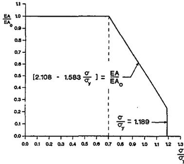
**Fig. 9** Axial Stiffness Correction
