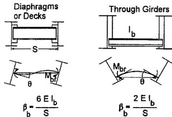
Fig. 20 Torsional Bracing Stiffness
