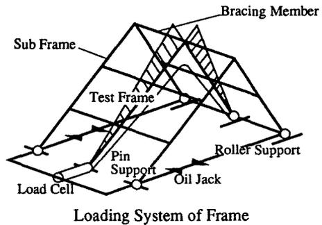
Fig.2 Bracing and Loading Condition
