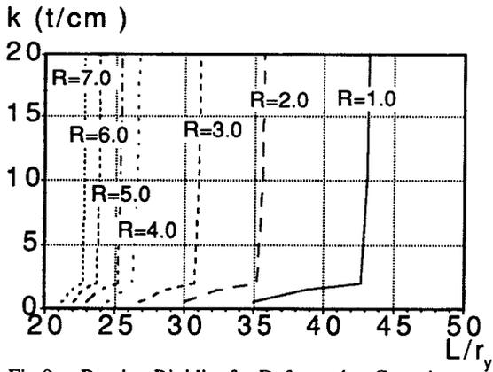
Fig.9 Bracing Rigidity for Deformation Capacity
