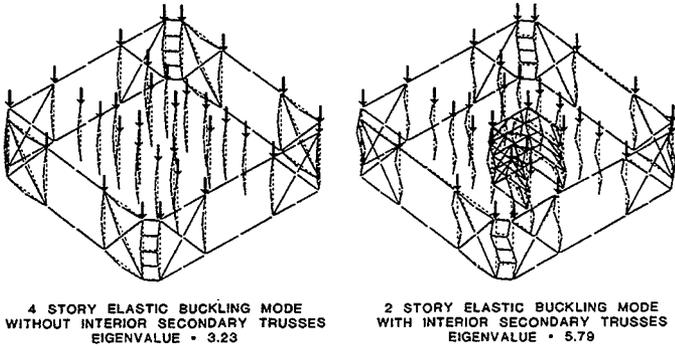
**Fig. 12 Elastic Buckling Study With/Without Secondary Trusses**
