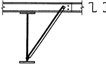
Figure 1 - Typical Cross section with Diagonal Brace
