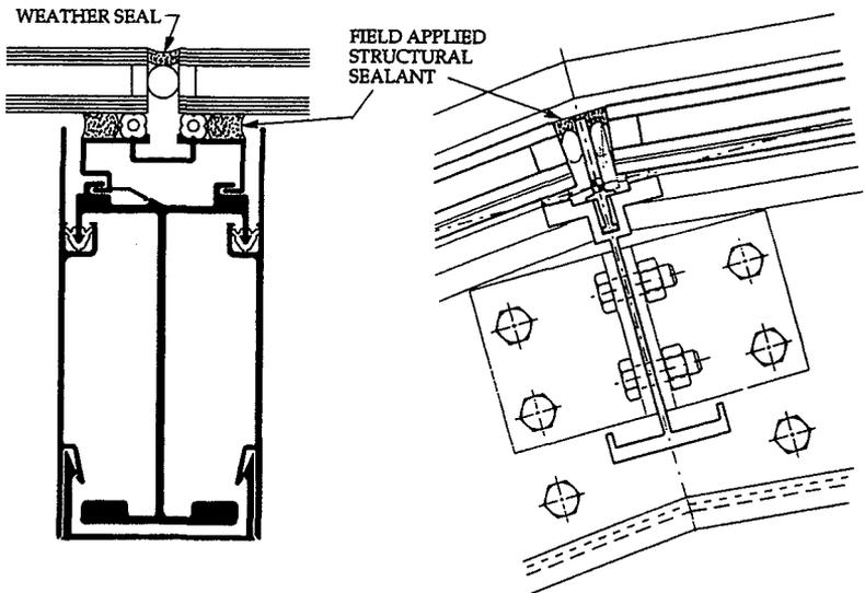
FIGURE 4 - GLASS HELD BY STRUCTURAL SEALANT
