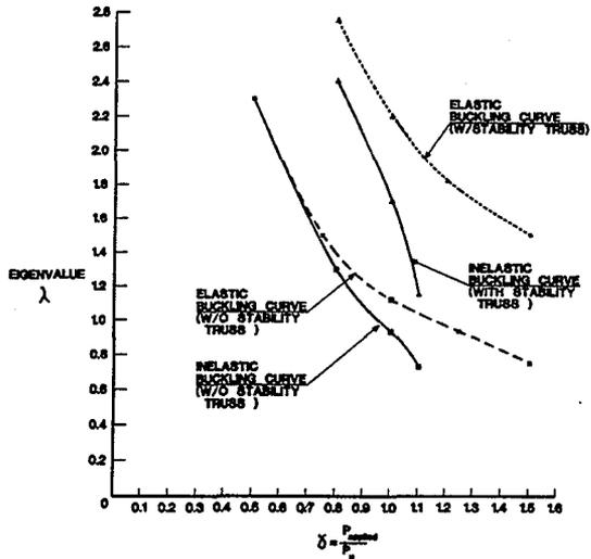
Fig. 19 Integrated Example Buckling Results
