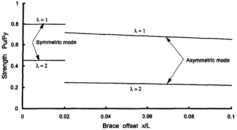
Fig. 3 Influence of brace position on column strength.
