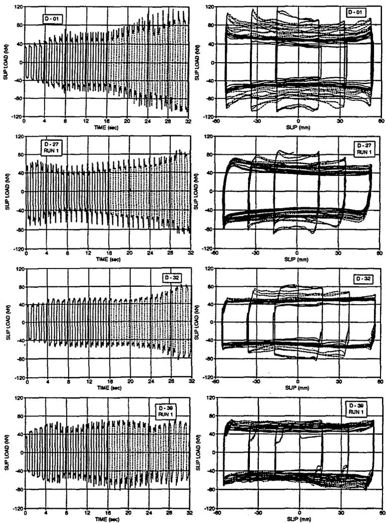
Fig. 4. Dynamic cyclic tests: slip load time history and slip load to relative slip relationships under 1.0 Hz cyclic loading.
