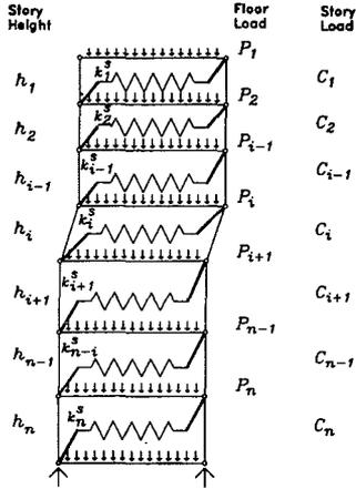
FIG. 3. Frame Model with Internal Bracing
