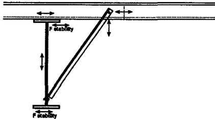
Figure 2 - Bracing Forces Induced into Secondary Members
