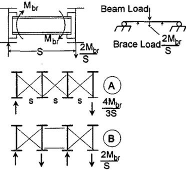
Fig. 22 Beam Load from Braces
