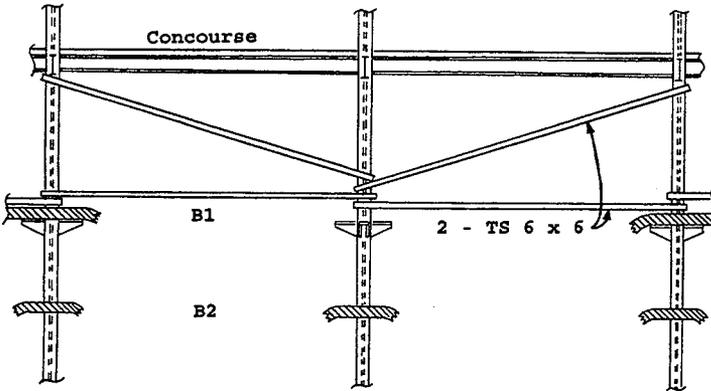
FIGURE 4: Schematic detail of emergency bracing
