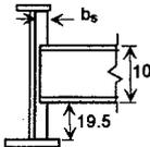
The stiffness of the diaphragms on the exterior girders is  $6EI_{br}/S$ . Since there are diaphragms on both sides of each interior girder, the stiffness is  $2 \times 6EI_{br}/S$ . The average stiffness available to each girder is  $(2 \times 6 + 3 \times 12)/5 = 9.6 EI_{br}/S$ .
