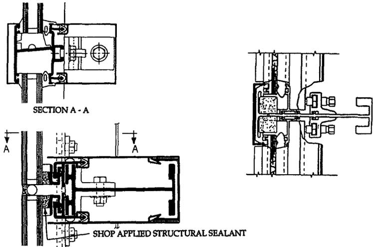
FIGURE 7 - HORIZONTAL MEMBERS WITH FLANGES RELYING ON WEB STIFFNESS
