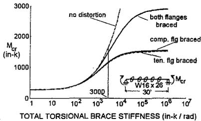
Fig. 15 Effect of Torsional Brace Location
