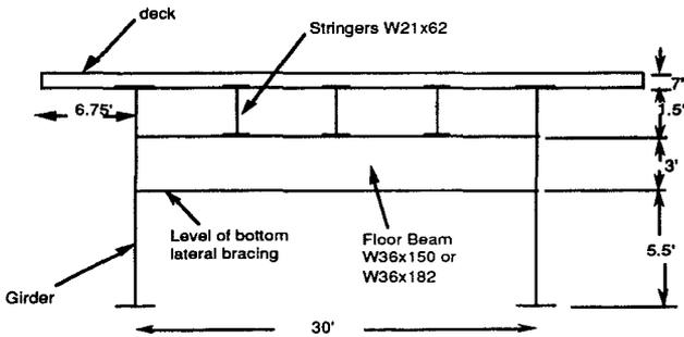
Figure 3. Bridge Cross-Section
