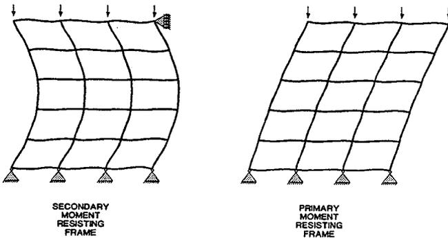
Fig. 5 Moment Resisting Frame Buckling Modes
