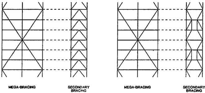
Fig. 4 Secondary Bracing System Forms (Source: Thornton, et. al. 1988)
