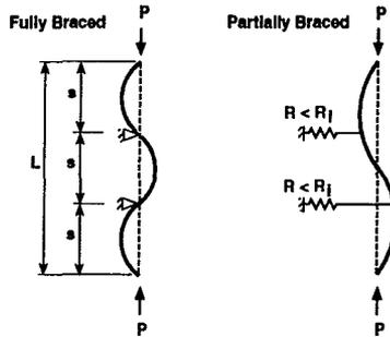
Figure 5 - Buckling modes of fully braced versus partially braced column halves
