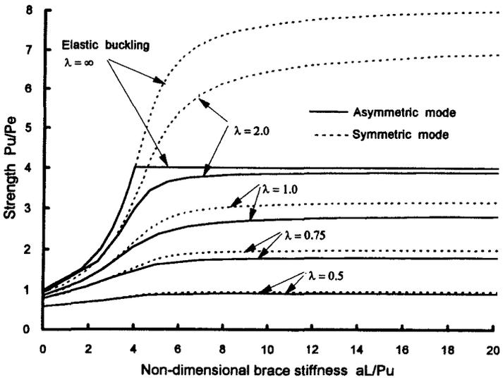
Fig.5 Ultimate strength of columns of  $\lambda = 1$  with central brace of varying stiffness  $aL/P_u$
