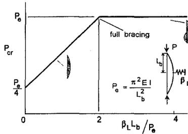
Fig. 1 Effect of Brace Stiffness
