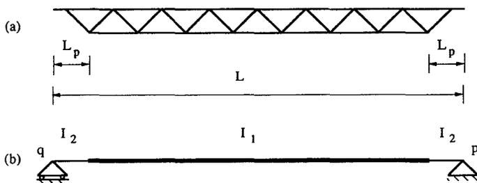
Fig. 1 (a) Open-web steel joist (b) Equivalent beam model
