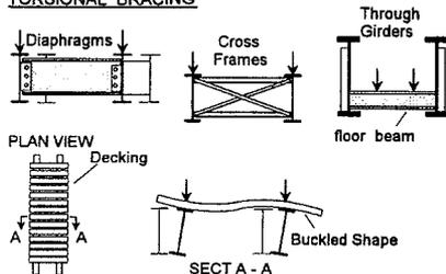
Fig. 3 Types of Beam Bracing
