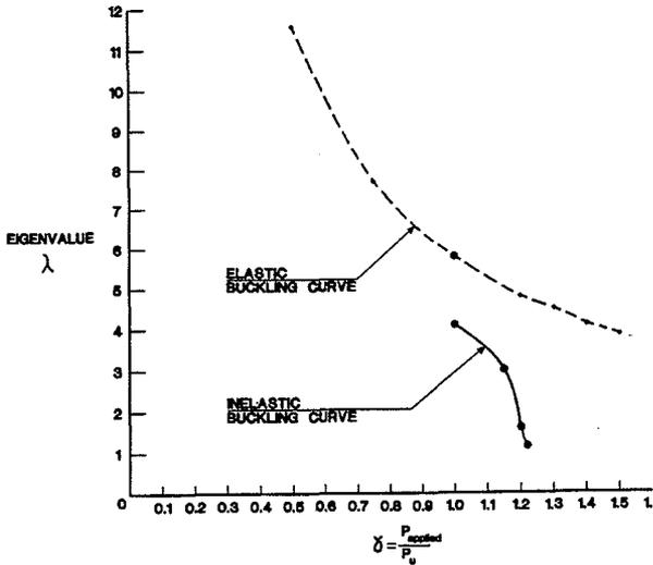
**Fig. 13 Buckling Analysis Results**
