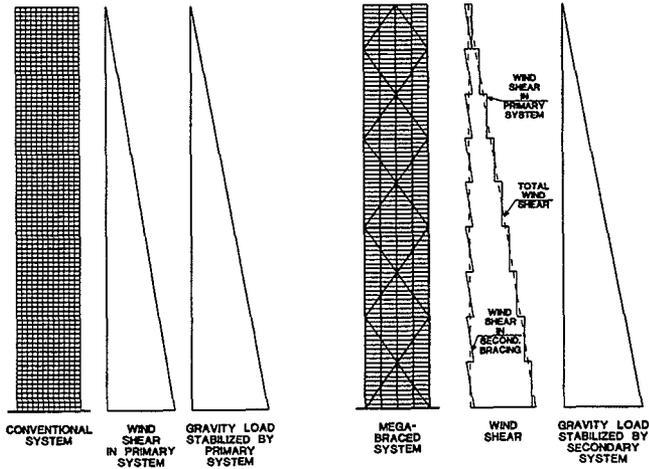
Fig. 3 Separation of Lateral Load and Stability Systems
