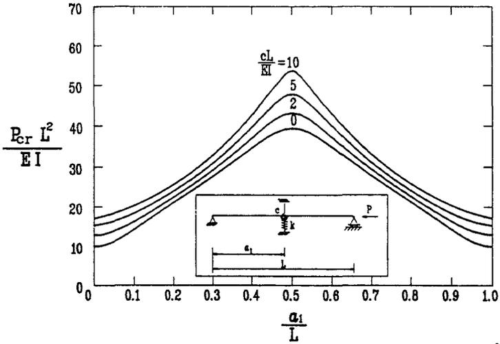
Fig. 1. Effect of bracing location on critical load;  $k=300EI/L^3$
