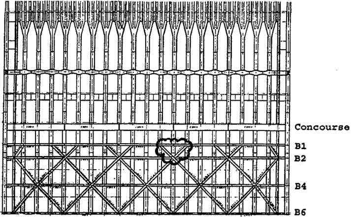
FIGURE 3: South elevation of Tower 1, indicating damaged area
