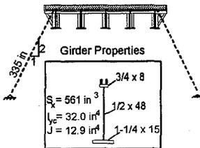
Span = 80 ft.; 10 in. concrete slab
