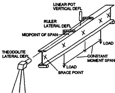
Figure 14: INSTRUMENTATION
