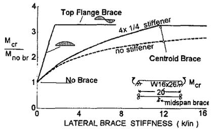
Fig. 6 Effect of Lateral Brace Location
