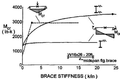
Fig. 10 Beams with Inflection Points
