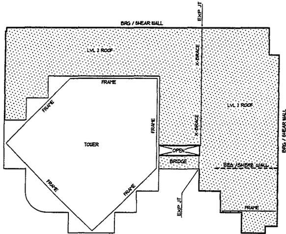
Fig. 2 FRAMING AT LEVEL 2 - 2ND FLOOR OFFICE TOWER AND CINEMA ROOF
