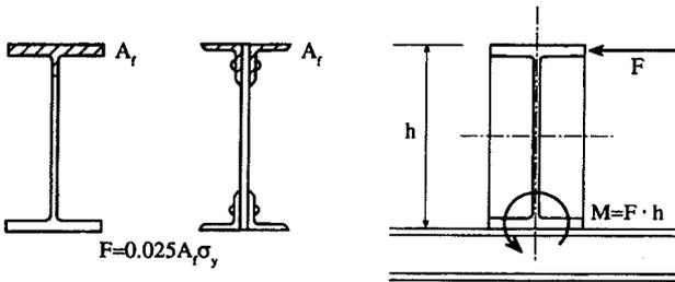
Fig.10 Bracing Force
