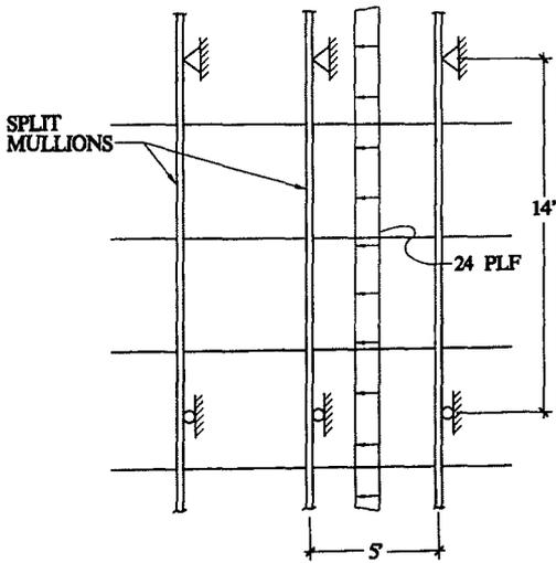
FIGURE 8 - CURTAINWALL FRAMING WITH SPLIT MULLIONS
