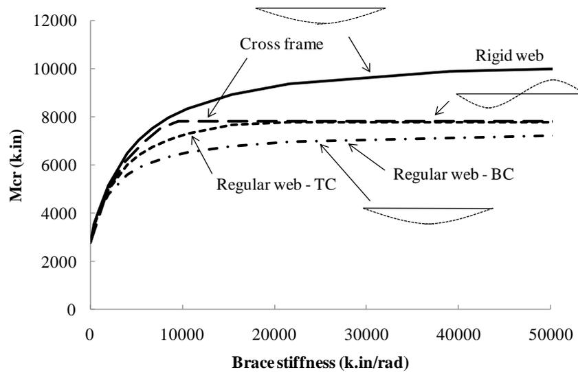
Figure 7 Buckling behavior of truss with different bracing conditions (W8x24 chord W3x8 web truss)
