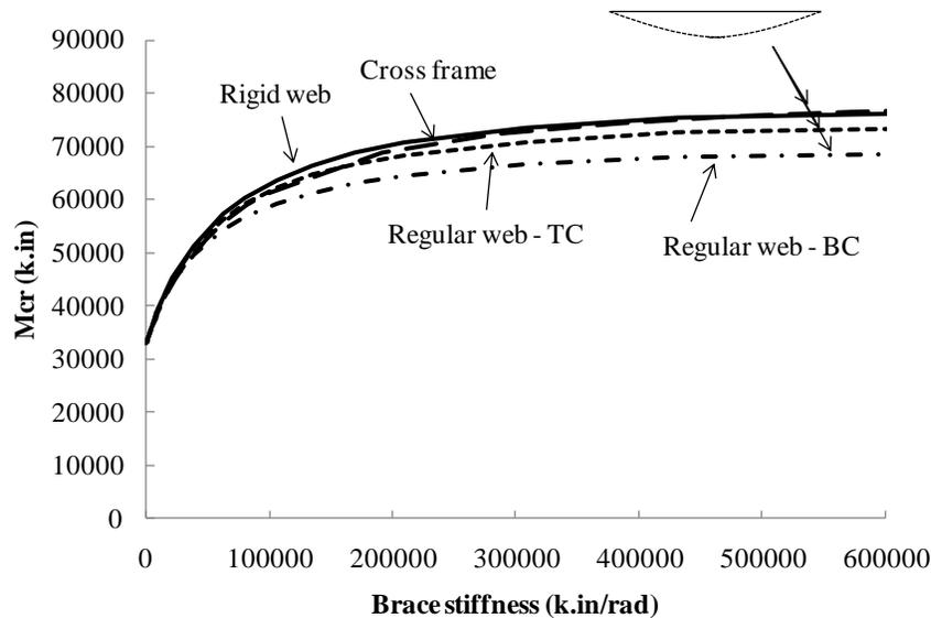
Figure 9 Buckling behavior of truss with different bracing conditions (W12x50 chord W12x26 web truss)
