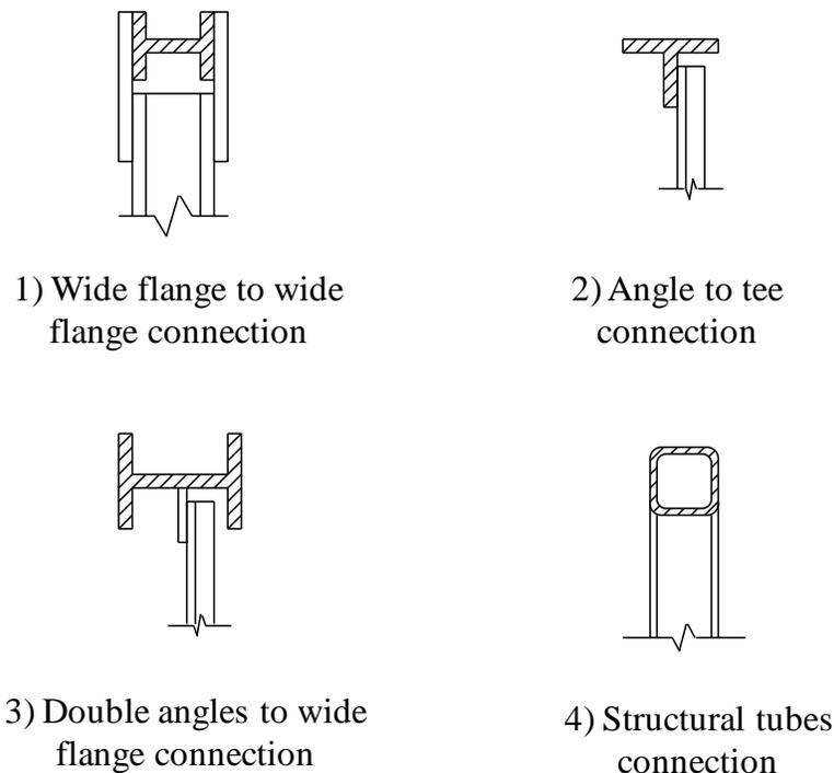
Figure 1 Types of truss connection (DeBlauw, 2007)
