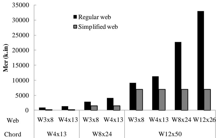
Figure 10 Buckling capacity of truss with uniform moment
