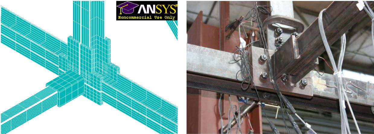
Figure 3 Comparison of the FEA model to actual truss at midspan bottom chord
