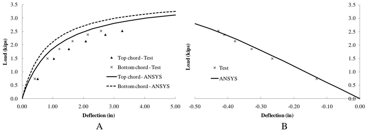
Figure 5 Buckling test of 72-ft span truss with top chord loading without intermediate bracing (A) Midspan lateral deflection (B) Midspan vertical deflection
