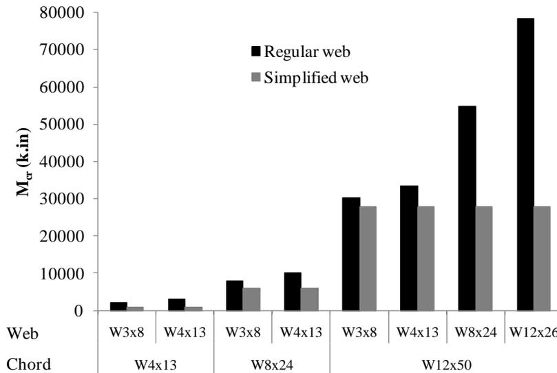
Figure 12 Buckling capacity of truss with single cross frame at midspan with uniform moment
