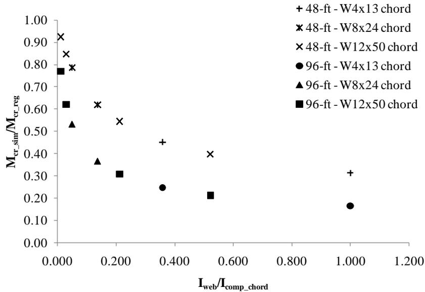
Figure 11 Reduction in buckling capacity of truss with simplified web
