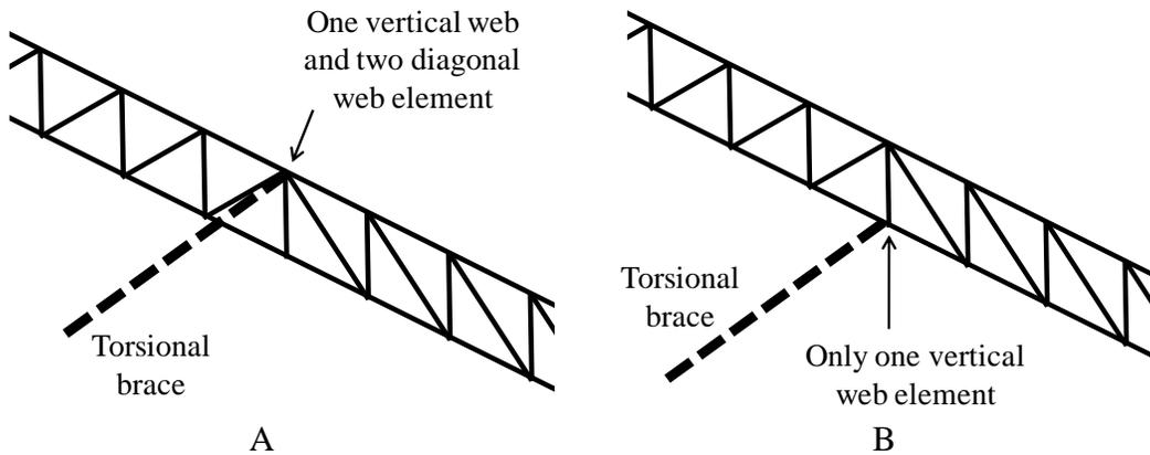
Figure 8 Midspan torsional brace connections (A) Top chord bracing (B) Bottom chord bracing
