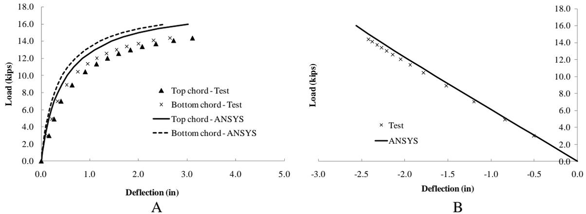
Figure 6 Buckling test of truss with 3 small torsional braces at top chord with top chord loading (A) Midspan lateral deflection (B) Midspan vertical deflection
