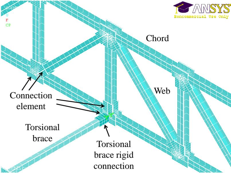
Figure 2 Enhanced FEA truss model with chord to web moment connection
