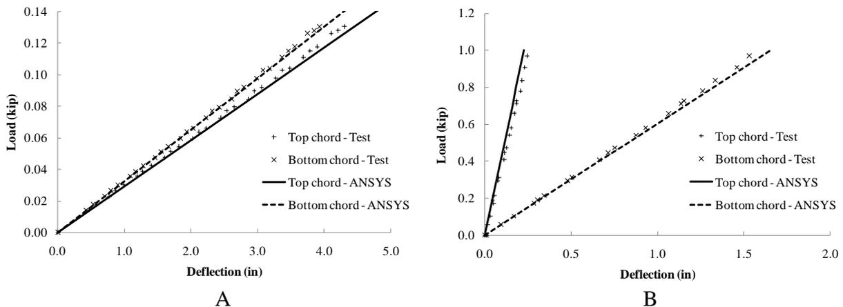
Figure 4 Midspan lateral deflections of 72-ft regular truss with bottom chord lateral loading
