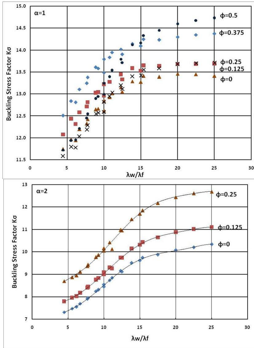
Figure 7: Variation of Shear Buckling Stress Factor with Relative Slenderness for different values of  $\alpha$  and  $\phi$
