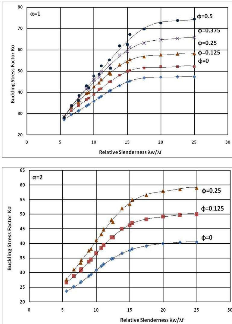
Figure 4: Variation of Bend Buckling Stress Factor with Relative Slenderness for different values of  $\alpha$  and  $\phi$
