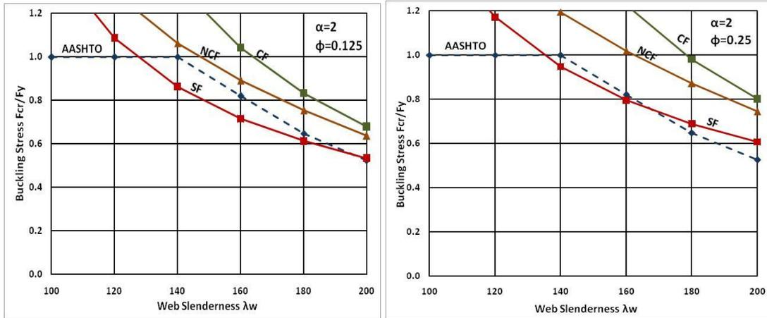
Figure 3: Variation of Bend Buckling Stress with Web Slenderness for different values of  $\alpha$  and  $\phi$  (contd.)
