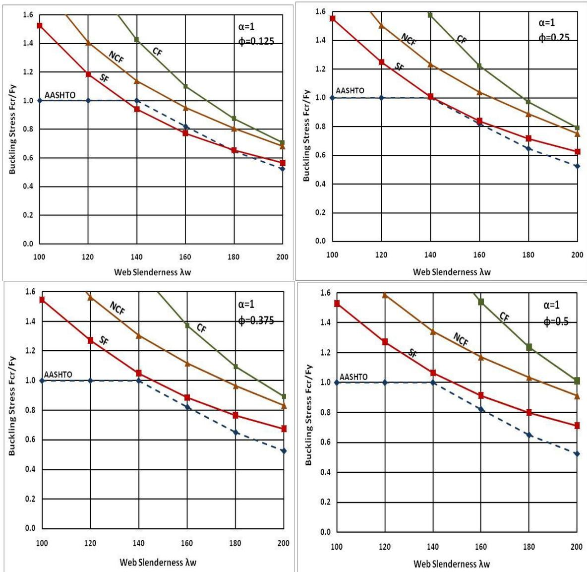
Figure 3: Variation of Bend Buckling Stress with Web Slenderness for different values of  $\alpha$  and  $\phi$
