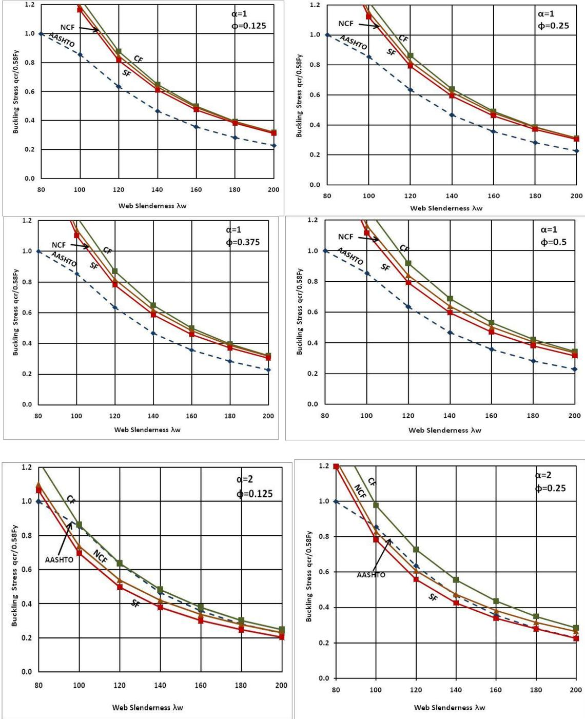
Figure 6: Variation of Shear Buckling Stress with Web Slenderness for different values of  $\alpha$  and  $\phi$
