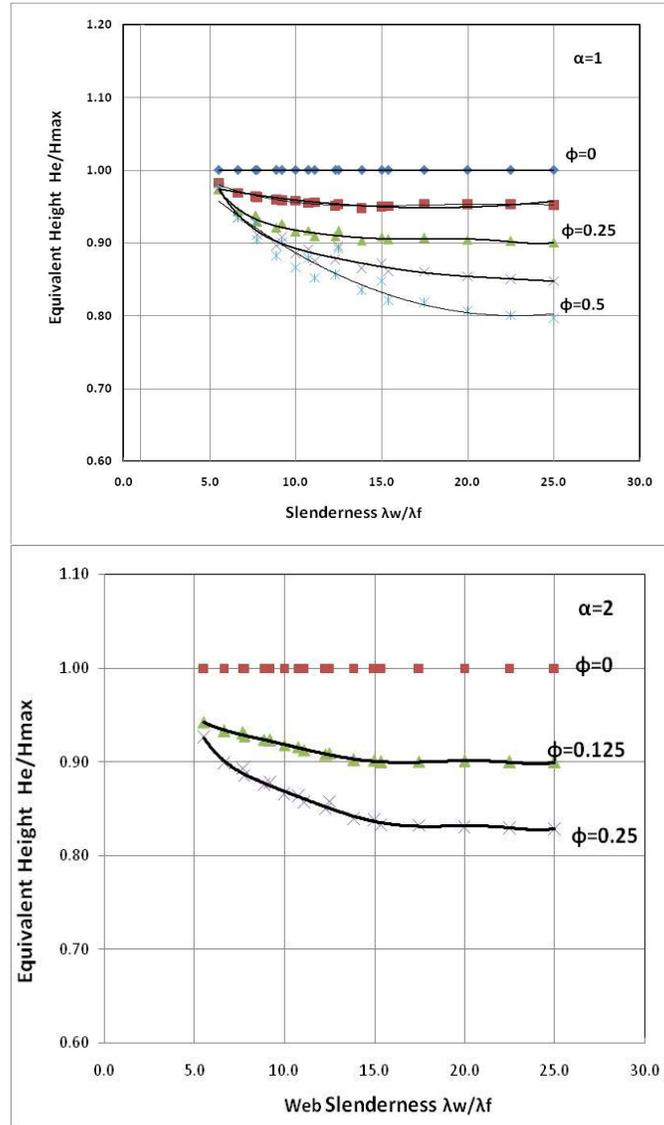
**Figure 5: Height of Equivalent Prismatic Girder**
