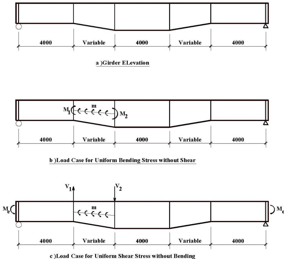
**Figure 1: Tapered Girder Model and Loading**
