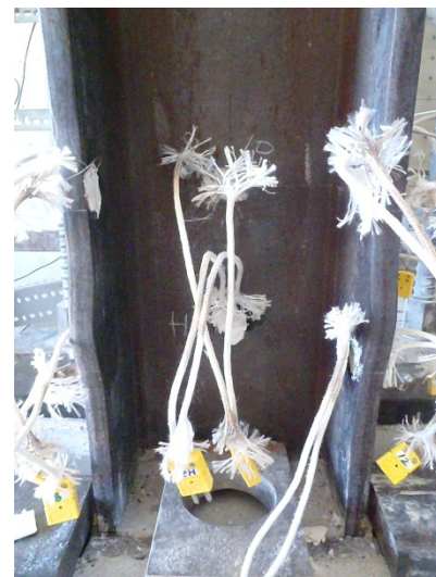
Figure 4: Local buckling at the heated region.
