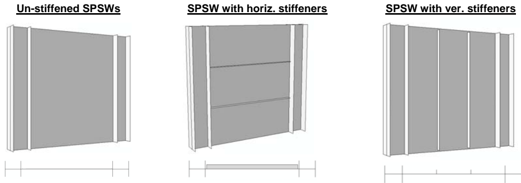
Figure 1: Un-stiffened steel plate shear wall and stiffened steel plate shear wall
