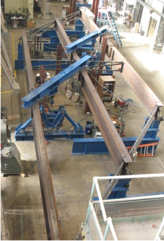
(a) Full load on continuous cross frames
