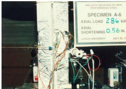
b) Test Specimen Near its Maximum Load-carrying Capacity
