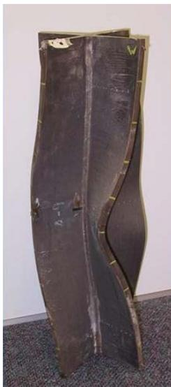
a) Inelastic Local Flange Buckling of “Fixed-Fixed” Column, West View, Specimen A-9
