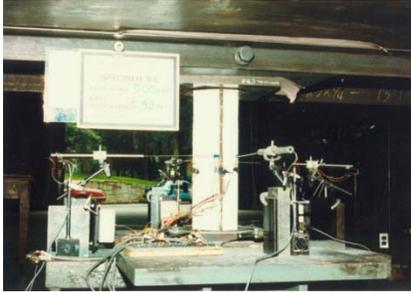
a) Test Specimen Near the Onset of Transverse Plate Movement
