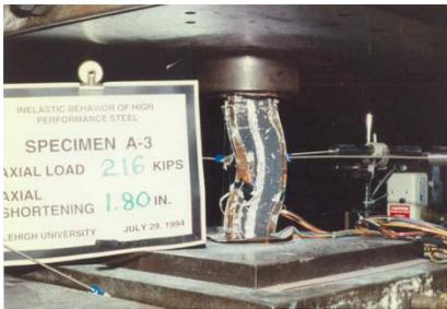
Figure 10: Specimen A-3 Deformed Shape at End of Test
