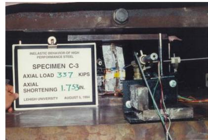
Figure 12: Specimen C-3 Deformed Shape at End of Test
